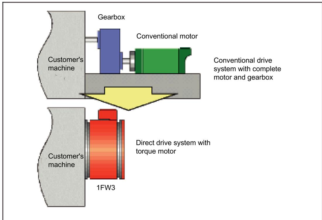
Figure 5-10 Comparison between conventional and direct drive systems
