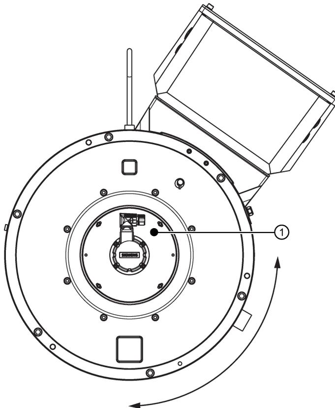
1 Center of gravity outside the motor axis
