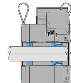
Hollow shaft with inner clamping element from the Ringspann company
