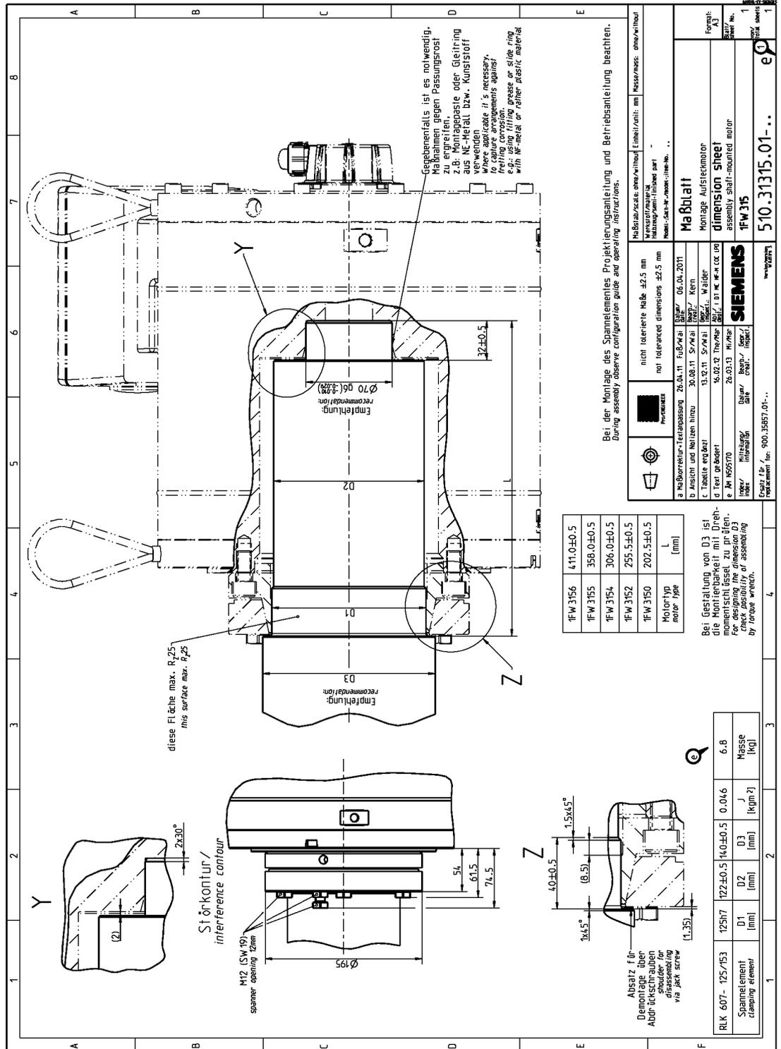
Figure 5-24 Dimension drawing, mounting plug-on motor 1FW315
