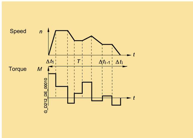
Figure 5-6 Example of a load duty cycle
