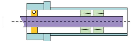
Two clamping sets are required to transmit the torque
