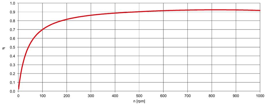
Figure 5-39 Example diagram: Efficiency as a function of speed
