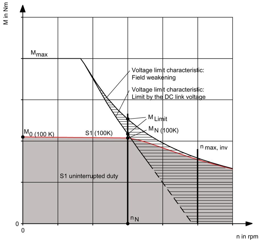
Figure 6-1 Torque characteristic of a synchronous motor operating on a SINAMICS drive system with field weakening (example characteristic)
