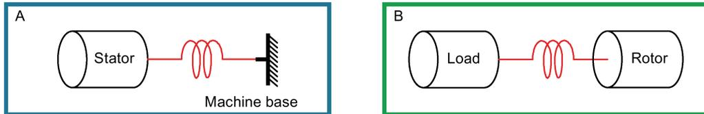
The influence of the Siemens torque arm is shown qualitatively in the following diagram. The two-mass oscillating system comprising motor and load still dominates the system response; however, coupling the stator through the Siemens torque arm is manifested in the form of additional resonance effects, which must be damped by the closed-loop control.
