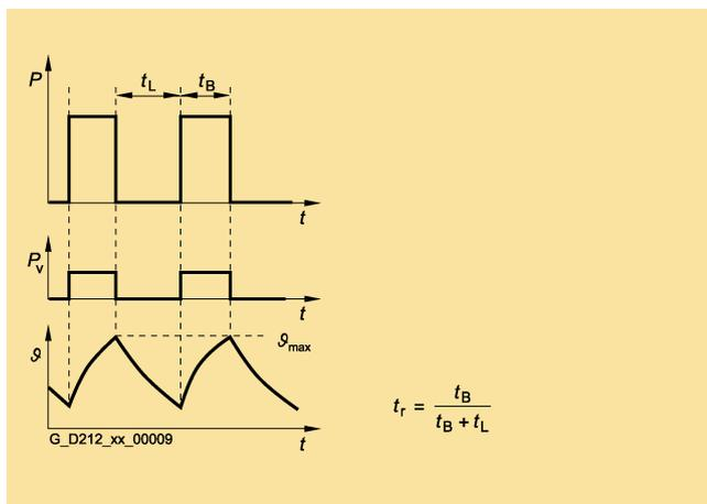
Figure 5-4 S3 duty (intermittent operation without influencing starting)
