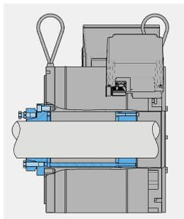
Hollow shaft with option, clamping element and centering part
