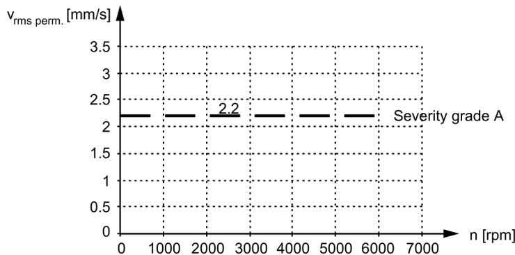
Figure 3-30 Vibration severity grade
