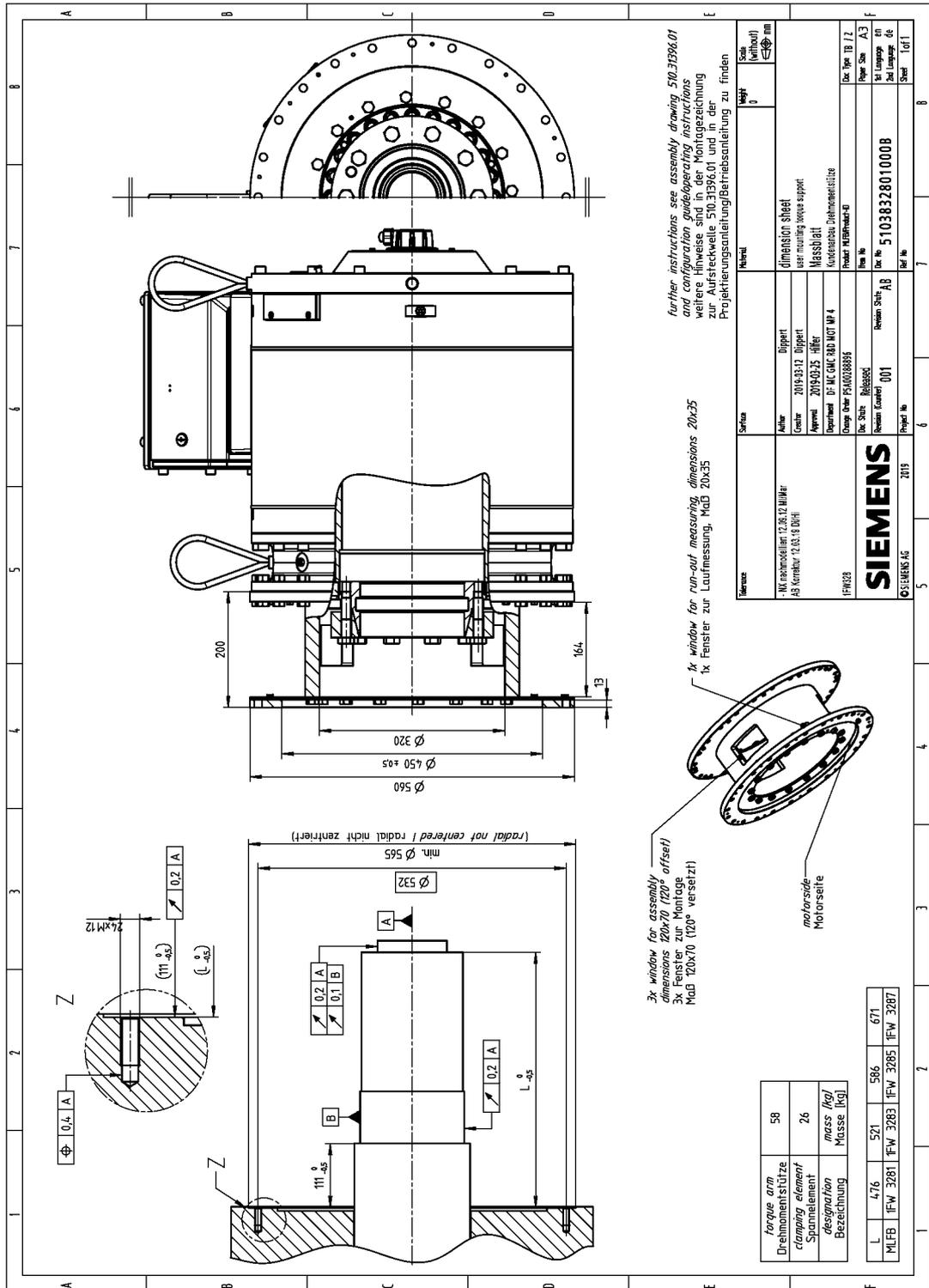
Figure 5-22 1FW328 Siemens torque arm, dimension drawing 510.38328.01
