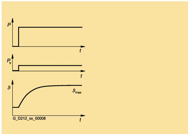
Figure 5-3 S1 duty (continuous operation)
