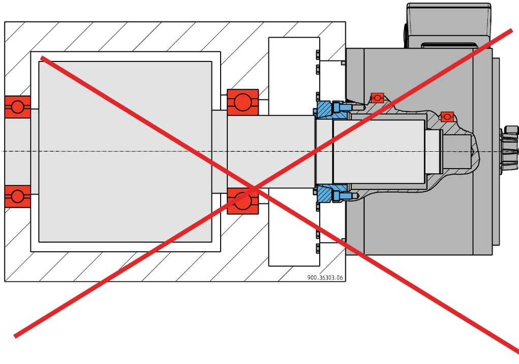
Figure 5-11 Overdetermined bearing of a shaft
