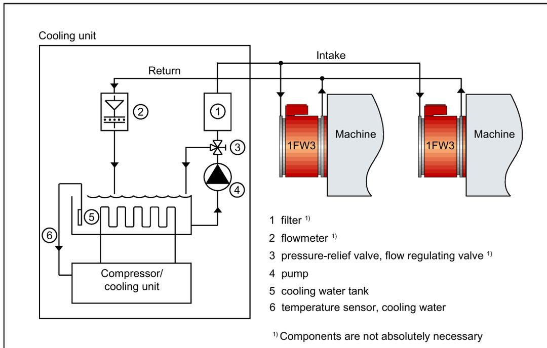
Figure 3-1 Example of a semi-open cooling circuit
