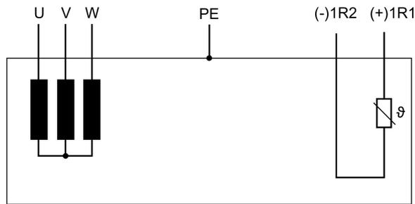
Figure 8-1 Circuit diagram of a motor
