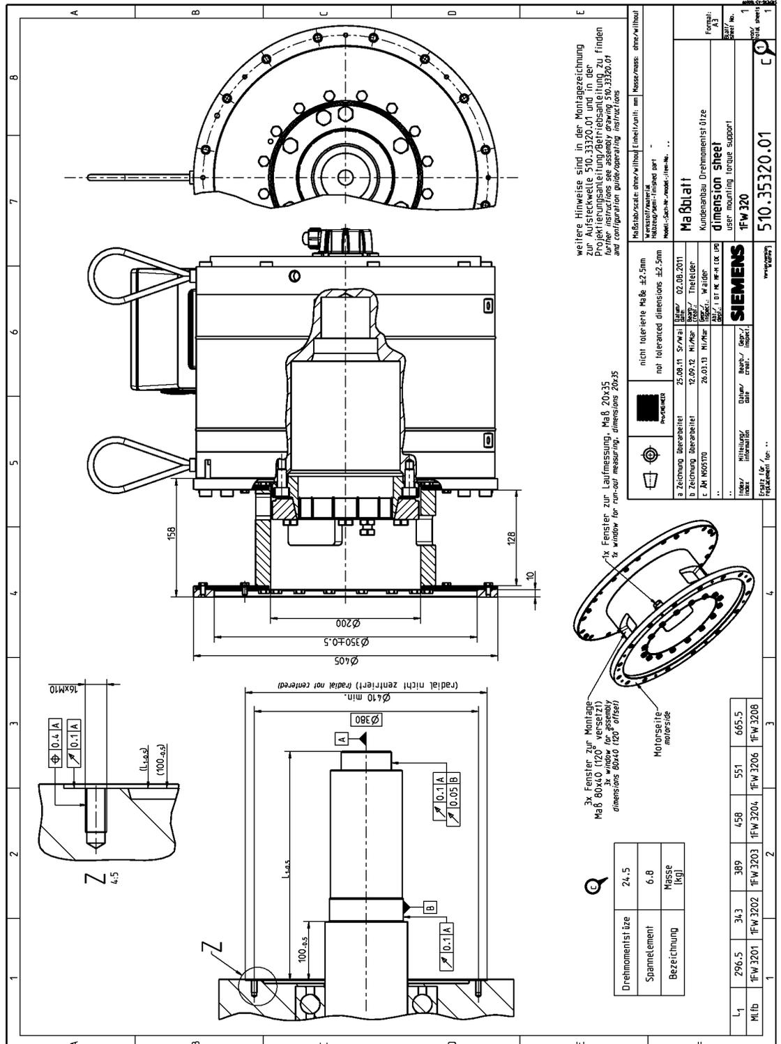
Figure 5-21 1FW320 Siemens torque arm, dimension drawing 510.35320.01
