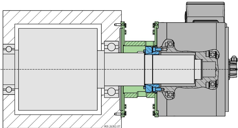
Figure 5-13 Schematic representation of the Siemens torque arm
