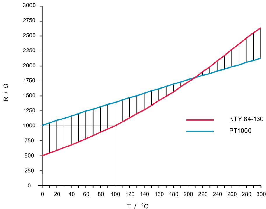
Figure 4-3 Comparison of KTY 84-130 and Pt1000 temperature sensors
