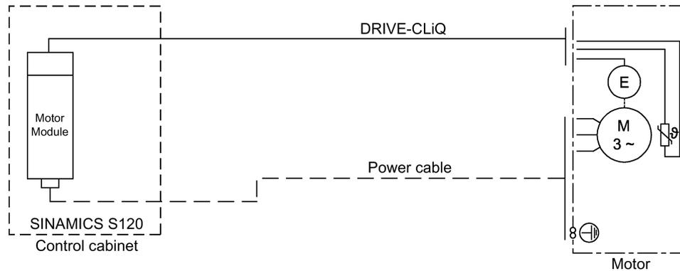
Figure 8-7 Connecting encoders using the DRIVE-CLiQ interface
