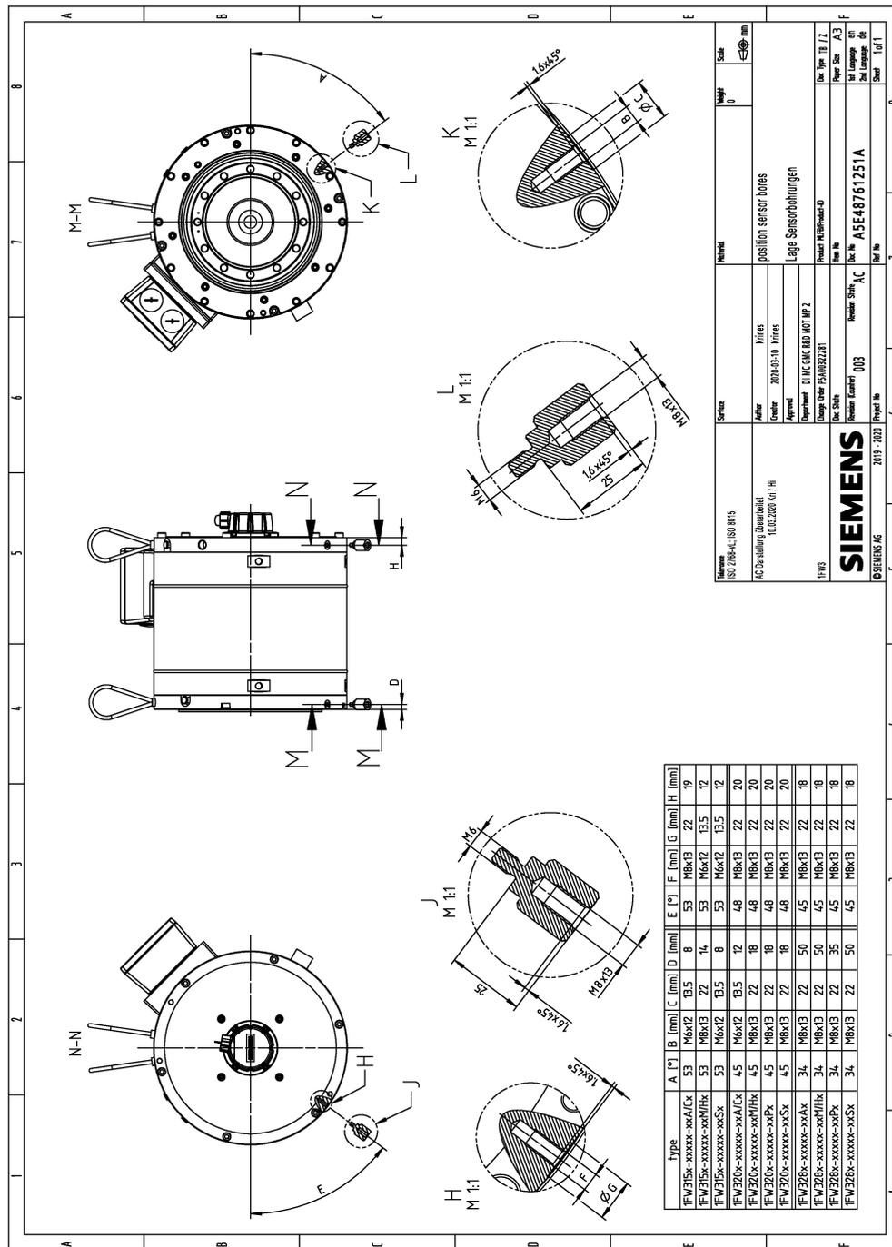
Figure 5-36 Position and dimensions of the sensor holes for the vibration sensors
