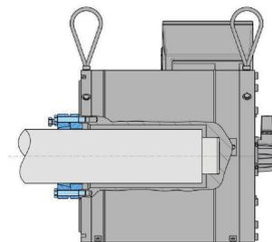
Plug-on shaft with clamping element
