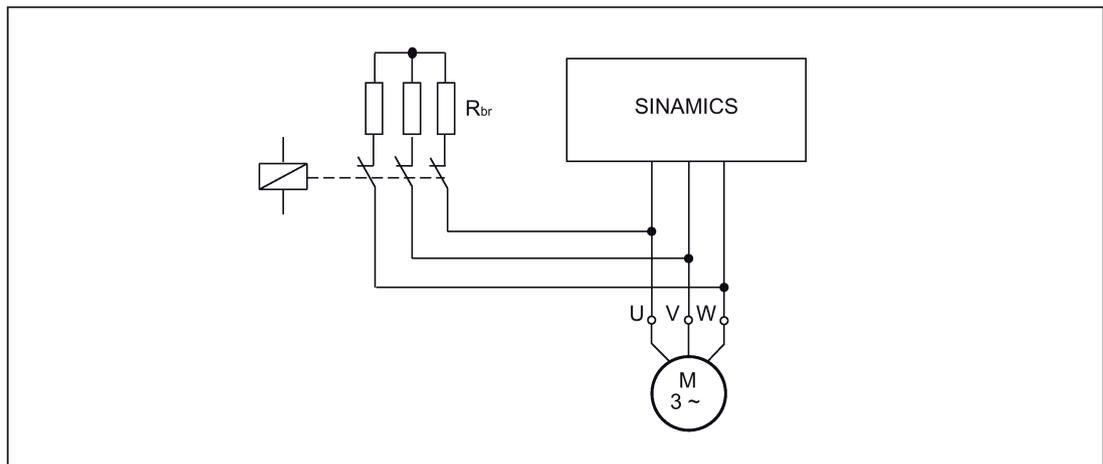
Figure 5-8 Circuit (schematic) with brake resistors
