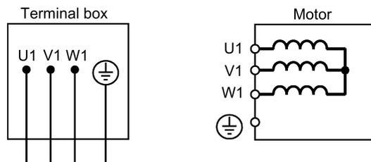
Y circuit: supply voltage 400 V / 480 V
