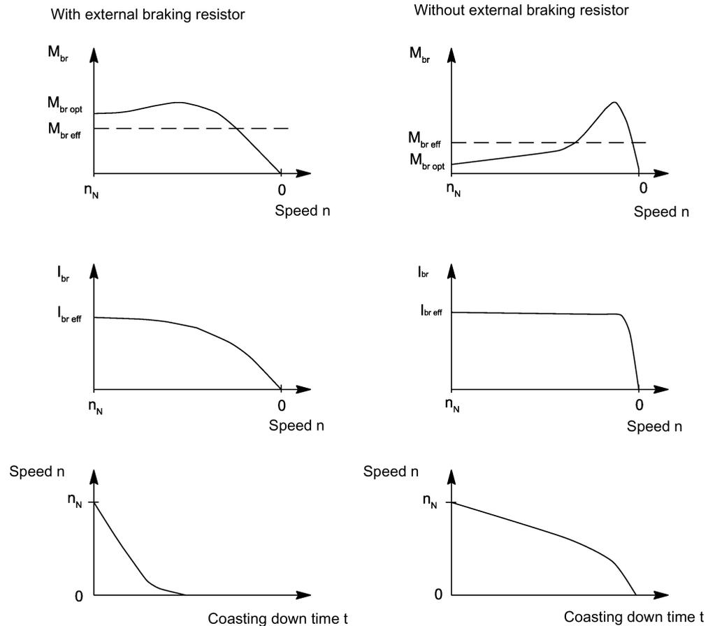
Figure 5-9 Armature short-circuit braking
