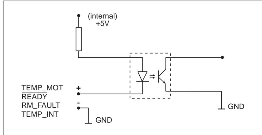
Fig. 2-7 Input circuit principle
