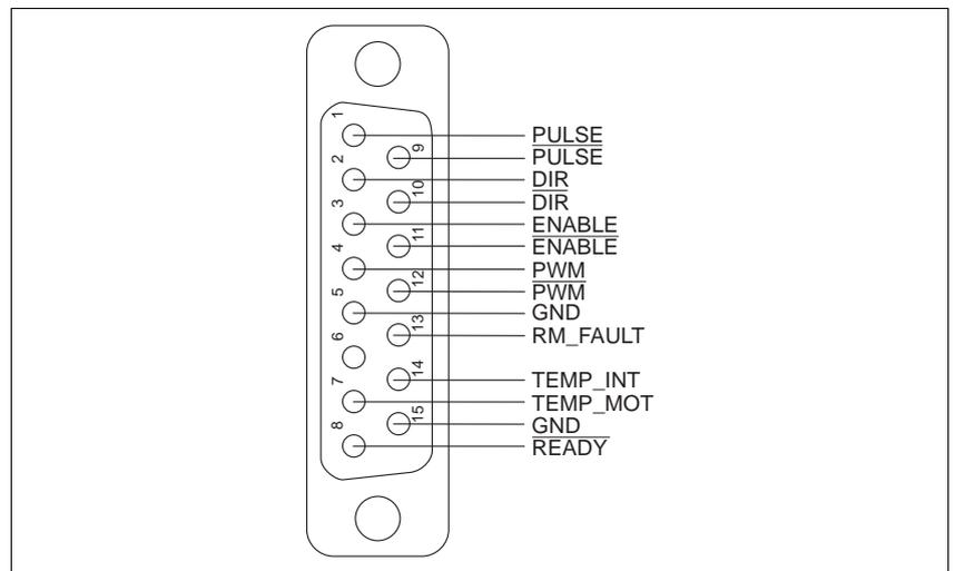
Fig. 2-3 Power controller connector assembly
