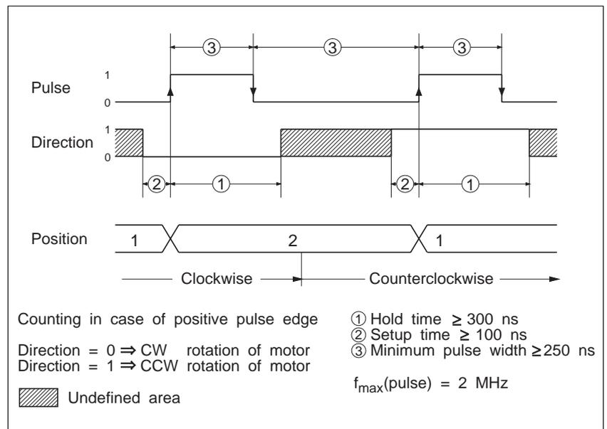
Fig. 2-23 Timing diagram – pulse/direction signals
