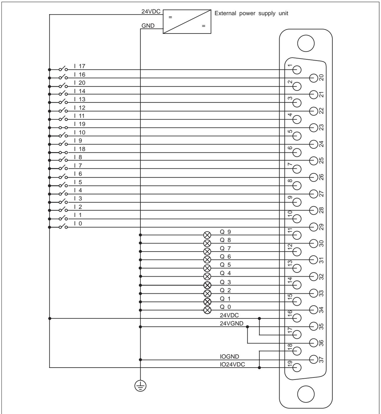
Fig. 2-11 Wiring example
