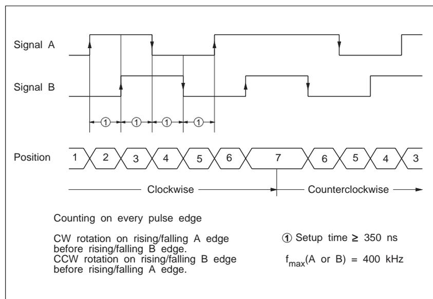
Fig. 2-22 Timing diagram – encoder signals A/B
