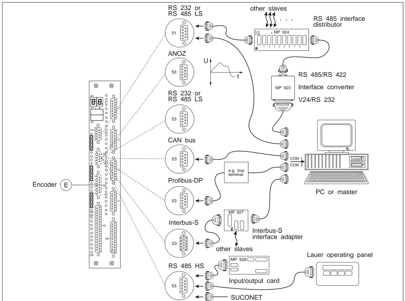
Fig. 1-5 Connection diagram
