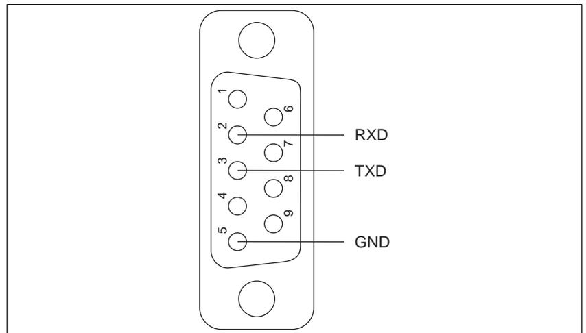
*Fig. 2-13 Controller/PC wiring*
