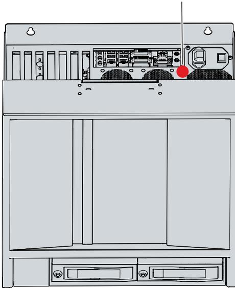
Fig. 16: C6675\_Grounding bolt for functional earthing
