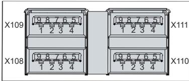
Fig. 5: C6675\_USB interface pin numbering
