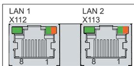
Fig. 6: C6675\_Ethernet interface pin numbering
