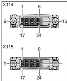
Fig. 7: C6675\_DVI interface pin numbering
