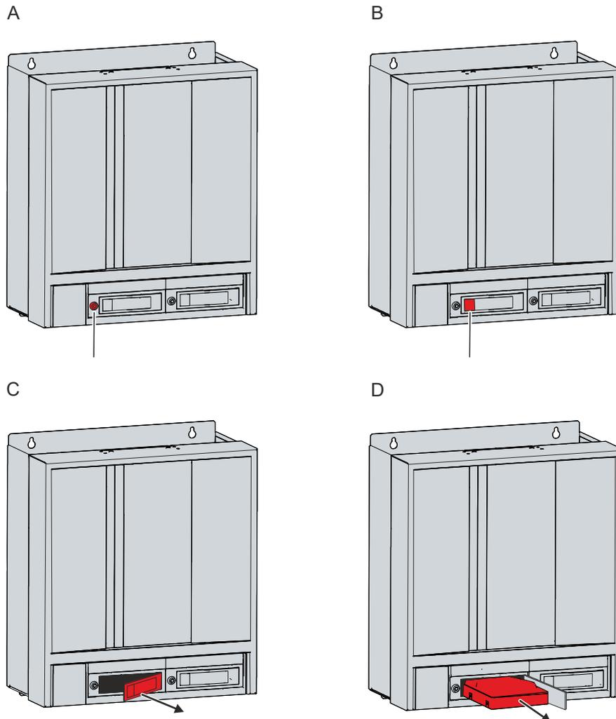
Fig. 25: C6675\_exchange hard disk
