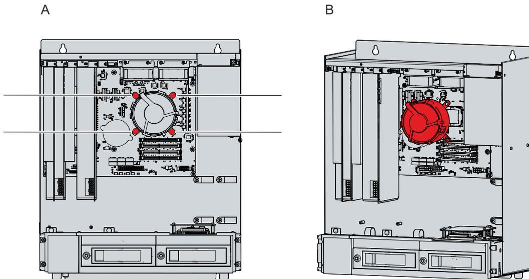
Fig. 29: C6675\_exchange CPU cooler
