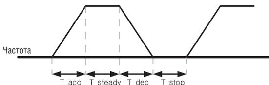
$$H76 = \frac{T\_dec}{T\_dec + T\_steady1 + T\_acc + T\_steady2} \times 100 [\%]$$
