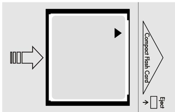
Figure 4-25 Inserting the memory card
