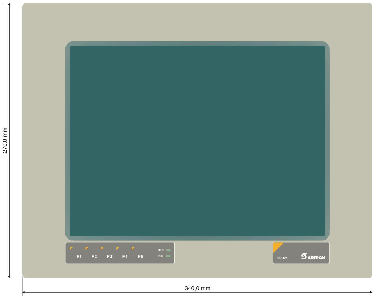
Figure 2-1 Front Panel Dimensions
