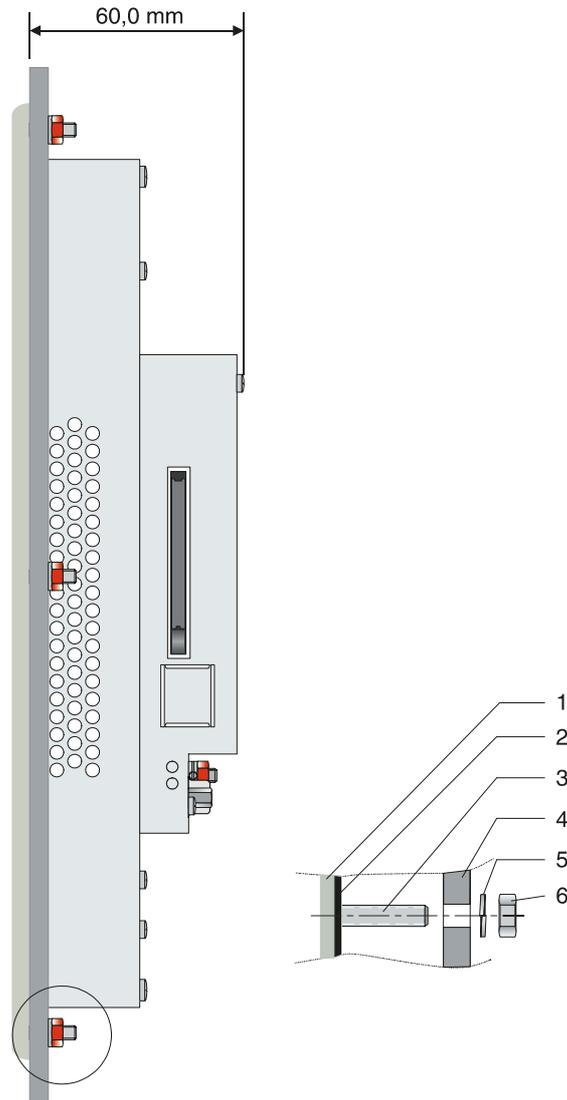
Figure 2-3 Side view and mounting depth for standard device
