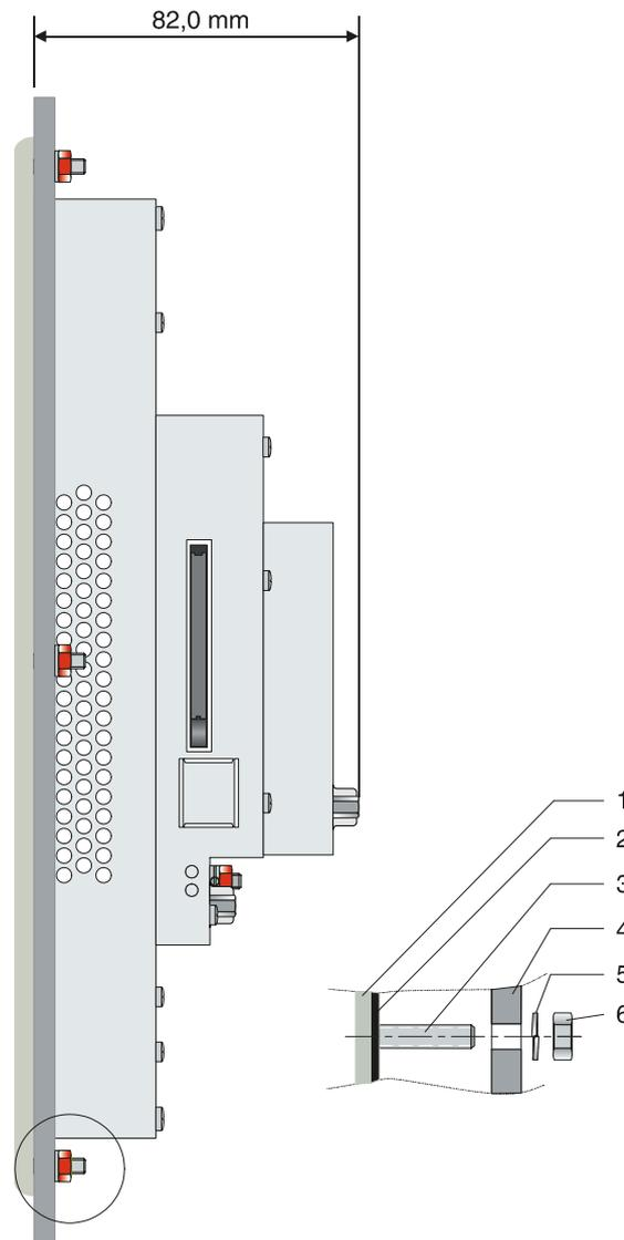
Figure 2-4 Side view and mounting depth for field bus device
