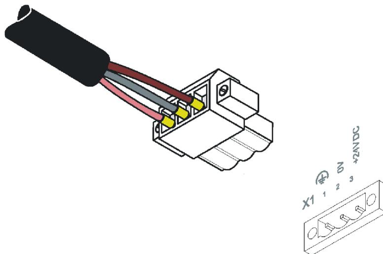
Figure 2-7 Female connector strip is plugged on
