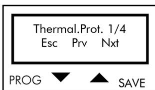
Press PROG to quit the Motor Thermal Protection submenu. Press ↓ and ↑ to scroll through the parameters.
