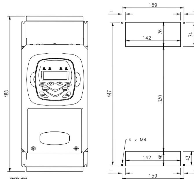
Figure 2: Piercing template of the mounting panel for SINUS K S05 through-panel assembly.
