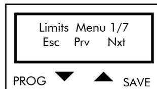
Press PROG to quit the Limits submenu. Press ↓ and ↑ to scroll through the parameters.
