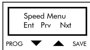
Press PROG to access the submenu. The first page of the submenu appears:
