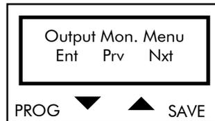
Press PROG to enter the Output Monitor submenu. Press ↑ and ↓ to scroll through the other submenus.
