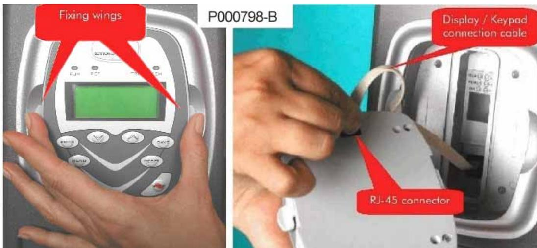
Figure 17: Removing the display/keypad.
