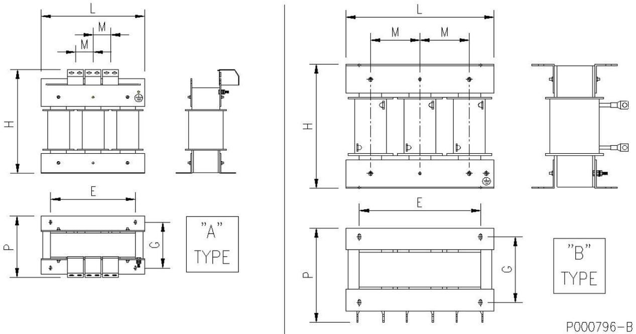
Figure 22: Mechanical features of an AC 3-phase inductance.
