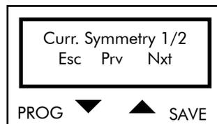
Press PROG to quit the Carrier Symmetry submenu; press  $\downarrow$  and  $\uparrow$  to scroll through the parameters.
