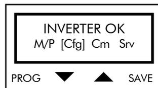
Press  $\uparrow$  and  $\downarrow$  to select a different submenu (in square brackets), then press PROG to access the selected submenu.
