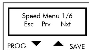
Press PROG to quit the Speed submenu. Press ↑ and ↓ to scroll through the parameters.
