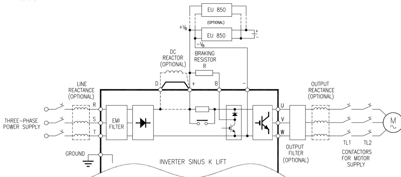
Figure 33: Wiring diagram for EU850 unit.
