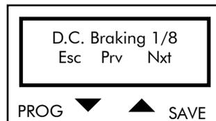
Press PROG to quit the D.C. Braking submenu. Press ↓ and ↑ to scroll through the parameters.
