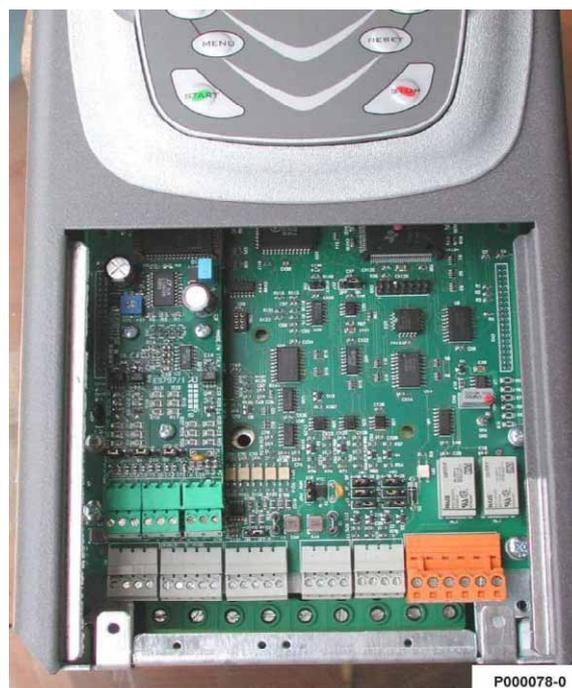
Figure 25: Encoder board fastened to its slot.
