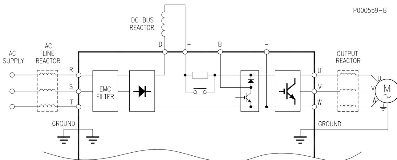
Figure 19: Wiring diagram for optional inductance.
