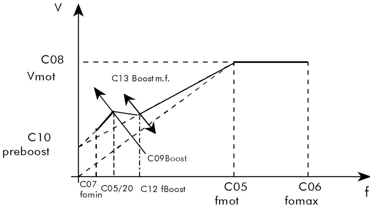
**Figure 35: Parameters relating to voltage/frequency pattern.**
