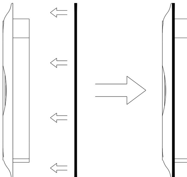
3 – Fit the plastic shell in the relevant slot.
