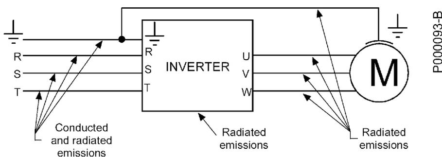
Figure 53: Disturbance sources in a power drive system equipped with an inverter.
