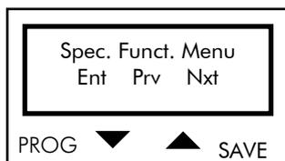
Press PROG to enter the Special Function submenu. Press ↓ and ↑ to scroll through the other submenus of the Configuration menu.
