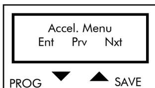
Press PROG to enter the Acceleration submenu. Press ↑ and ↓ to scroll through the other submenus.
