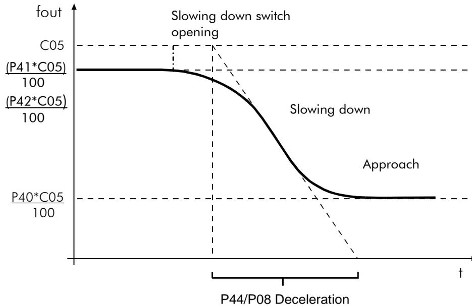
Figure 45: Frequency produced during slowing down in Normal operating mode.
