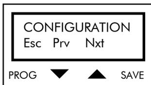
Press PROG to return to the page for the selection of the main menus; press ↑ and ↓ to scroll through the submenus.
