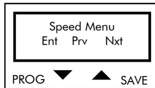
Press PROG to enter the Speed submenu. Press ↑ and ↓ to scroll through the other submenus.
