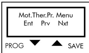
Press PROG to enter the Motor Thermal Protection submenu. Press ↓ and ↑ to scroll through the other submenus of the Configuration menu.
