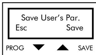
Press PROG to quit the Save User's Parameters submenu; press SAVE to save all the parameters. The square brackets indicate that parameters are being saved to Eeprom; when square brackets disappear (after a few seconds), parameter saving is over.
