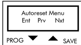
Press PROG to enter the Autoreset submenu. Press ↓ and ↑ to scroll through the other submenus of the Configuration menu.
