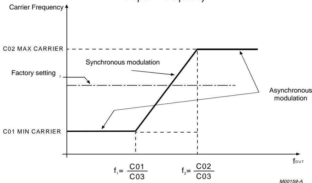
Figure 36: Carrier frequency depending on output frequency.
