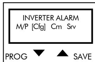
The display LEDs start flashing; alarm messages detailed in section ALARM MESSAGES may be displayed.
