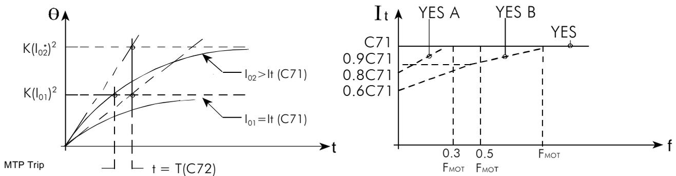
**Figure 41: Motor heating with two different, constant current values and pick-up current  $I_t$  of the motor thermal protection with respect to the frequency/speed depending on the configuration of parameter C70.**
