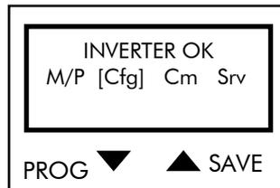
This occurs if the inverter is disabled or no run command is sent or the frequency reference is equal to zero.
