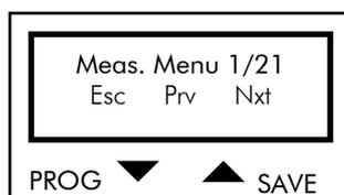
Press PROG to return to the Measures submenu access page. Press ↑ and ↓ to scroll through the parameters.
