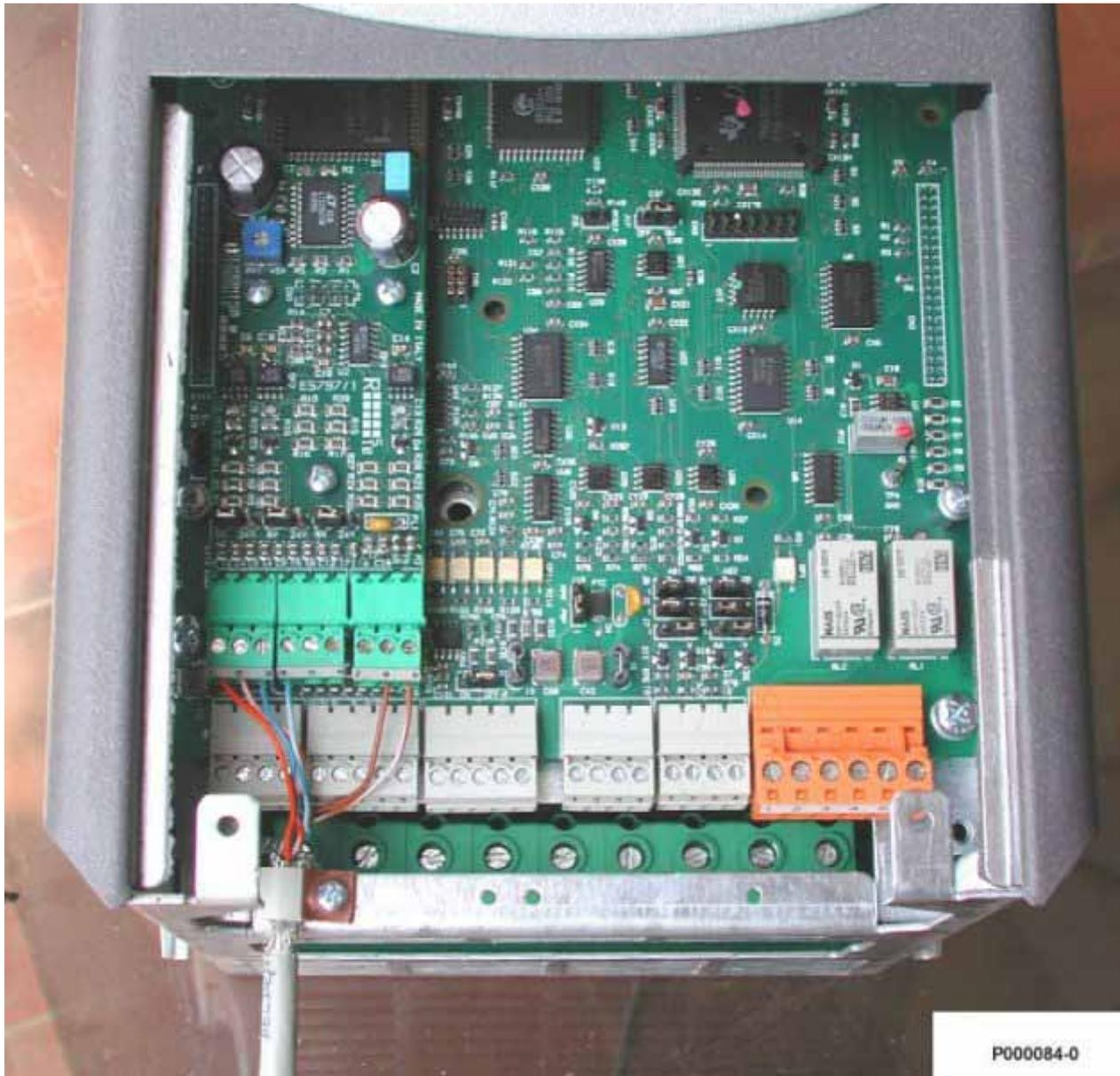
**Figure 31: Wiring the encoder cable.**
