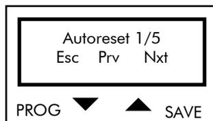
Press PROG to quit the Autoreset submenu. Press ↓ and ↑ to scroll through the parameters.
