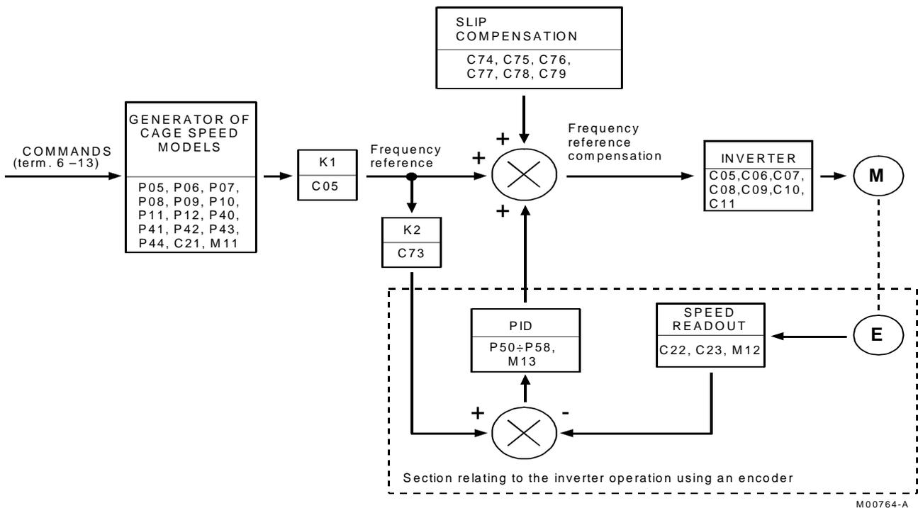
Figure 34: Block diagram of the speed regulator.
