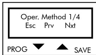
Press PROG to quit the Operation Method submenu. Press ↓ and ↑ to scroll through the parameters.
