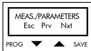
use  $\uparrow$  (Nxt) and  $\downarrow$  (Prv) to scroll the submenus up to the access page of the "Speed" submenu:
