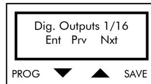
Press PROG to quit the Digital Outputs submenu. Press ↑ and ↓ to scroll through the parameters.
