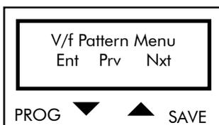
Press PROG to enter the V/F Pattern submenu. Press ↓ and ↑ to scroll through the other submenus of the Configuration menu.
