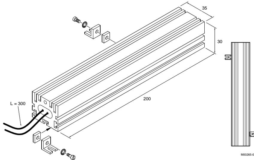
Figure 13: Overall dimensions, 56-100Ω/350W resistor.
