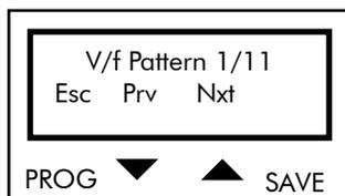
Press PROG to quit the V/F Pattern submenu. Press ↓ and ↑ to scroll through the parameters.
