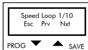
Press PROG to quit the Speed Loop submenu. Press  $\uparrow$  and  $\downarrow$  to scroll through the parameters.
