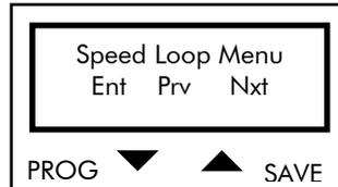
Press PROG to enter the Speed Loop submenu. Press  $\uparrow$  and  $\downarrow$  to scroll through the other submenus.
