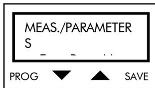
Press PROG to return to the main menu selection page; press ↑ and ↓ to scroll the submenus. All parameters are included in different submenus, except for key parameter P01 and the parameters relating to the inverter ratings. Scroll the submenus to directly access these parameters.
