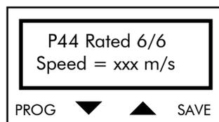
**Press PROG; the flashing cursor appears and allows altering the parameter value.**
