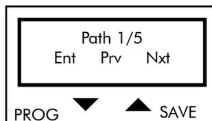
Press PROG to return to the Path submenu access page. Press ↑ and ↓ to scroll through the parameters.
