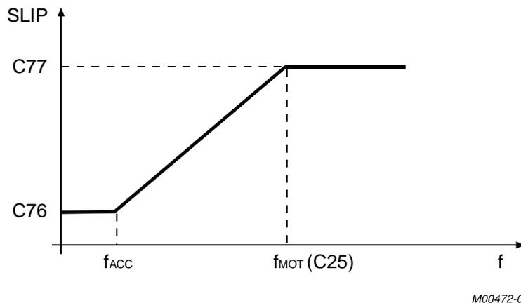
**Figure 38: Slip compensation based on the produced frequency.**
