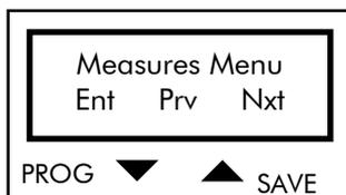
Press PROG to access the first page of the Measures submenu. Press ↑ and ↓ to scroll through the submenus.
