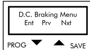
Press PROG to enter the D.C. Braking submenu. Press ↓ and ↑ to scroll through the other submenus of the Configuration menu.
