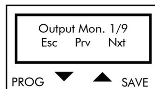
Press PROG to quit the Output Monitor submenu. Press ↑ and ↓ to scroll through the parameters.
