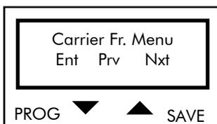
Press PROG to enter the Carrier Frequency submenu. Press ↑ and ↓ to scroll through the other submenus.
