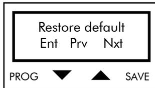
Press PROG to access the submenu: press ↑ and ↓ to scroll through the other submenus of the Commands menu.
