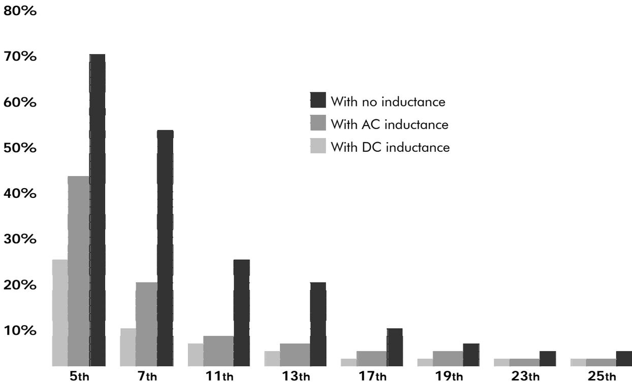
**Figure 20: Amplitude of harmonic currents (approximate values)**
