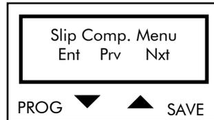
Press PROG to enter the Slip Compensation submenu. Press ↓ and ↑ to scroll through the submenus of the Configuration menu.
