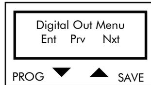
Press PROG to enter the Digital Outputs submenu. Press ↑ and ↓ to scroll through the other submenus.
