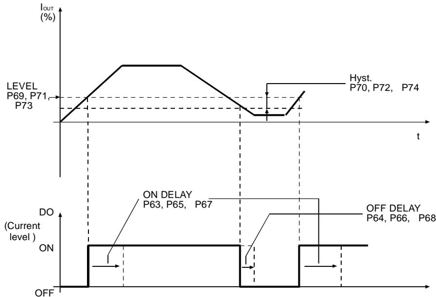
**Figure 50: Characteristics of a digital output programmed as "Current Level" and characteristics of the output frequency in respect to time.**
