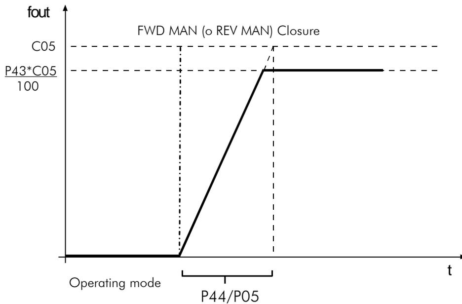
Figure 42: Frequency produced during startup in maintenance mode.
