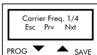
Press PROG to quit the Carrier Frequency submenu; press ↓ and ↑ to scroll through the parameters.
