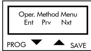
Press PROG to enter the Operation Method submenu. Press ↓ and ↑ to scroll through the other submenus of the Configuration menu.
