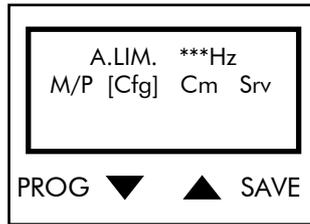
7) If the output frequency is under the reference value for current limit activation at constant frequency:
