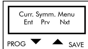
Press PROG to enter the Carrier Symmetry submenu. Press  $\uparrow$  and  $\downarrow$  to scroll through the other submenus.
