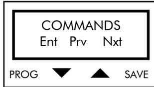
Press PROG to return to the page for the selection of the main menus; press ↑ and ↓ to scroll through the submenus.
