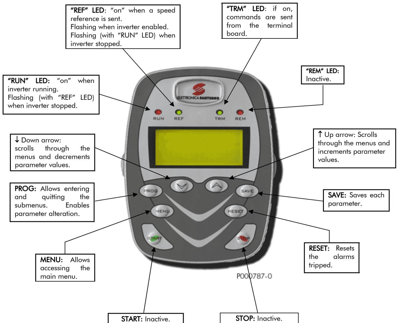
The keypad includes the following keys: **PROG**, **↓**, **↑**, **SAVE**, **MENU**, **RESET**, **START**, **STOP**. They are detailed below.
