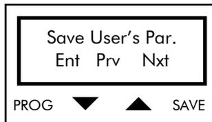
Press PROG to enter the Save User's Parameters submenu. Press ↑ and ↓ to scroll through the other submenus.
