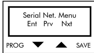
Press PROG to enter the Serial Network submenu. Press ↓ and ↑ to scroll through the other submenus of the Configuration menu.
