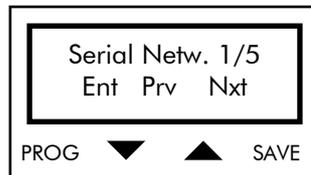
Press PROG to quit the Serial Network submenu. Press ↓ and ↑ to scroll through the parameters.
