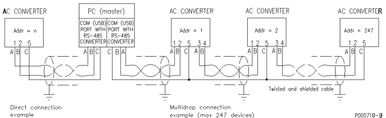
Figure 12: Example of multidrop and direct connection.
