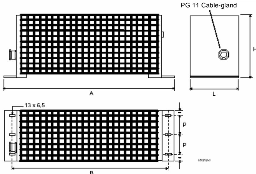
Figure 16: Overall dimensions, 4kW, 8kW, and 12kW braking resistors.
