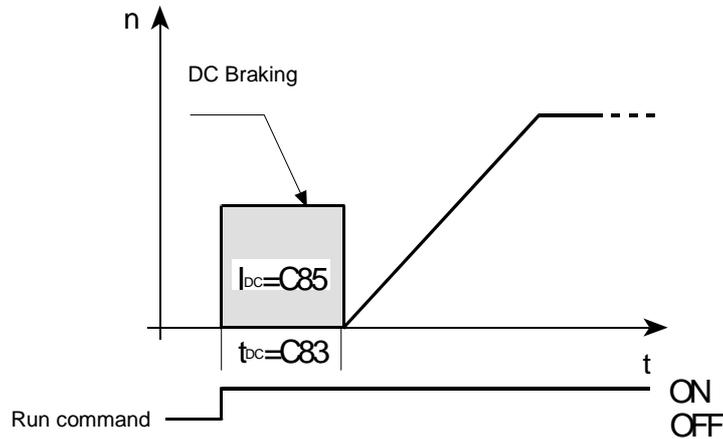
Figure 40: Output frequency/speed and braking DC current when the DC BRAKING AT START function is enabled.
