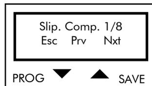
Press PROG to quit the Slip Compensation submenu. Press ↓ and ↑ to scroll through the parameters.
