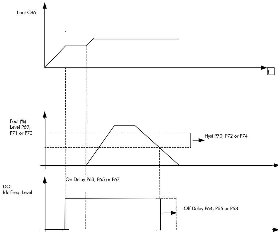
**Figure 52: Characteristics of a digital output programmed as "Idc Freq. Level" in respect to output current variations and output frequency variations in time.**
