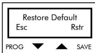
Press PROG (Esc) to quit the Restore Default submenu. Press SAVE to automatically restore the default parameters. The square brackets indicate that parameter restoration is occurring; when square brackets disappear (after a few seconds), parameter restoration is over.
