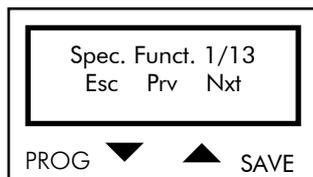
Press PROG to quit the Special Function submenu. Press ↓ and ↑ to scroll through the parameters.
