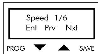
Press  $\uparrow$  (Nxt) and  $\downarrow$  (Prv) to scroll through the parameters up to parameter P44:
