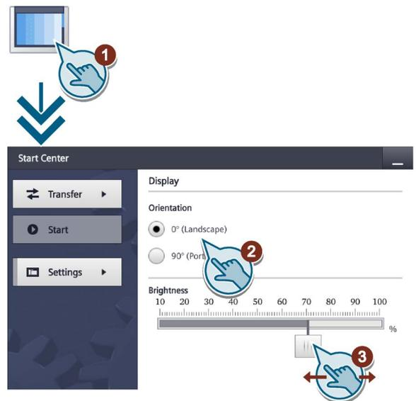
You can set the display brightness of the HMI device to a value between 0% and 100% with the "SetBrightness" system function. If the brightness is set to 0% and the screen saver switches on, touching the display or a key will switch off the screen saver. The brightness then changes back to the value that was set before the system function was called.
