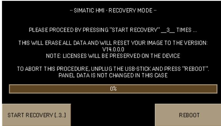
6. To reset the HMI device to factory settings, press the "START RECOVERY (.3.)" button three times in a row and follow the instructions on the display. At the end of the recovery operation, remove the USB stick and press the "REBOOT" button.
