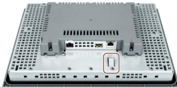
After the power-on test, use a cable tie to secure the connected cables to the marked fixing element in order to provide strain relief.
