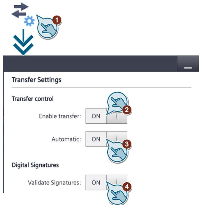
4. To select the check of the signature during transfer of an HMI device image, select "Validate Signatures" = "ON".
