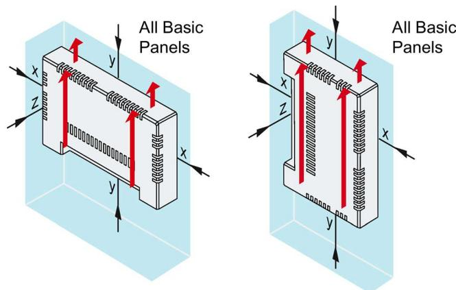
Required clearance around the HMI devices.
