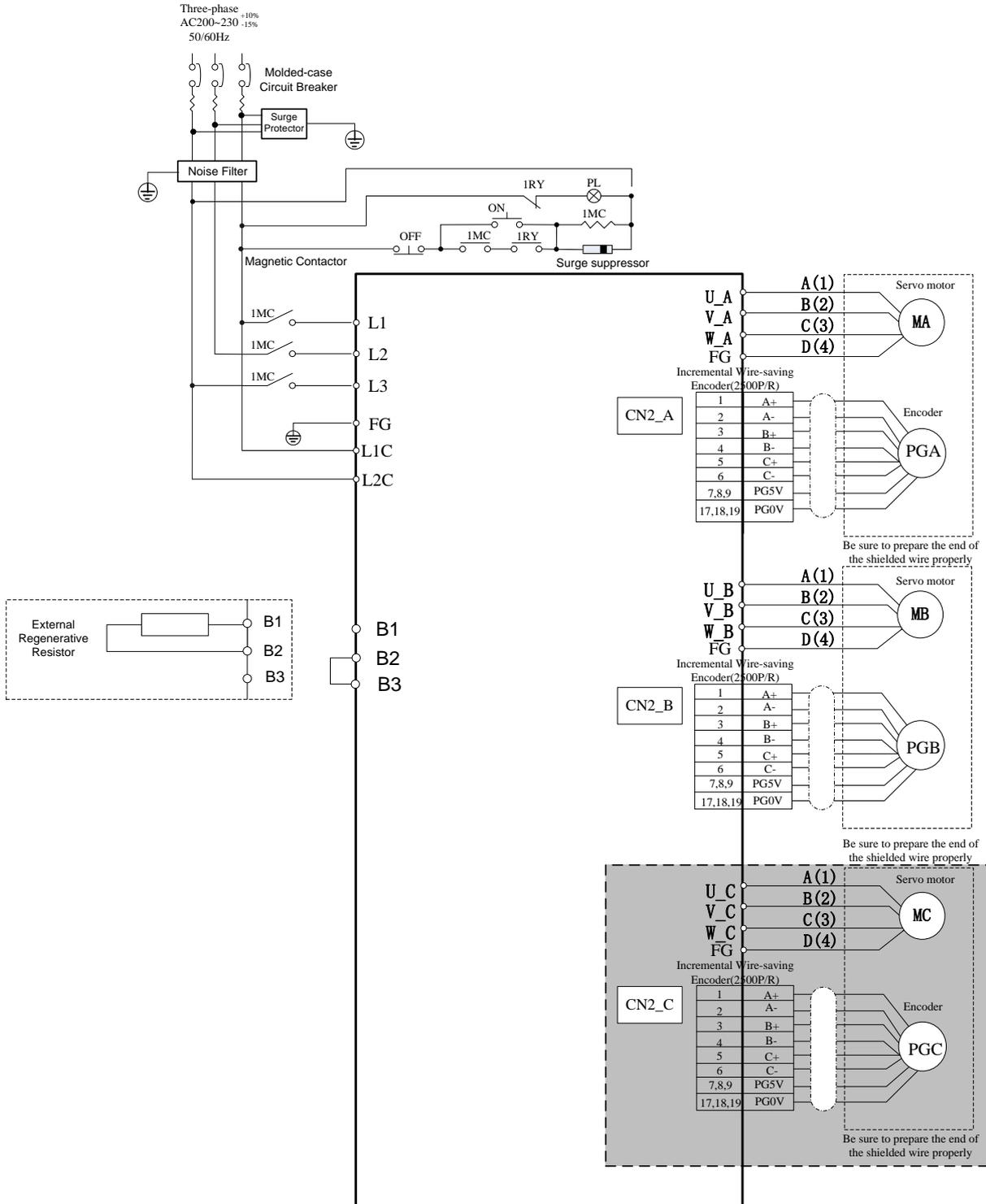
Note :The wiring of ETS-IR two-axis servo drive does not include the gray part of graph.
