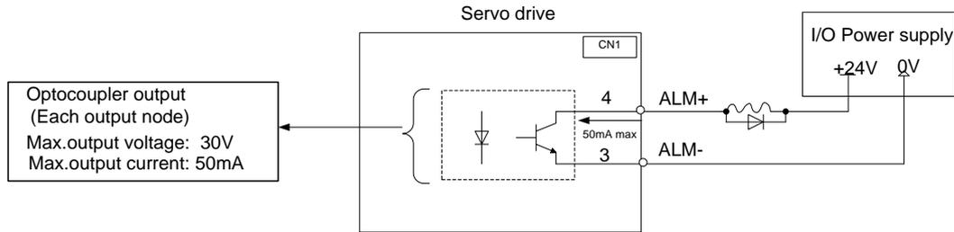
An external +24V I/O power supply is required since there is no +24V power source available inside the servo drive.
