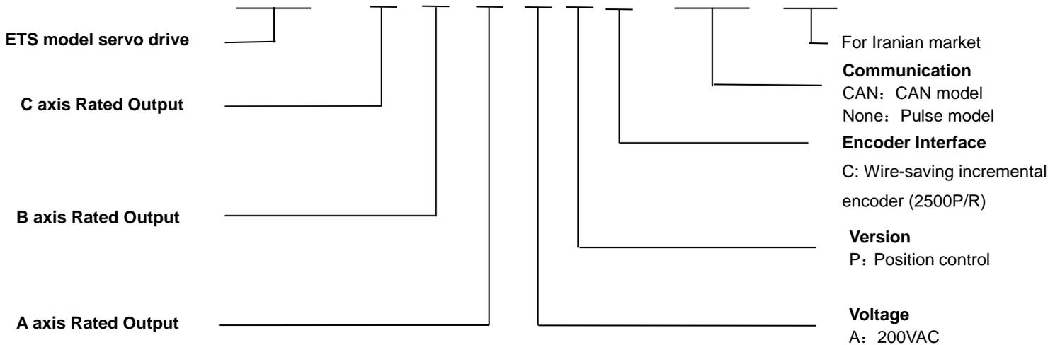
Notes: Each axis of ETS-IR servo drive equips 50W、100W、200W、400W、750W、1.0kW servo motor, and assures three times overload capacity.
