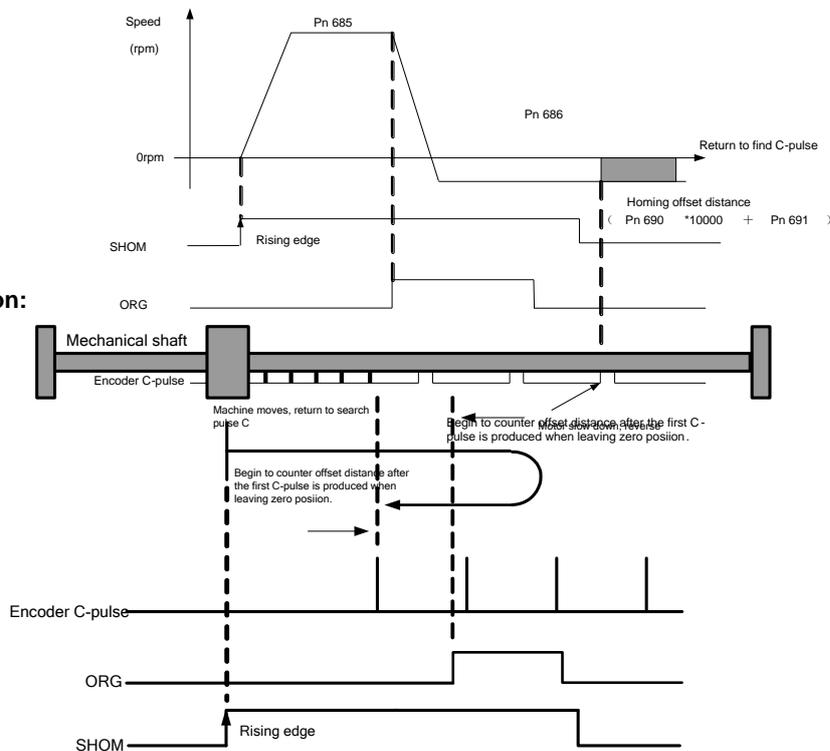
**After hitting the origin signal ORG, the motor will find C-pulse directly; the figure is shown as below:**
