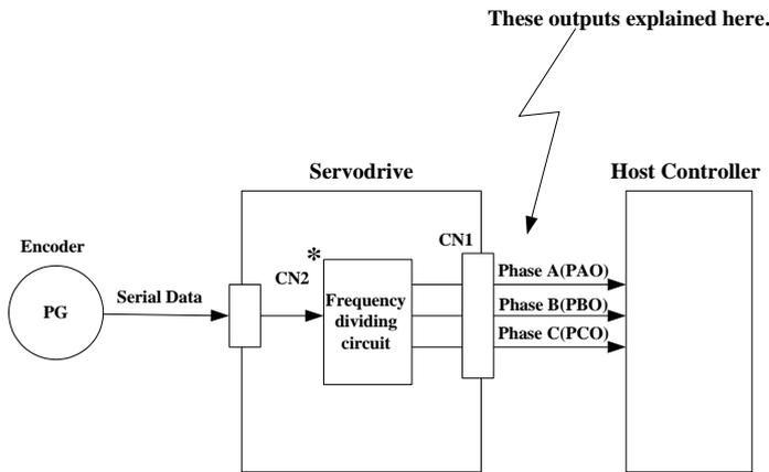
\*The dividing output phase form is the same as the standard setting(Pn001.0=0) even if in reverse rotation mode(Pn001.0=1).
