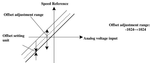
Adjust the speed reference offset manually in the following procedure.
