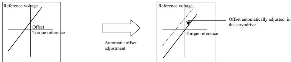
After completion of the automatic adjustment, the amount of offset is stored in the servo drive. The amount of offset can be checked in the manual adjustment of torque reference offset(Fn004).
