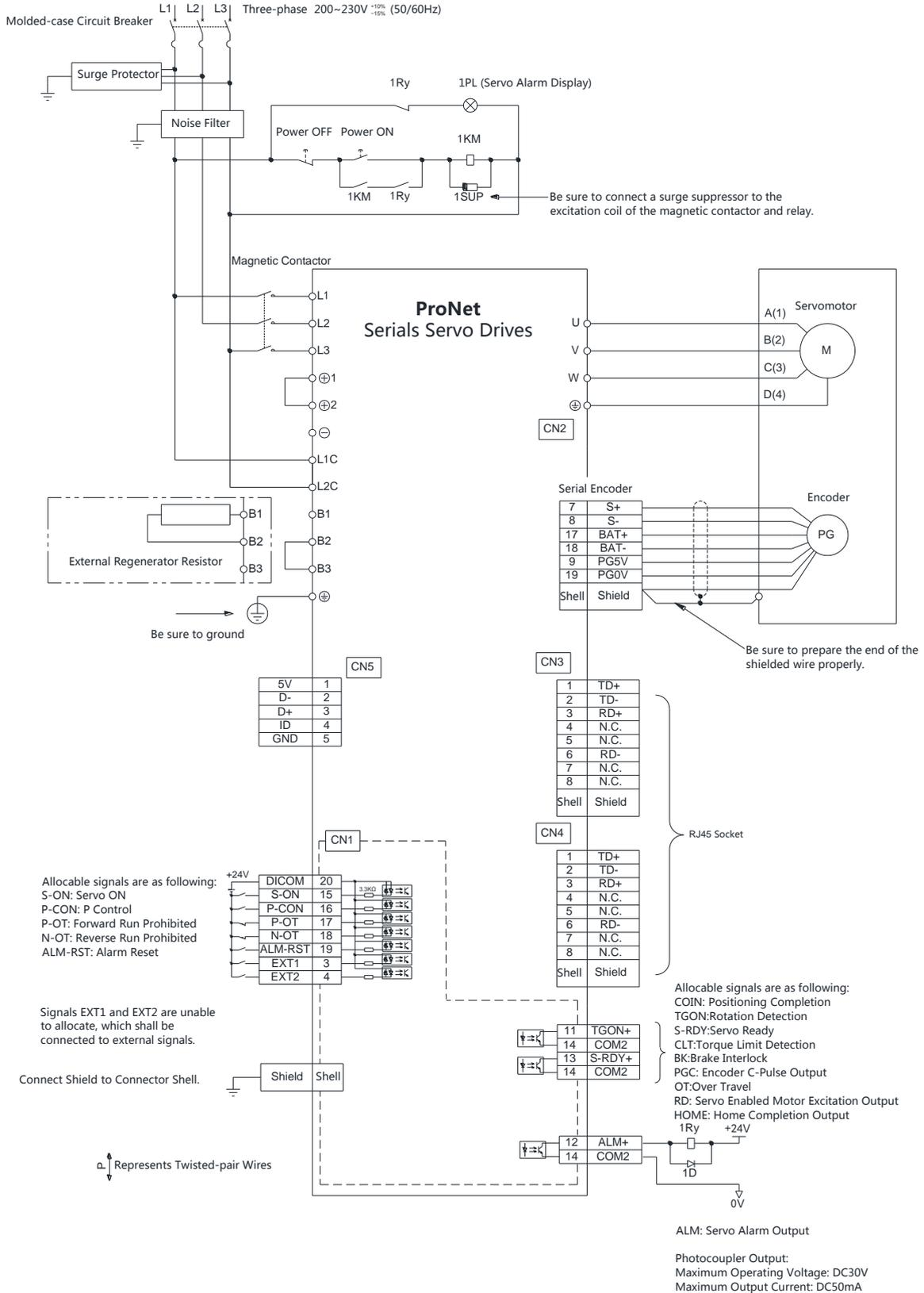
The standard wiring example of ProNet-□□□EG-EC servo drives is as shown in the following figure.
