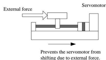
1. The servomotor with the built in brake, is a de-energization brake. It is used to hold the servomotor and cannot be used as a braking purposes. Use the holding brake only to hold a stopped servomotor.
