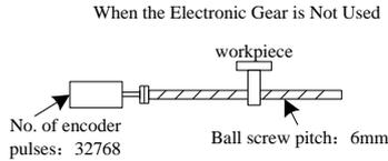
To move a workpiece 10mm :
