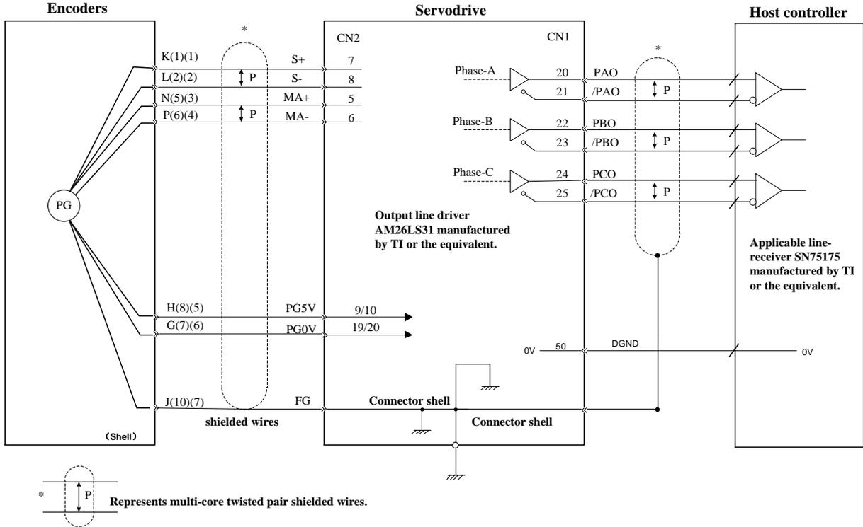
Note: The pin numbers for the connector wiring differ depending on the servomotors.
