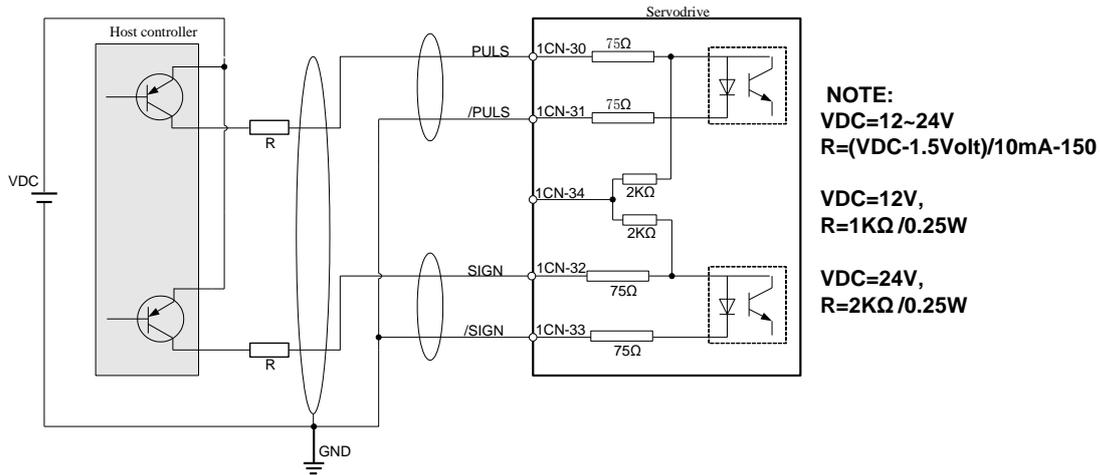
**Note:** When the host controller is applied by open-collector signal output, the input signal noise margin lowers. When a position error caused by the noise occurs, set the parameter Pn006.3.
