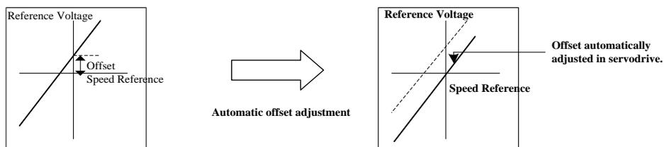
After completion of the automatic adjustment, the amount of offset is stored in the servo drive. The amount of offset can be checked in the speed reference offset manual adjustment mode (Fn004). Refer to **4.5.3 (2) Manual Adjustment of the**
