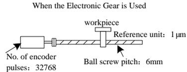
To move a workpiece 10mm using reference units:
