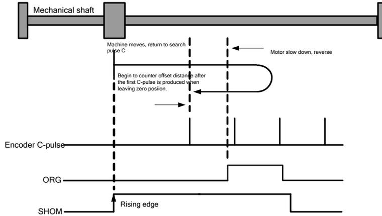
**After hitting the origin signal ORG, the motor will find C-pulse directly; the figure is shown as below:**
