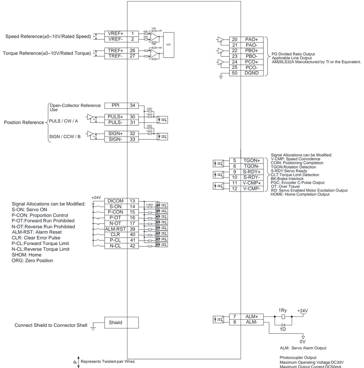
The I/O signal connections diagram of the ProNet-□□□EG-EC servo drives is as shown in the following figure.
