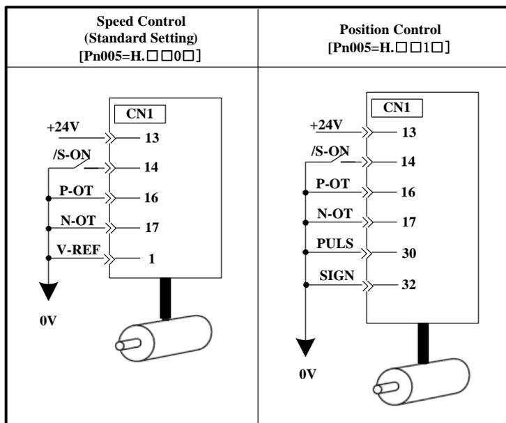
**(2) Operating Procedure in Speed Control Mode (Pn005=H. □□0□)**
