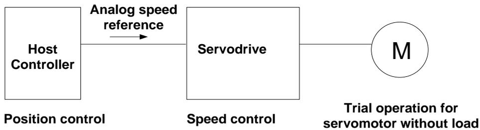
When the servo drive conducts speed control and position control is conducted at the host controller, perform the operation below, following the operation in **Operation Procedure in Speed Control Mode (Pn005=H. □□0□)**.
