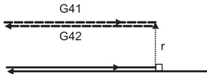
(5) When the compensation direction is switched using G41/G42, it is possible that the arc may exceed 360°. If the arc exceeds 360°, compensation will be performed as shown in the figure and uncut section will be left.
