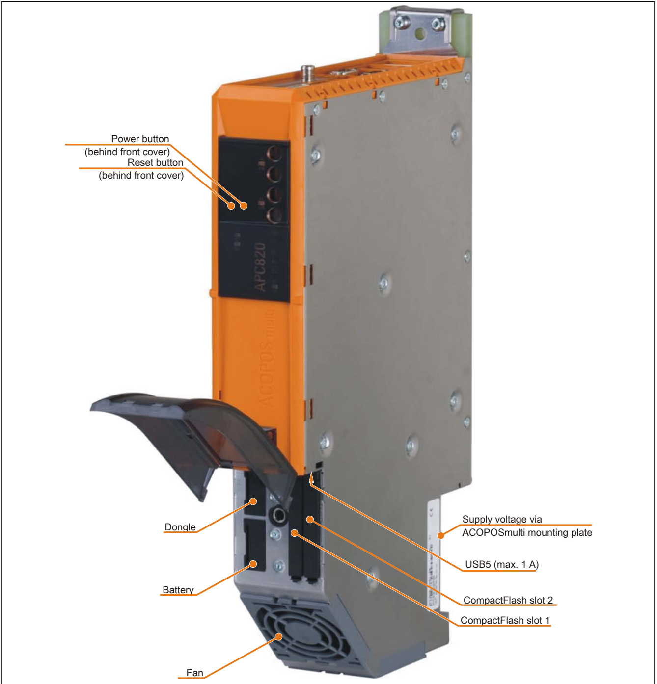
Figure 8: APC820 interface overview - Front side \geq A1
