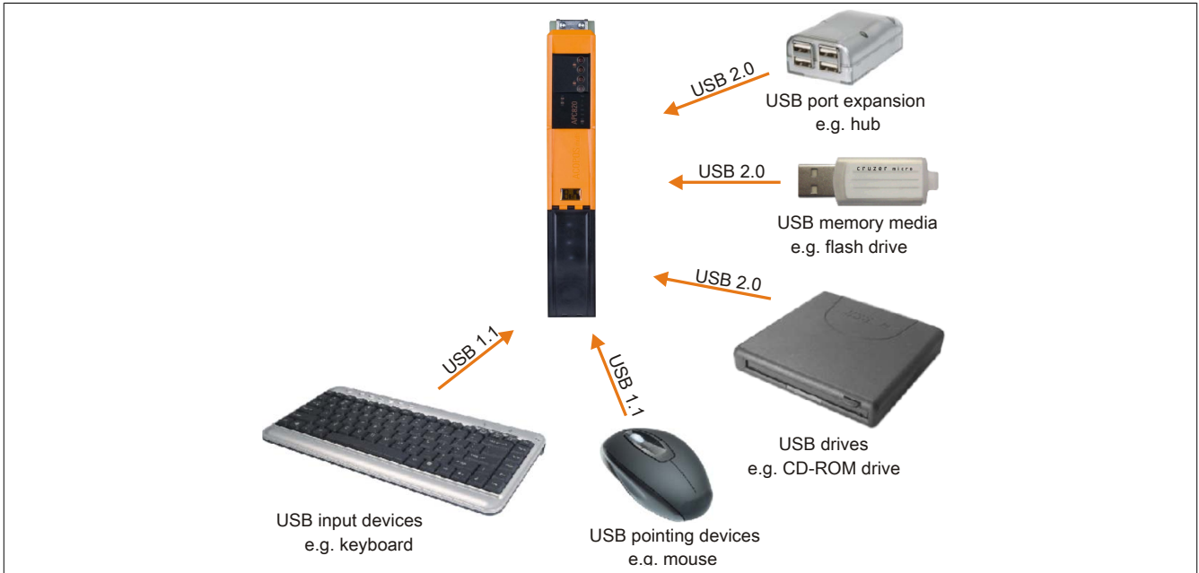
Figure 29: Local connection of USB peripheral devices on the APC820
