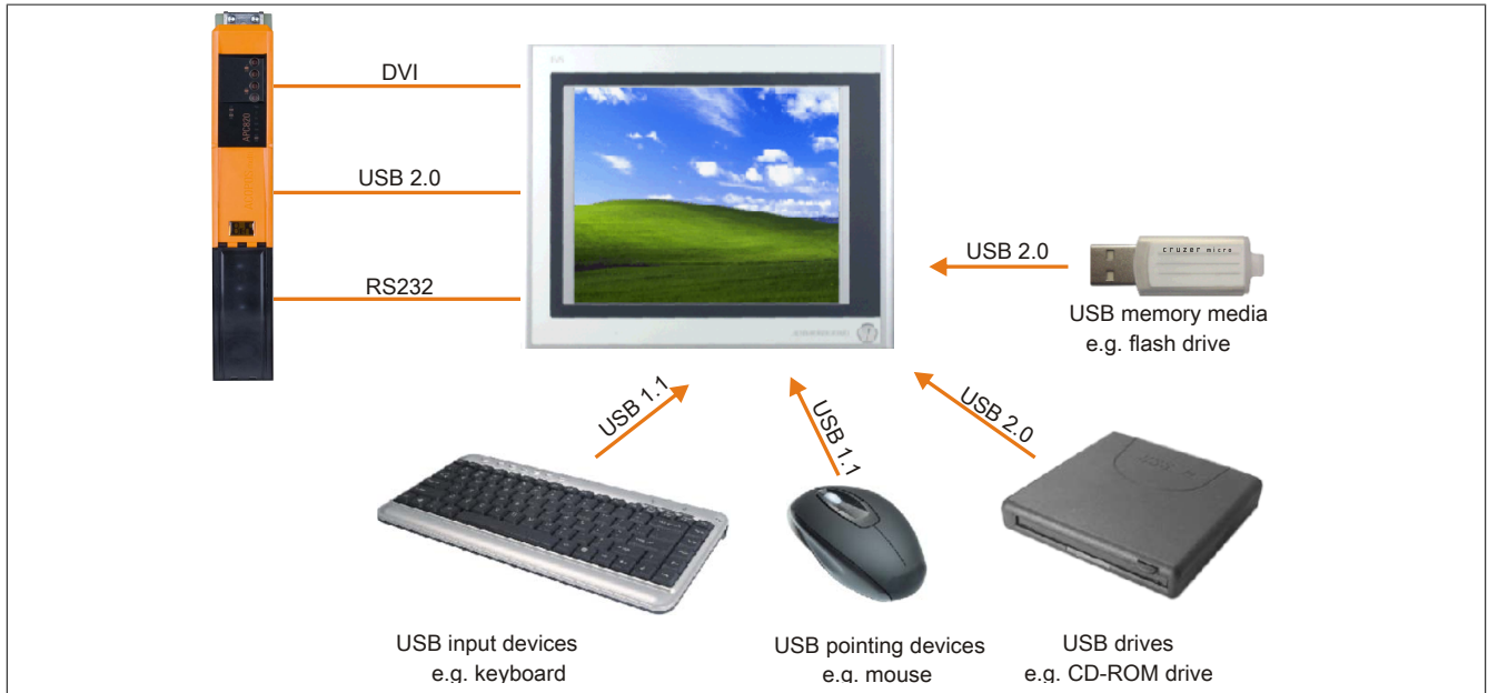
Figure 30: Remote connection of USB peripheral devices on the APC900 via DVI
