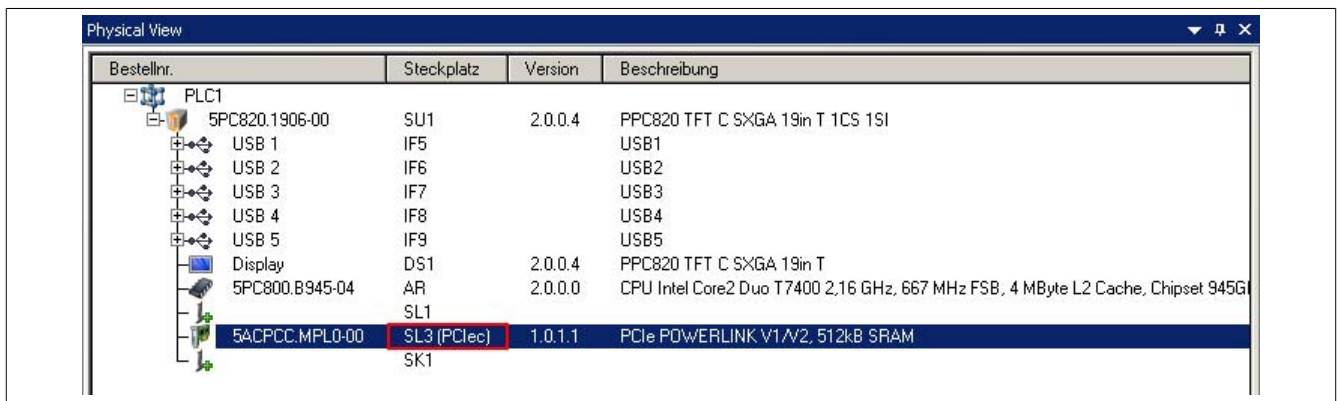
Figure 16: Integrating the POWERLINK plug-in card in Automation Studio
