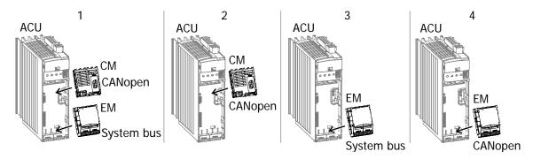
The frequency inverter must be extended by either the CANopen® communication module CM-CAN or a fitting EM module for the CAN connection.
