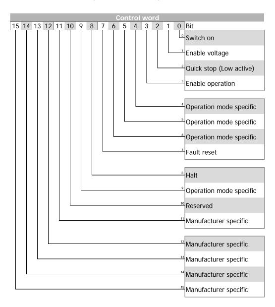
Bits 9 ... 15 are used depening on the configuration and on 0x6060 Mode of Operation.
