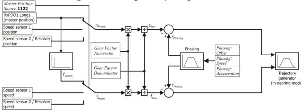
The master position and speed is multiplied with the *gear factor*. When a *Phasing* is started, the Phasing profile is added to the Master Speed until the Phasing offset is reached.
