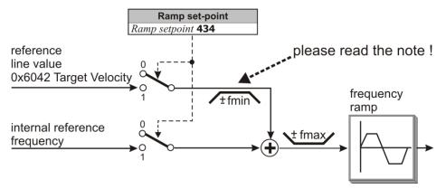
The internal reference value from the reference frequency value channel and the reference line value can be fed to the ramp individually or as an added variable. Setting is carried out via the data set change-over capable parameter *Ramp setpoint* **434**.
