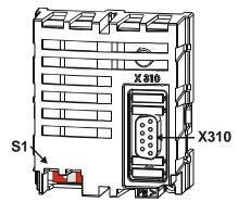
The **X310** (9-pole Sub-D) bus plug has been designed according to DS102 Version 2.0 (Bus node, option A).
