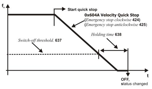
If frequency/speed zero has been reached during the holding time, the drive continues to be supplied with direct current until the switch-off time has expired. With this measure, there is an assurance that the drive is stationary in a change of state.
