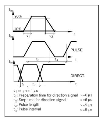
Figure 3-1 Response Time PULSE/DIRECT.
