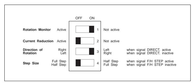
Figure 2-15 Switch Settings Parameter Switch
