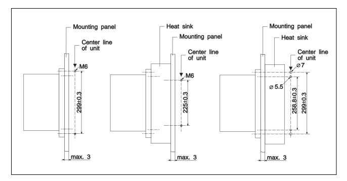
Figure 6-6 Drilling Schemes
