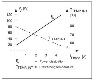
Figure 2-2 Power Dissipation Diagram
