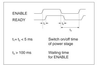
Figure 3-3 ENABLE/READY switching times
