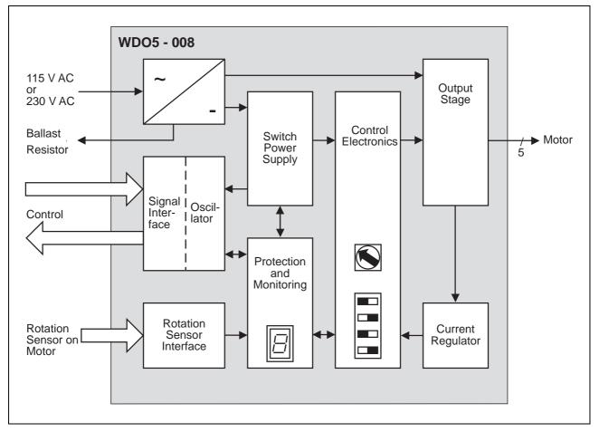
Figure 1-3 Function Connection Diagram WDO5-008
