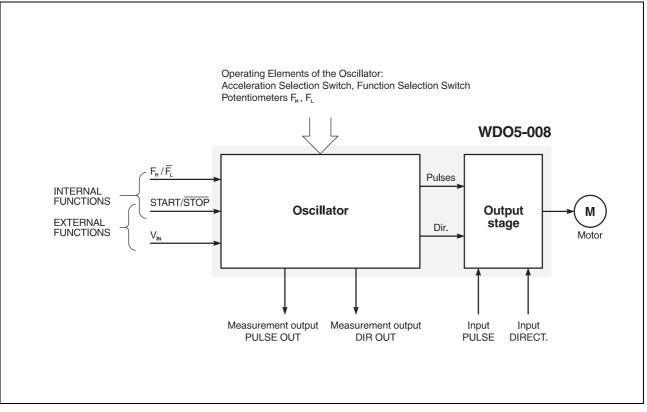
Figure 1-4 Functional Block Diagram, Oscillator
