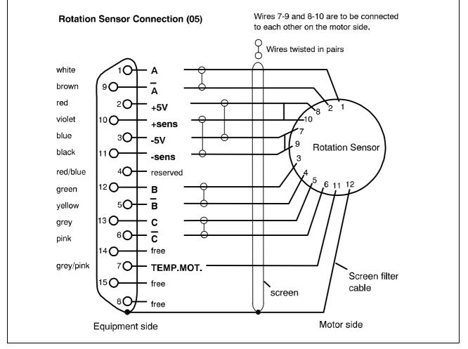
Figure 2-11 Wiring of the Rotation Sensor
