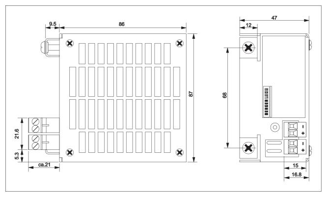
Figure 6-9 Dimensions: Fan Assembly
