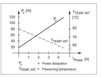
Figure 6-8 Power dissipation diagram
