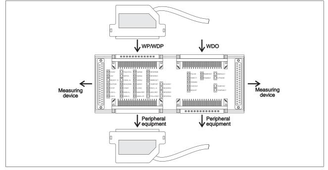
Figure 6-13 Initial Operation of Interface Tester D690
