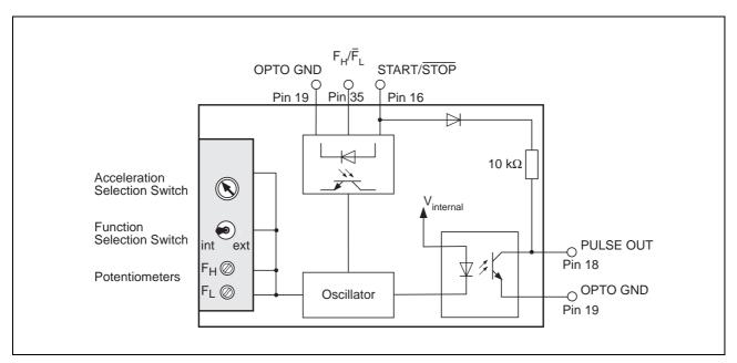
Figure 3-7 Operating Elements, Signal at Oscillator
