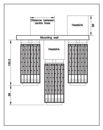
Figure 6-5 Mounting of Heatsink
