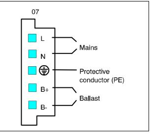
Figure 2-5 Mains and Load Connections
