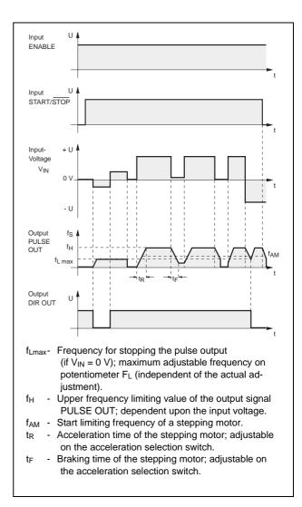
Figure 3-10 Oscillator Signals, Pulse Diagram Using External Mode
