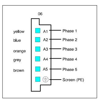
Figure 2-4 Motor Connection
