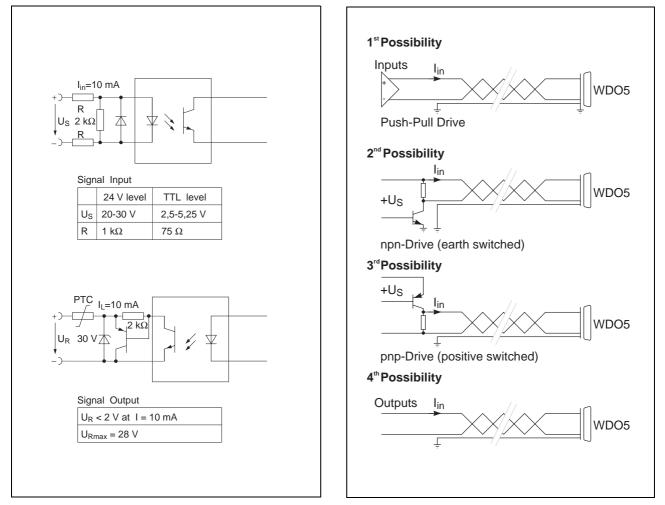
Figure 2-7 Internal Connections of Signal Interface
