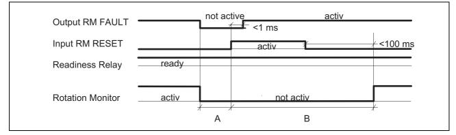
Figure 3-4 Signal Times RM RESET
