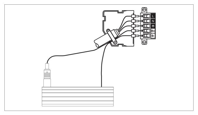
Figure 6-2 Ballast Resistor Connection
