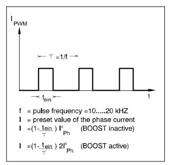
Figure 3-2 Phase Current Control via input IPWMIN
