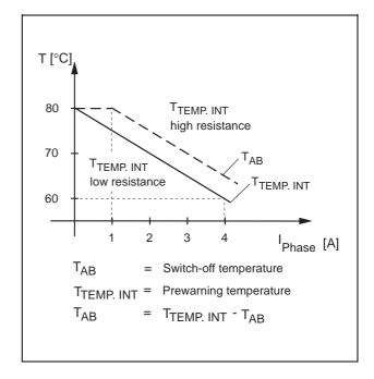
Figure 3-6 Typical Switch Behaviour TEMP. INT. in Dependence on Phase Current and the Heatsink Temperature
