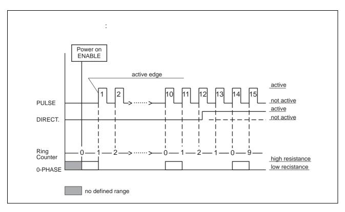
Figure 3-5 Dependance of the 0-PHASE Output on the Ring Counter count at Full Step
