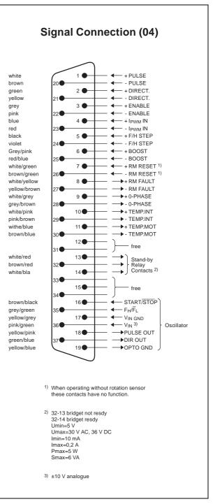
Figure 2-6 Wiring the Signal Socket
