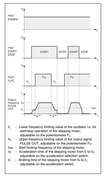
Figure 3-8 Oscillator Signals, Pulse Diagram with Internal Mode
