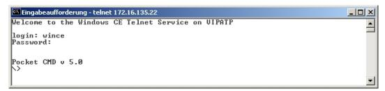
By entering  $\mathtt{Exit}$  res. closing the window you can terminate the Telnet connection at any time.
