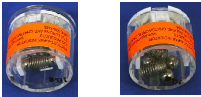
Figure 2–1. Shock Meter Sensor—intact (photo on left) and dislodged (photo on right)
