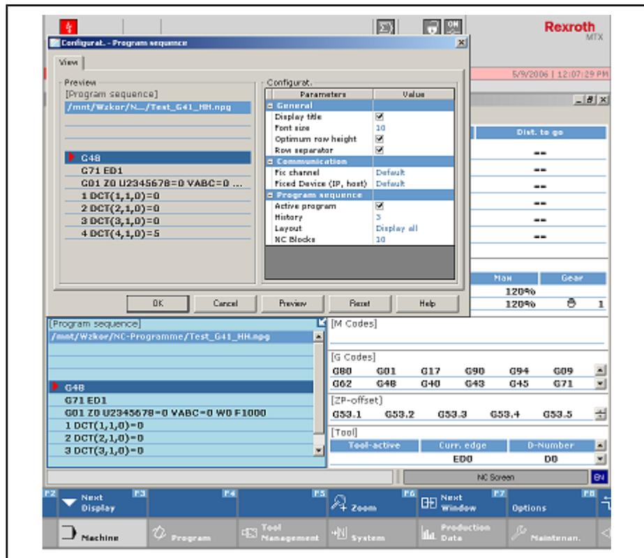
Fig.7-52: *Displaying the NC program section that is currently being processed*
