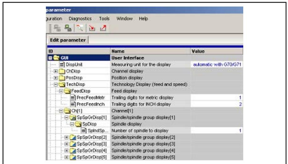
Fig.7-51: Settings options for the technology display in the configurator
