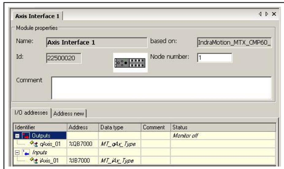
Fig.8-5: "Properties" dialog for the AxisInterface
