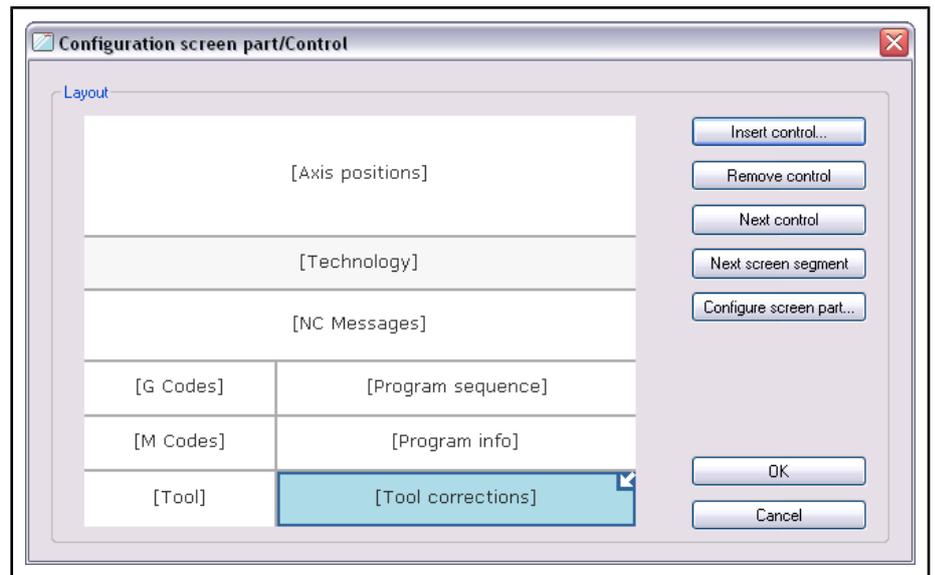
Fig.7-32: Dialog: "Screen segment/control configuration" (Example configuration of the new ACI screen with controls)
