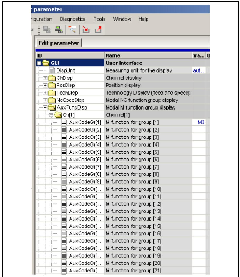
Fig.7-55: Configurator settings for the M-code display
