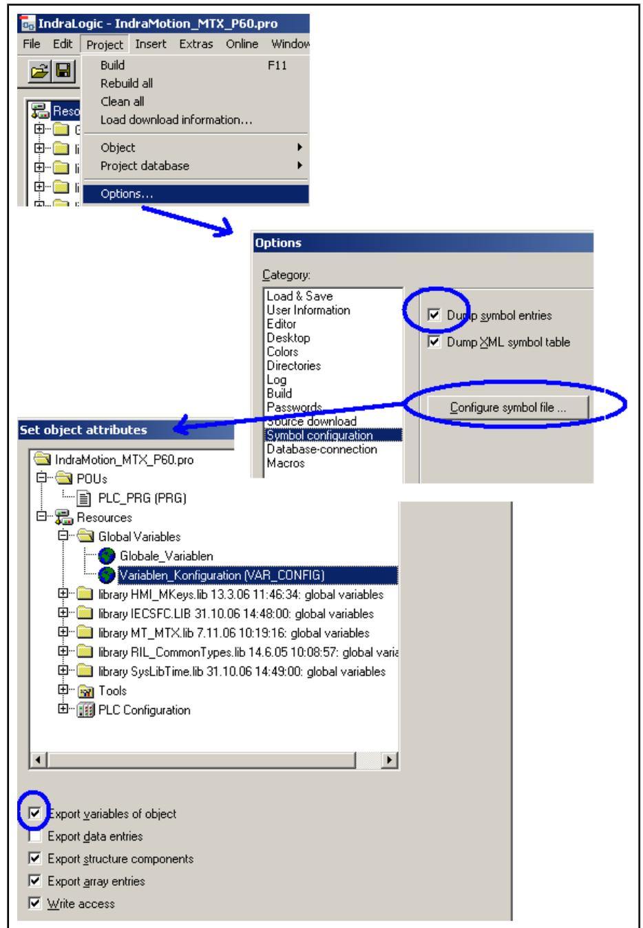
Fig.6-13: Procedure for configuring the symbol file
