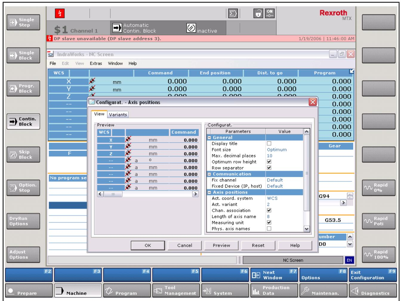
Fig.7-20: Dialog box: Example of a control's own configuration dialog box: "Configuration – Axis positions" of the control for the axis position display
