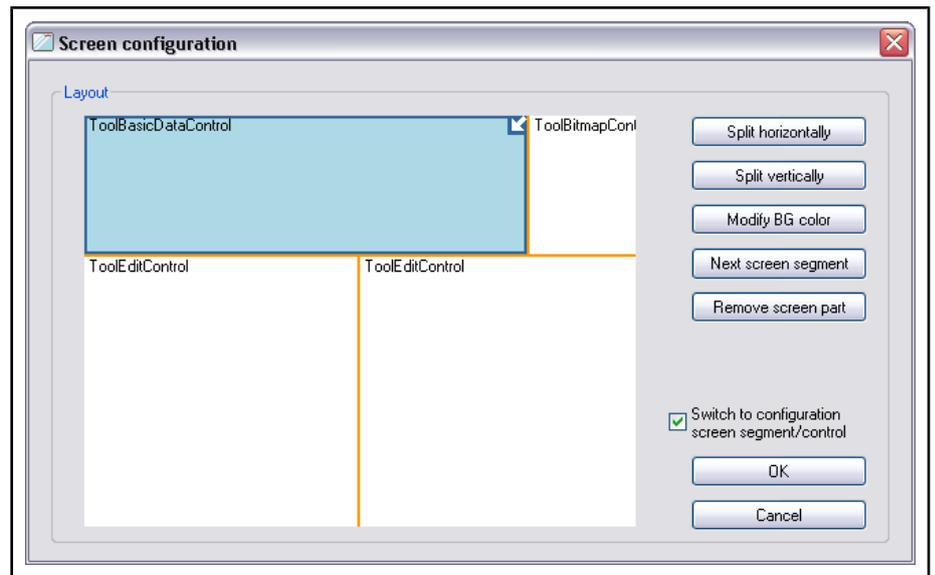
Fig. 16-123: Dialog: "Screen configuration" (with controls without process connection inserted into screen segments)
