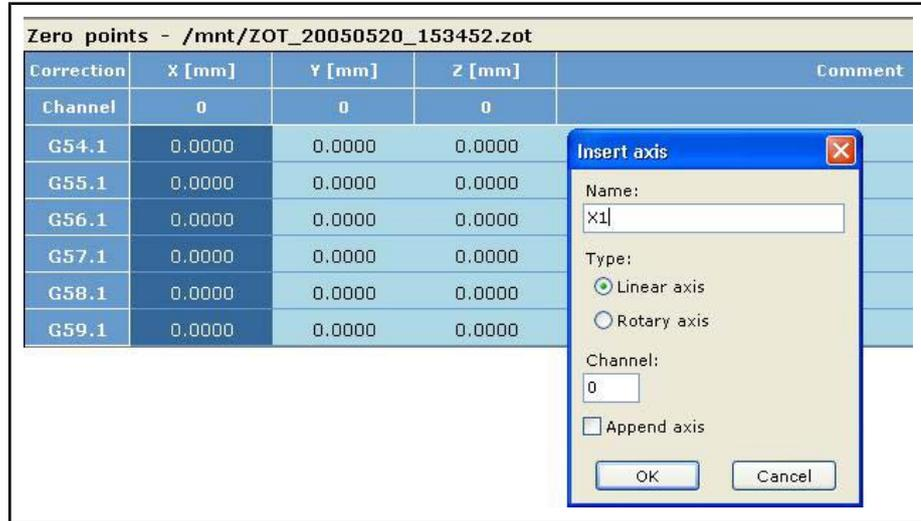
Fig.22-2: Zero offset table: adding axes
