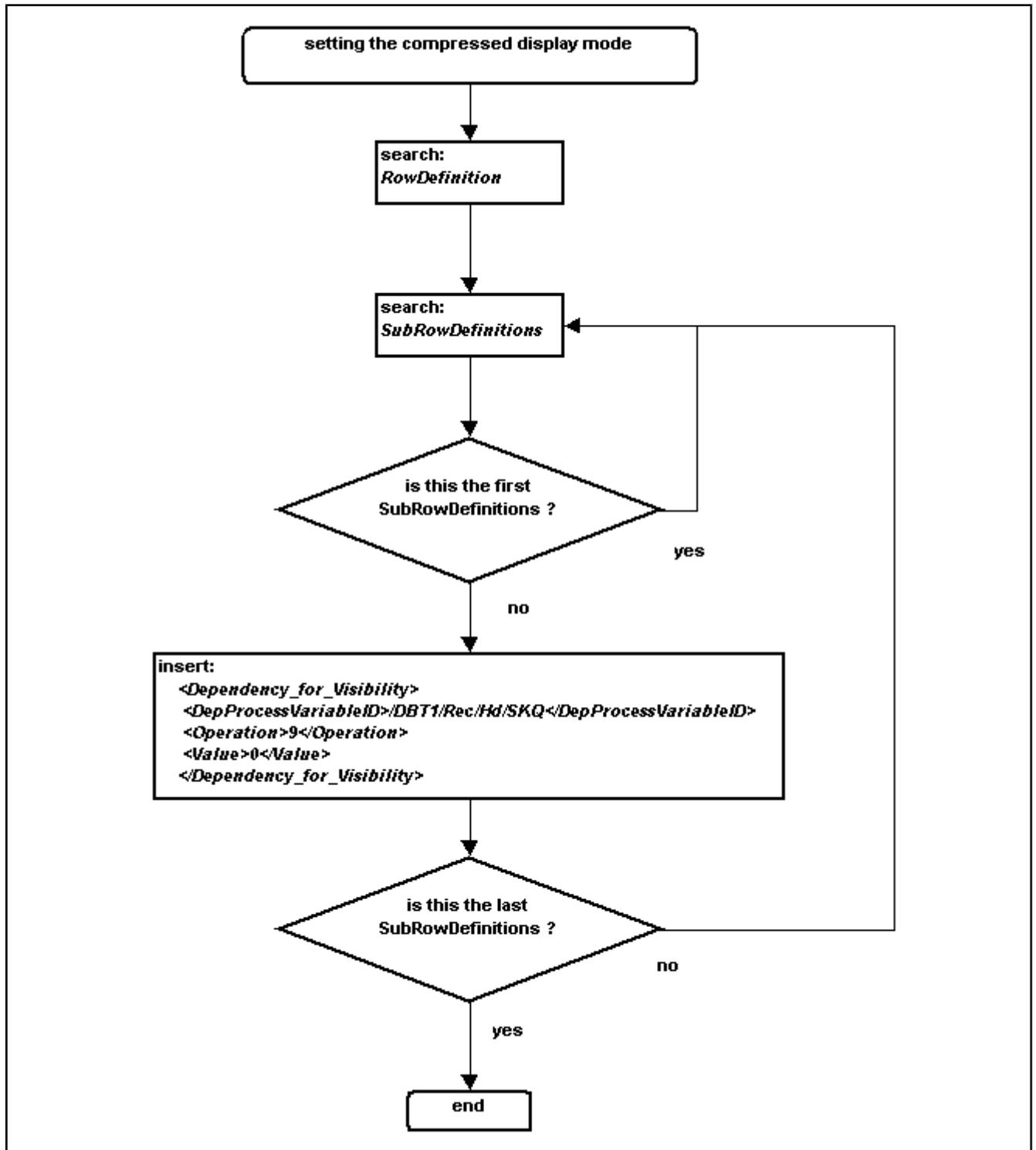
Fig.16-101: Setting the compressed display mode
