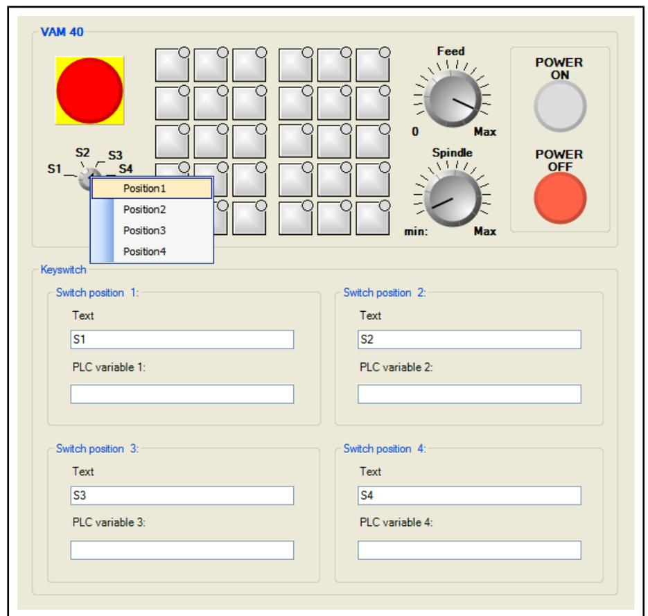
Fig.21-17: Configuration page of the key-operated switch
