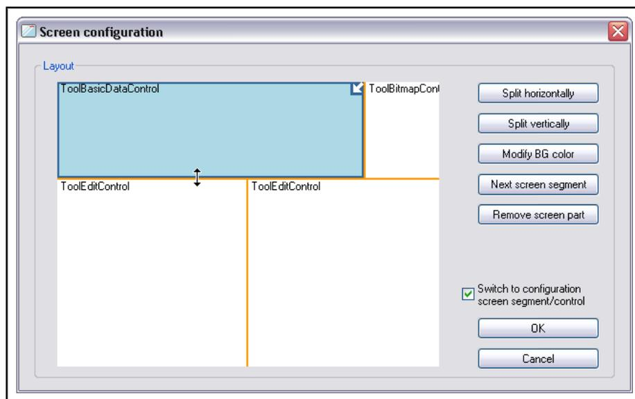
Fig. 16-150: Dialog: "Screen configuration" (cursor symbol indicates the possibility for moving the screen segment divider)
