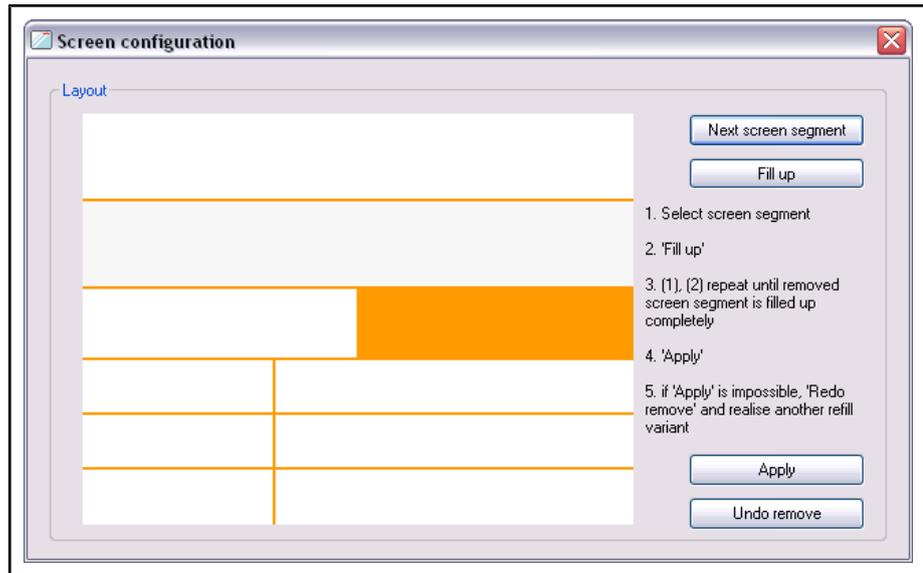
Fig.7-27: Dialog: "Screen configuration" (for filling the deleted screen segment)
