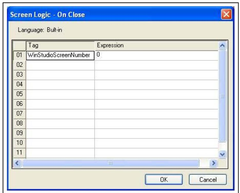
Fig.7-122: Dialog: Screen logic (for entering logic operations that are to be executed when a screen is closed)
