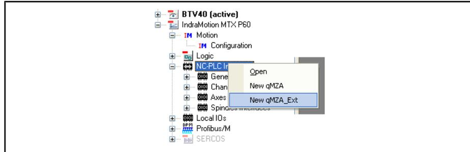
Fig.9-5: Inserting the MSD interface
