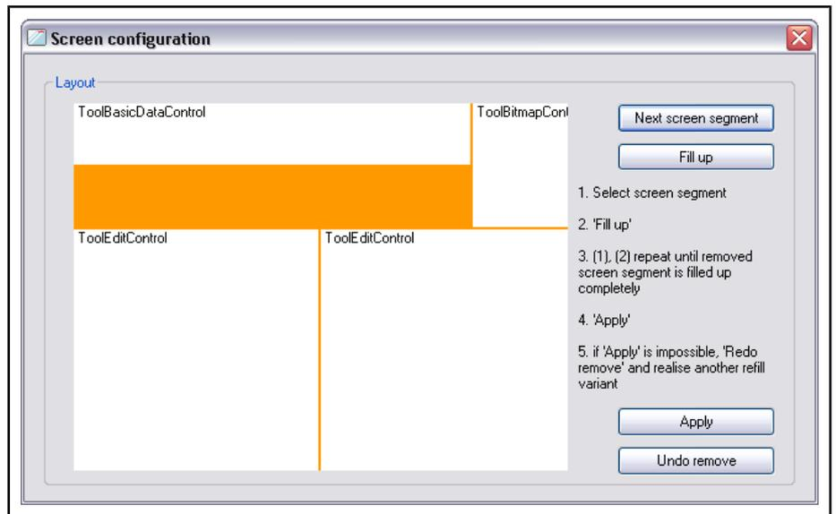
Fig.16-148: Dialog: "Screen configuration" (for filling the deleted screen segment)
