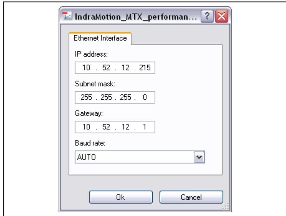
Fig.4-28: Configuration of the Ethernet interface of the MTX control
