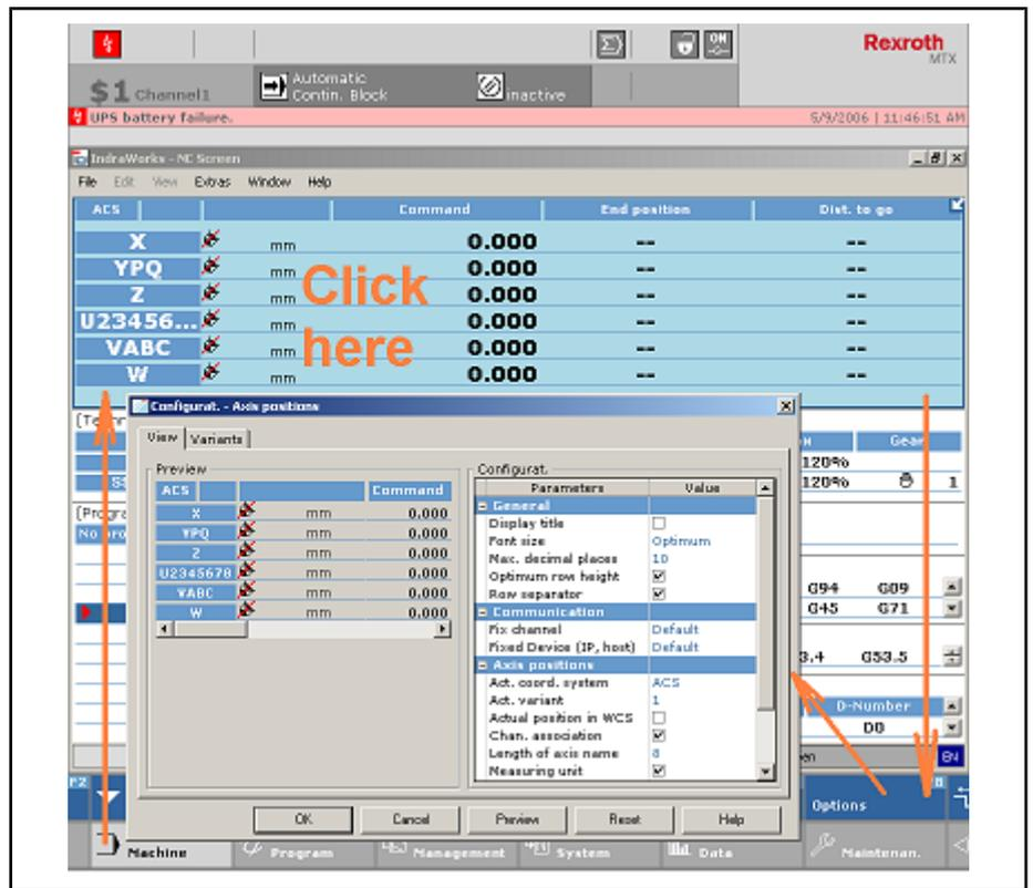
Fig.7-40: Dialog: Configuration axis positions (view)
