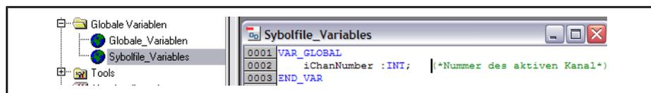
Fig.6-5: Example for generating a variable
