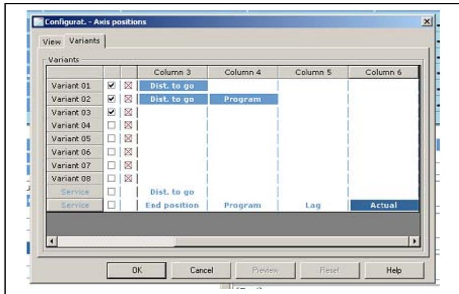
Fig.7-42: Dialog: Configuration axis positions (variants, columns 4-6)
