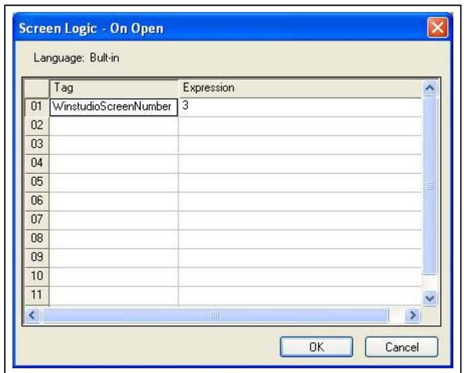
Fig.7-120: Dialog: Screen Logic (logic operations to be executed when calling a screen)
