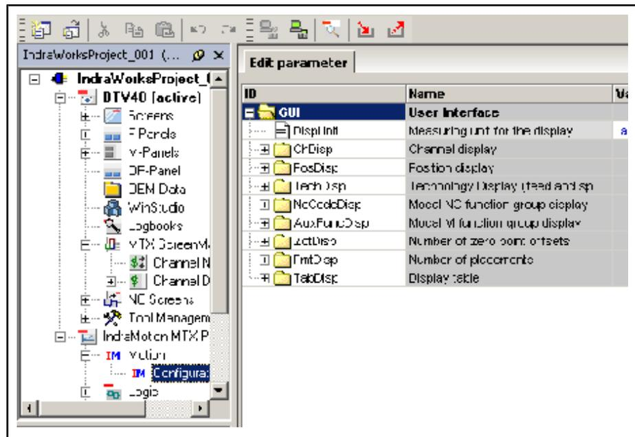
Fig.7-37: Configurator: User interface (GUI) data group
