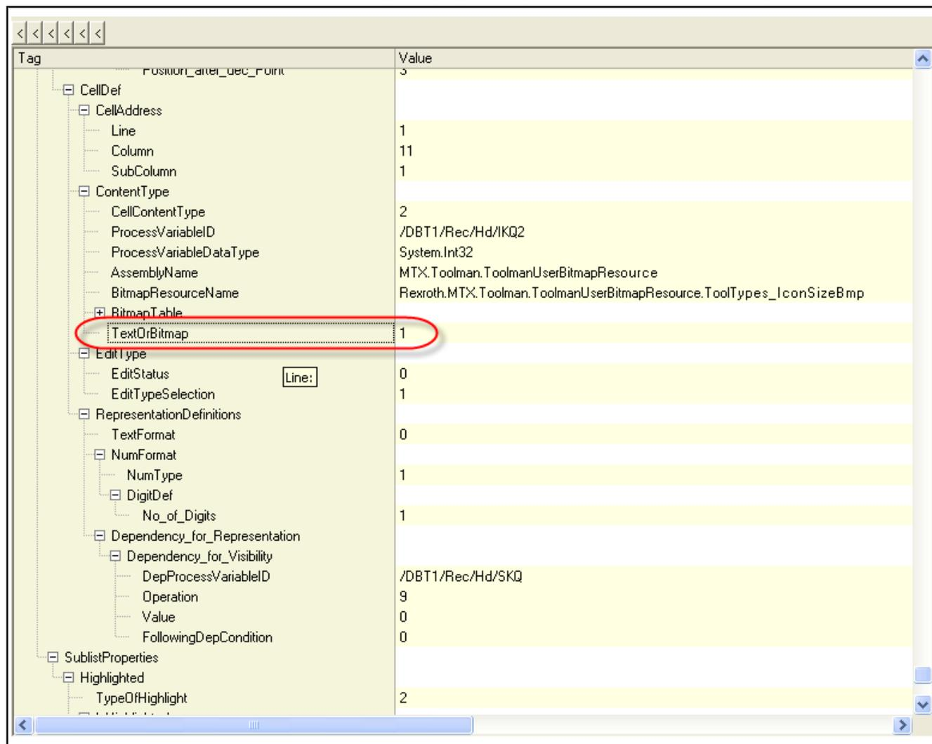
The screenshot shows a configuration file editor with a tree view on the left and a table on the right. The tree view is expanded to 'BitmapTable', and the 'TextOrBitmap' property is highlighted with a red oval and set to '1'. The table on the right shows the following values:
