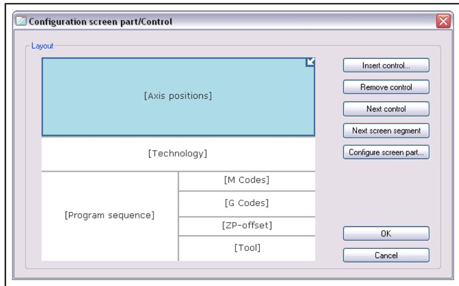
Fig. 7-11: Dialog: Configuration screen segment/control (with controls without process connection)
