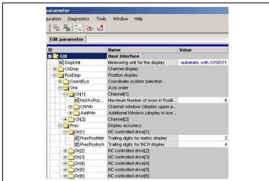
Fig.7-46: Specifying the precision of the position display in the configurator
