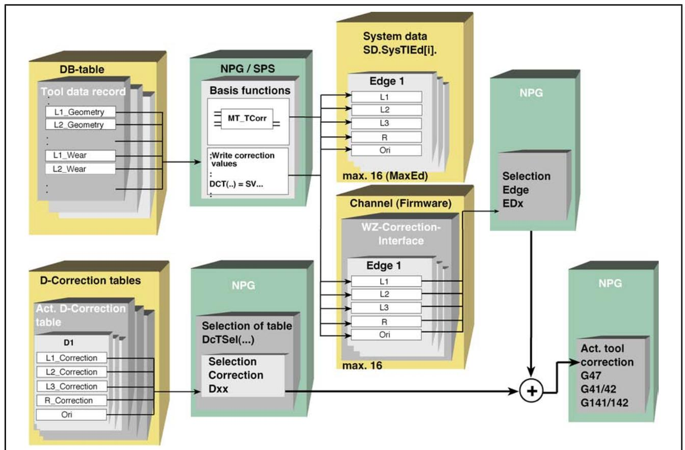
Fig. 16-1: Principle of D-corrections and external tool corrections
