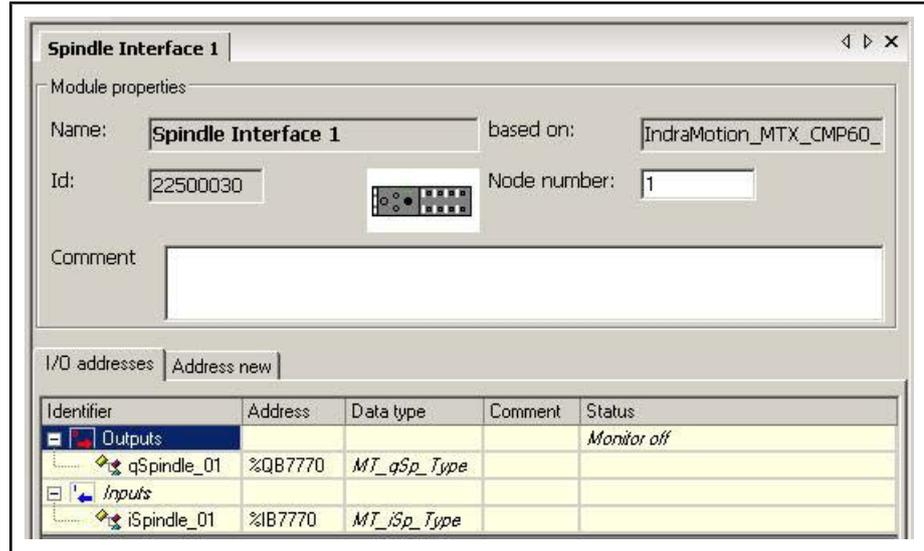
Fig. 8-7: "Properties" dialog for the spindle interface
