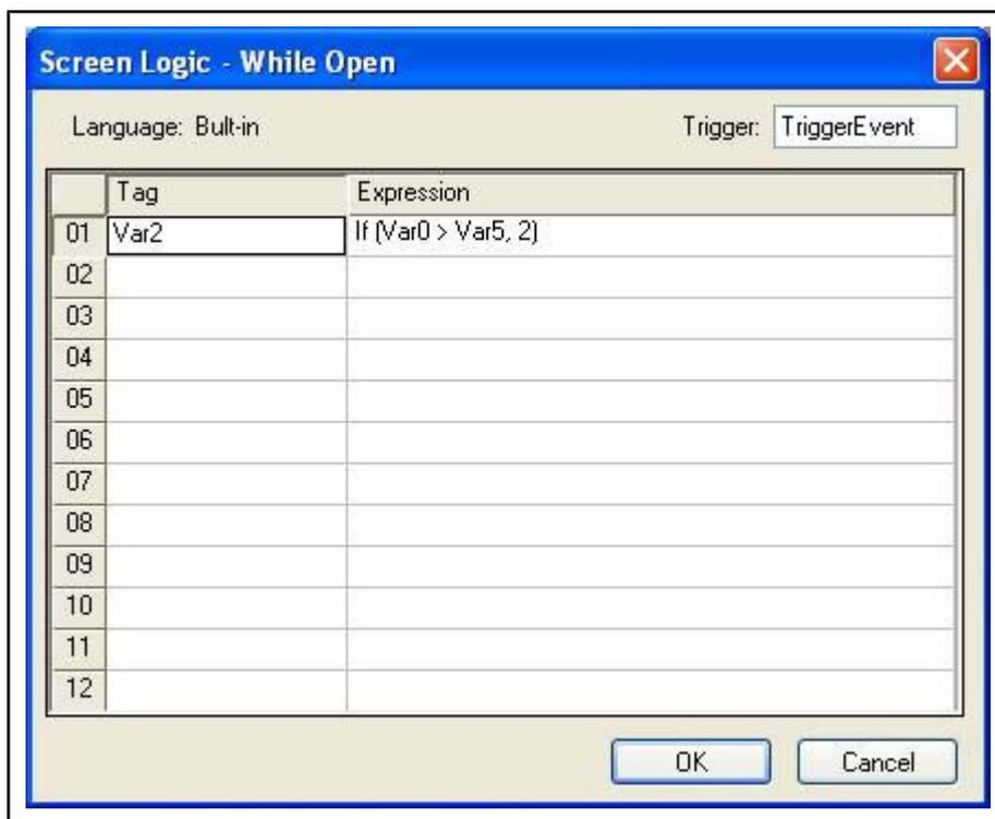
Fig.7-121: Dialog: Screen Logic (for entering logic operations that are to be executed cyclically while a screen is displayed)
