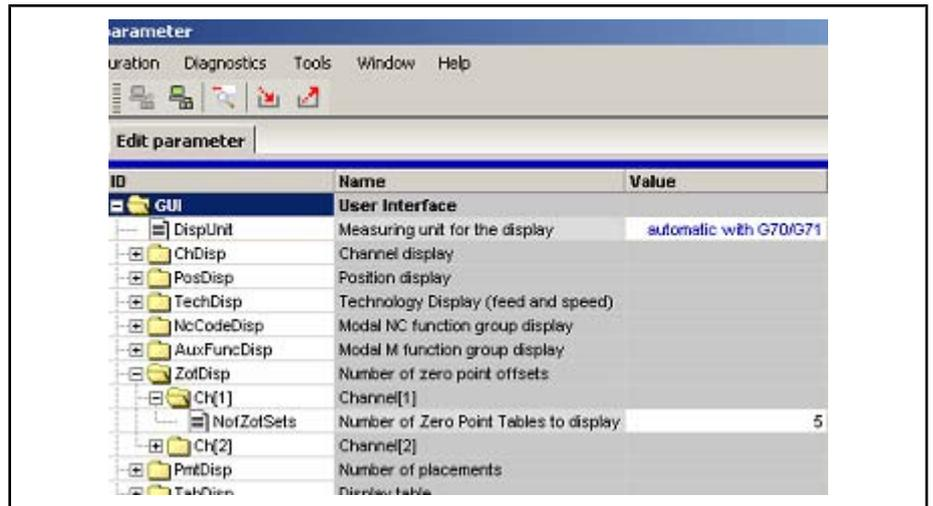
Fig.7-59: Configurator settings for the Z0 display
