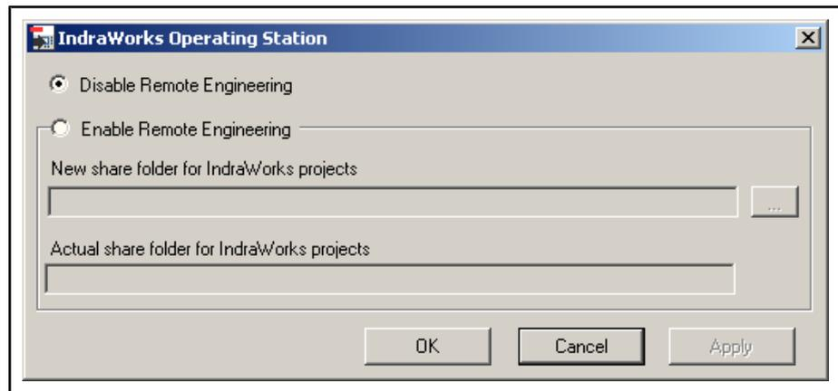
Fig.14-2: Dialog: IndraWorks Operating Station (Remote Engineering configuration)
