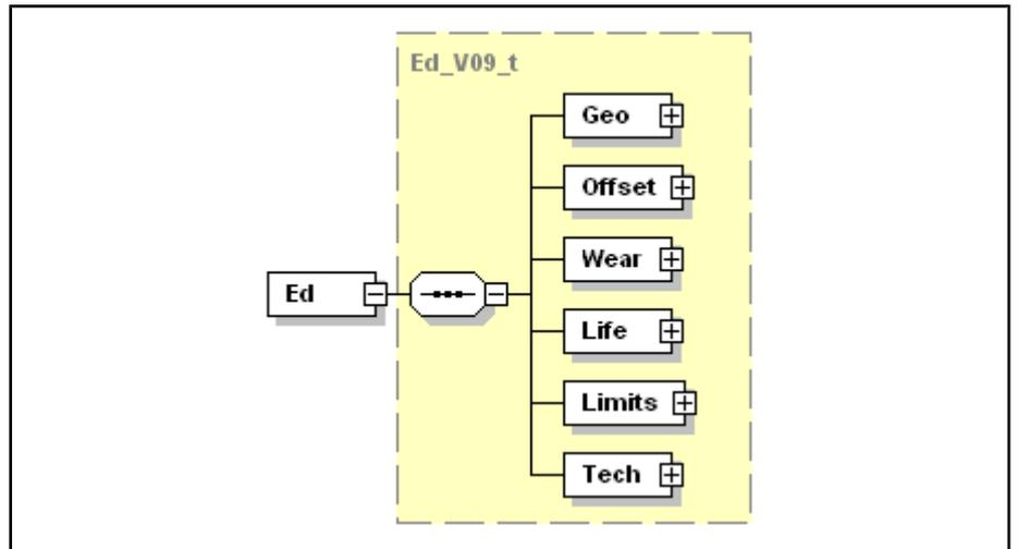
Fig. 16-47: Data record schema (9) (tool edge data upon delivery)
