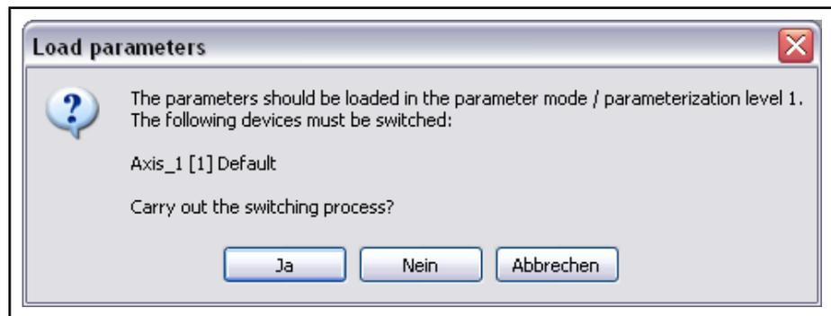
Fig. 12-10: Dialog: Load parameter (error message during the restoration of the drive parameters)
