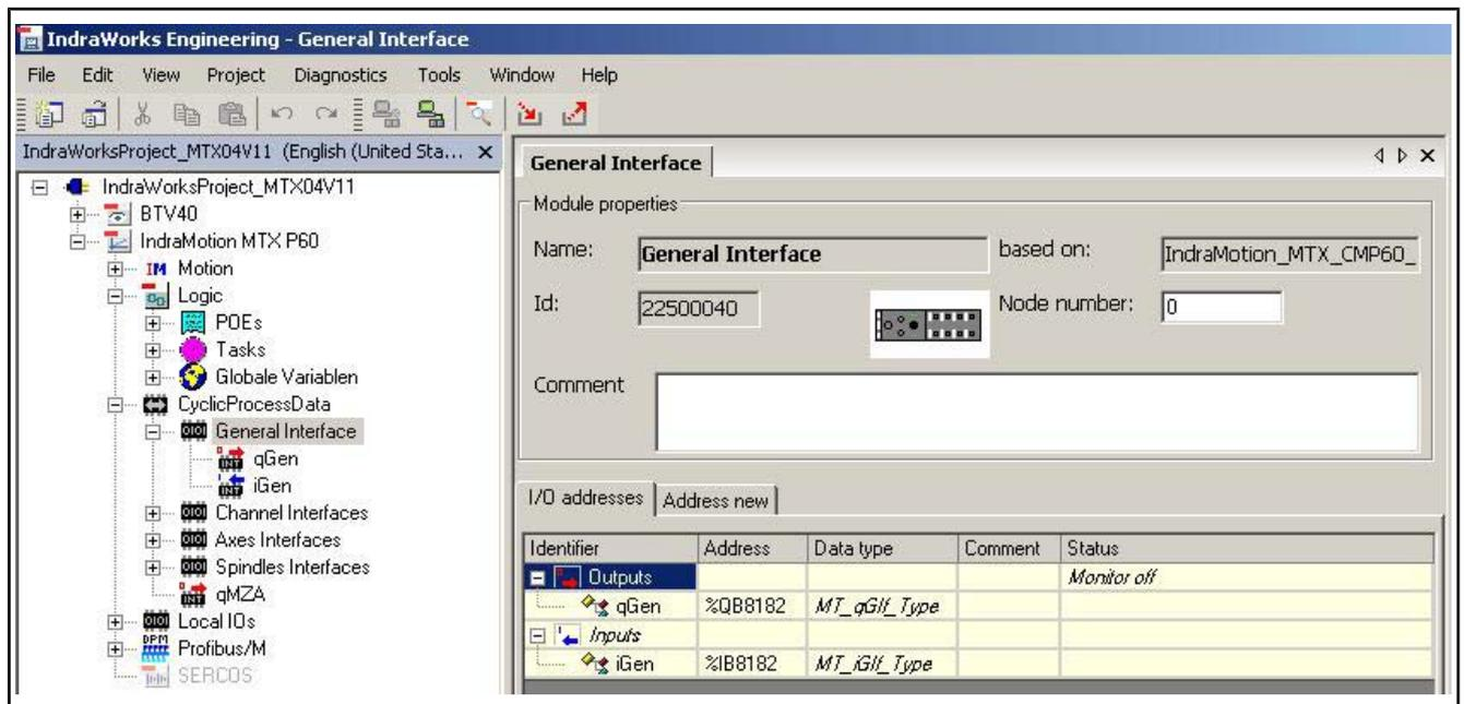
Fig. 8-1: The preset bit interface with the "Properties" dialog for the general interface
