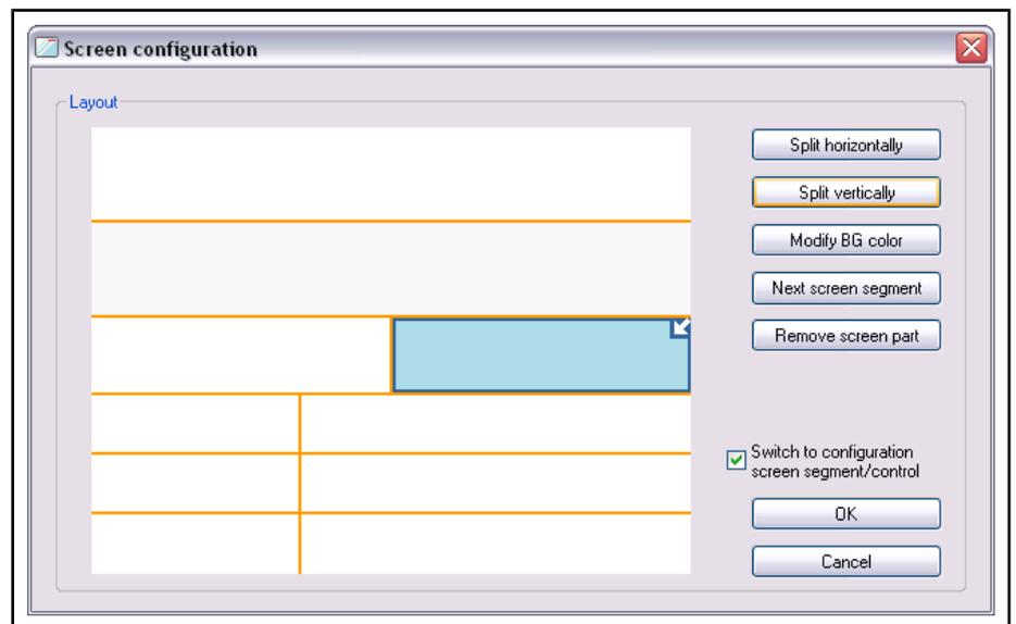
Fig.7-26: Dialog: Screen configuration (division of the new ACI screen after dividing)
