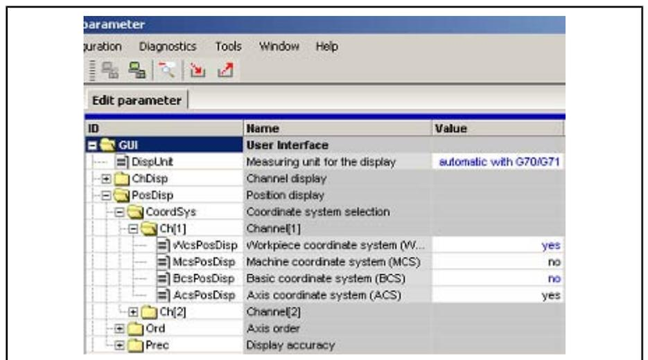
Fig.7-43: Specifying the selectable coordinate systems in the configurator
