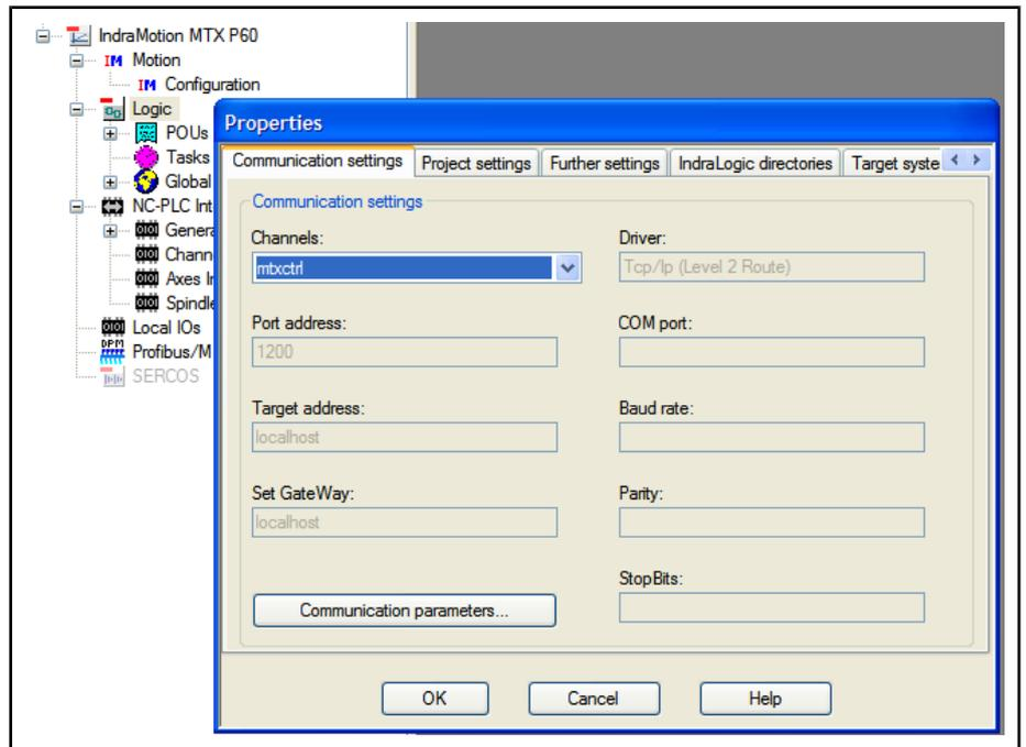
Fig.21-3: PLC communication parameters
