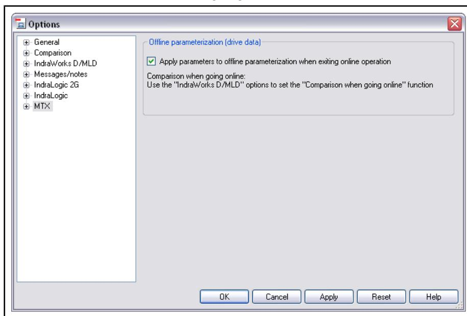
Fig. 5-30: "Option" dialog: Offline parameterization of the MTX
