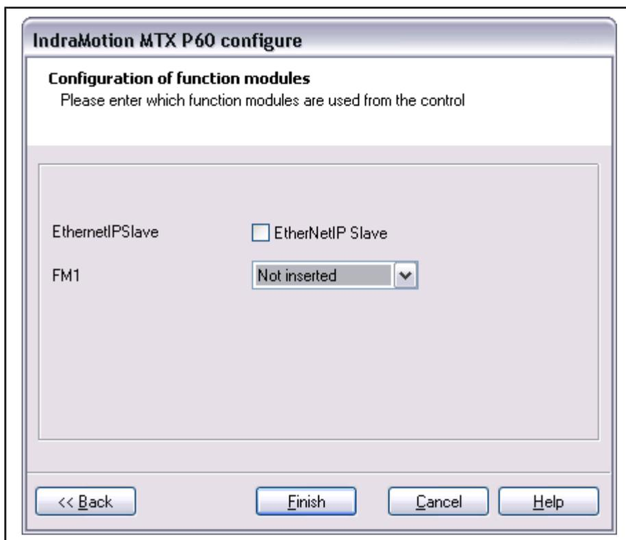
Fig.4-23: Dialog: Configure MTX P60 (configuration of function modules)
