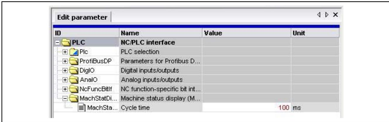
Fig.9-3: Setting MSD message system parameters
