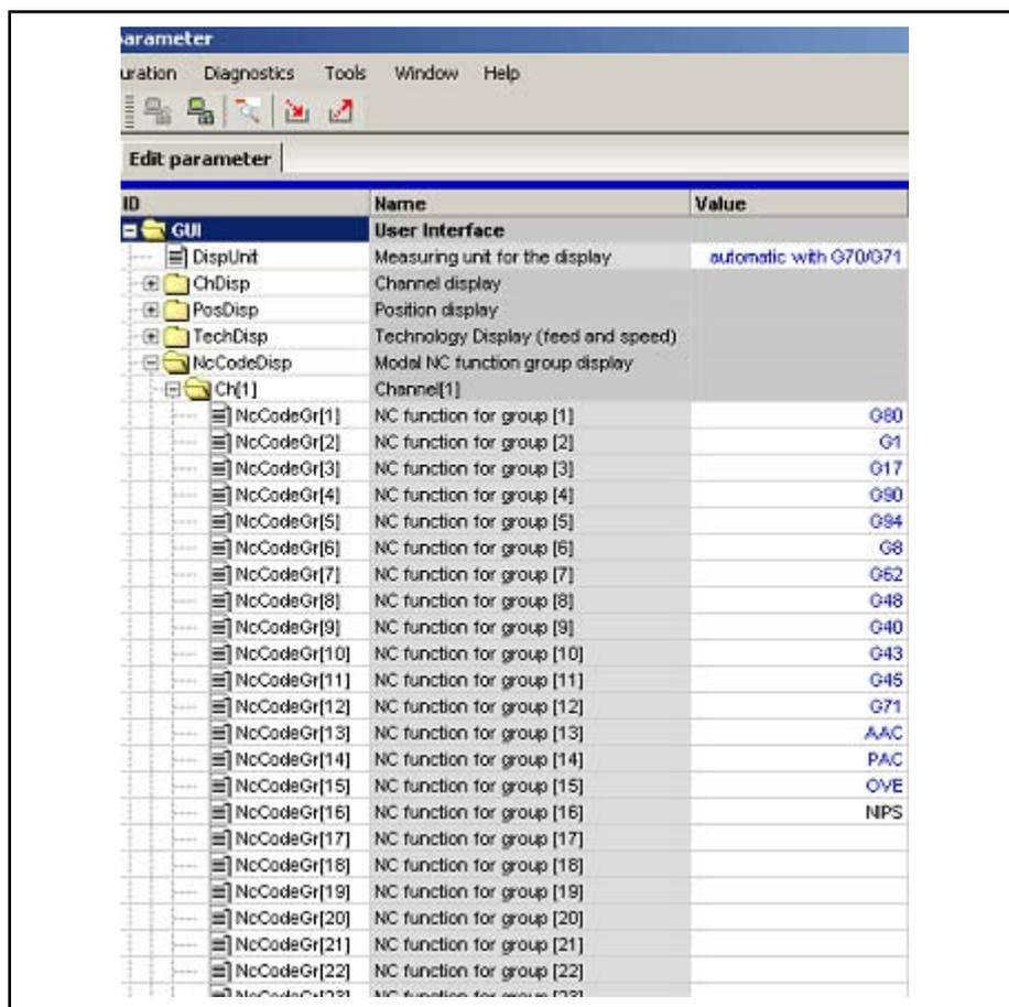
Fig.7-57: Configurator settings for the M-code display
