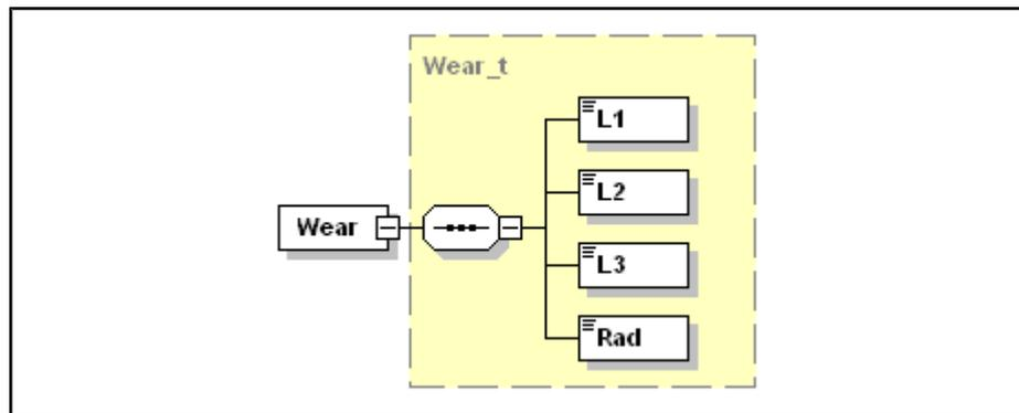
Fig.16-50: Data record schema (12) (wear data upon delivery)
