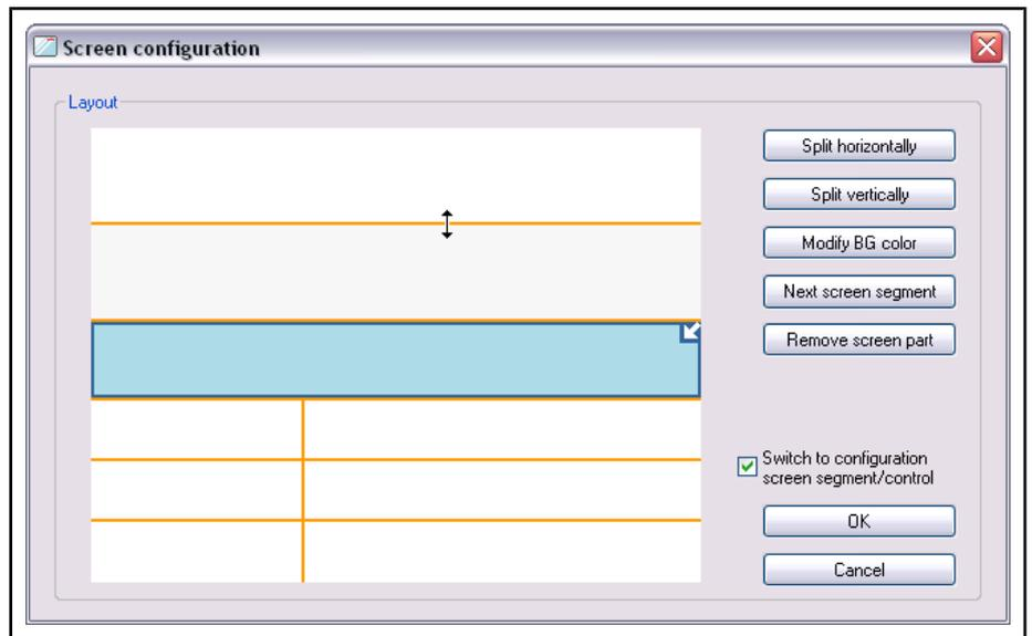
Fig.7-29: Dialog: "Screen configuration" (cursor symbol indicates the possibility for moving the screen segment divider)
