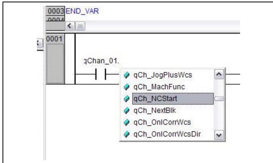
Fig.8-9: Example of using a channel output signal
