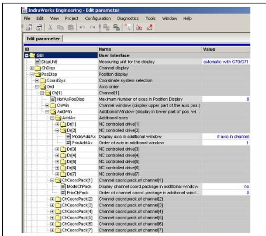
Fig.7-45: Specifying the channel axes to be displayed in the lower portion of the position display
