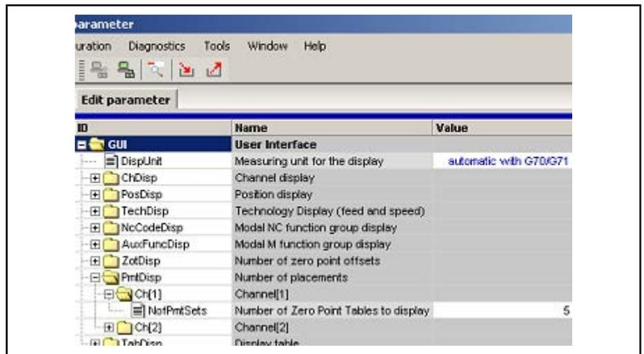
Fig.7-61: Configurator settings for the placements display
