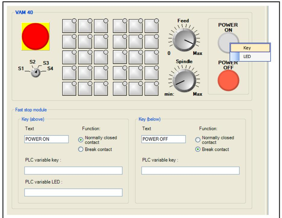
Fig.21-20: Configuration page of the quick-stop module
