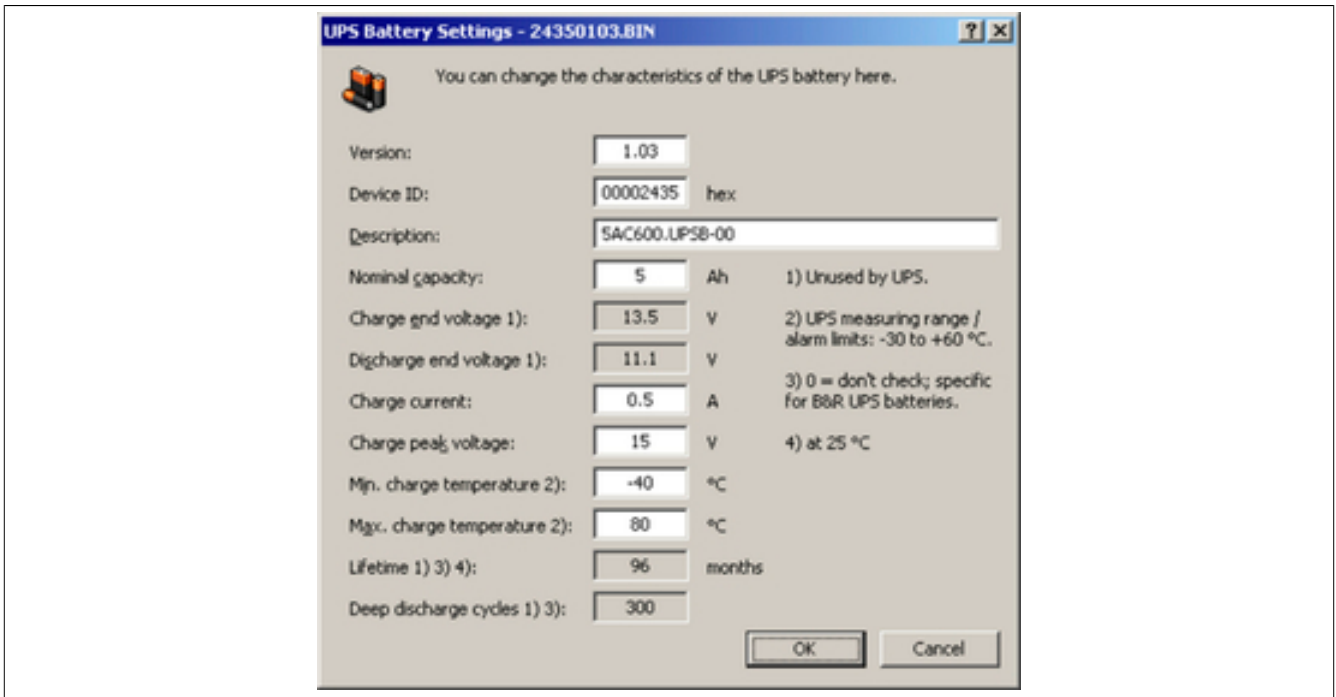
Figure 160: ADI Control Center - UPS battery settings
