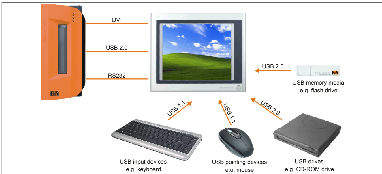
Figure 103: Remote connection of USB peripheral devices on the APC900 via DVI
