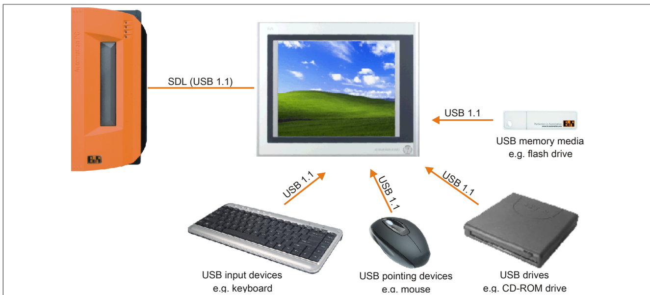
Figure 104: Remote connection of USB peripheral devices on the APC800/900 via SDL
