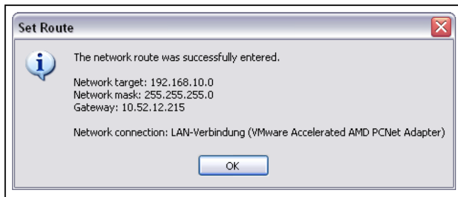
Fig.5-212: "Set Route" was carried out
