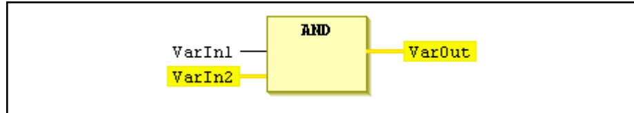
Fig.5-257: Example for a safe data flow: Operator AND with unsafe variable VarIn1, SAFE variables: VarIn2 and VarOut
