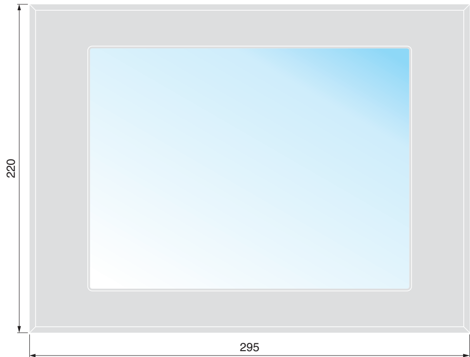
Figure 2-6 Front panel (dimensions in mm)
