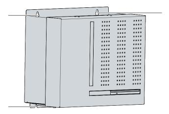
Fig. 25: C6640\_positions fastening screws
