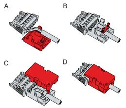
Fig. 21: C6640 Assembly of strain relief housing
