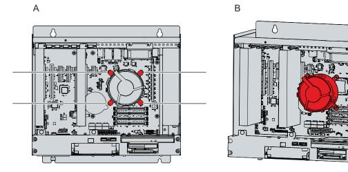
Fig. 34: C6640 exchange CPU cooler
