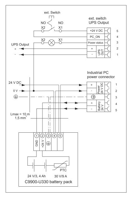
Fig. 19: C6640\_wiring diagram
