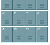
The function of the special keys above the display is also determined by the software. The function is displayed at the top edge of the display. The special keys each have an orange LED controlled by the software.
