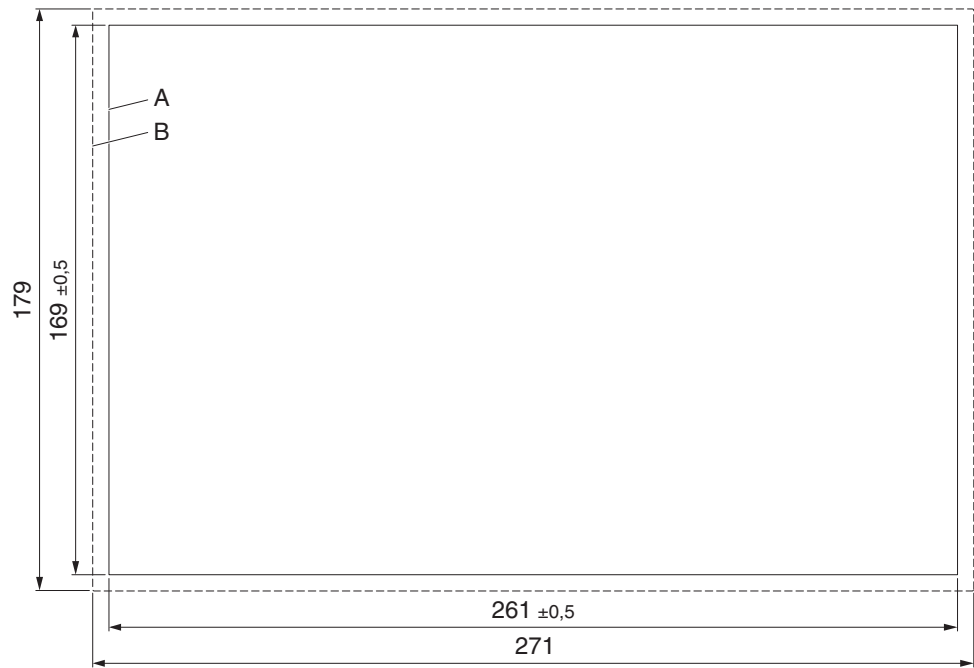
Figure 2-8 Mounting cutout (dimensions in mm)
