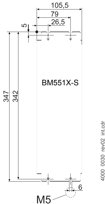
Figure 62: Drilling pattern BM551X
