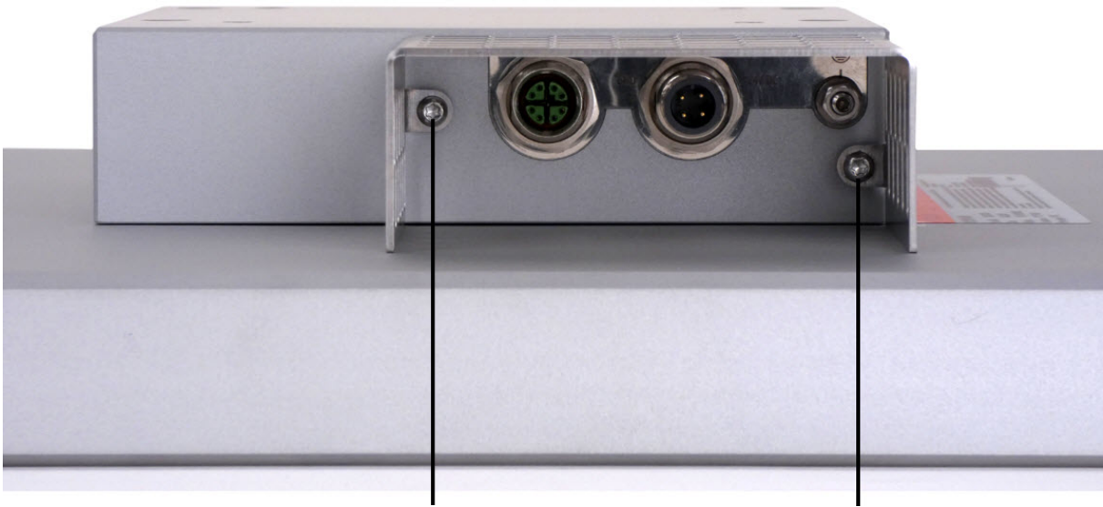
Fig. 3: After removing the two M3 screws with a star screwdriver Torx size 10 the protection cover can be removed.
