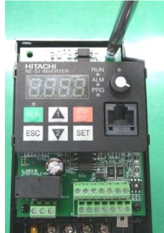
Remove two places of screws.
