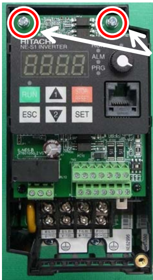
Remove two places of screws.
