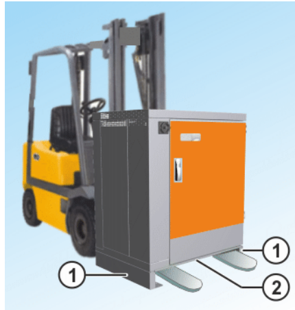
Fig. 7-2: Transportation with standard cabinet base
