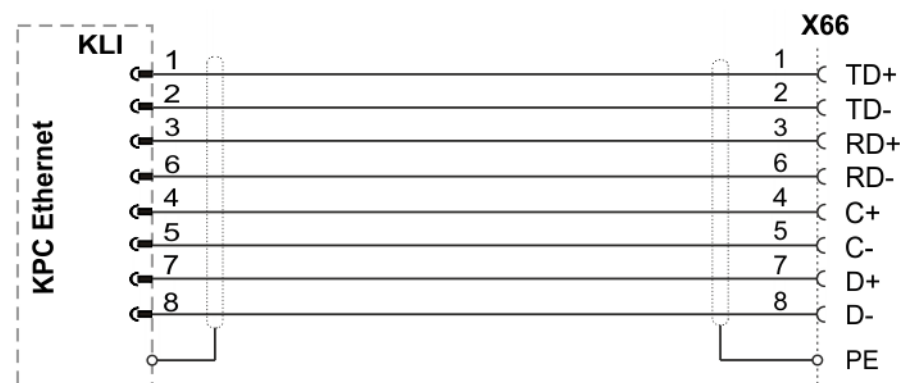
Fig. 6-16: Connector pin allocation X66
