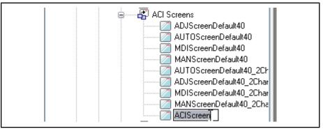
*Fig.7-16: Renaming an ACI screen in the project node*
