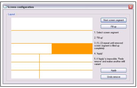
Fig.7-27: Dialog: "Screen configuration" (for filling the deleted screen segment)
