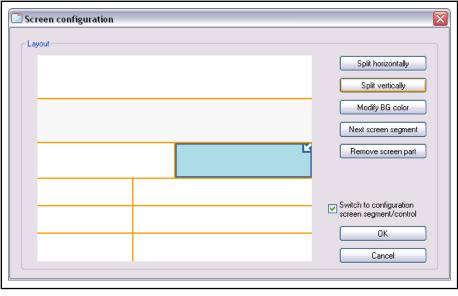
*Fig.7-26: Dialog: Screen configuration (division of the new ACI screen after dividing)*
