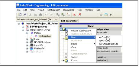
Fig.5-23: Creating an axis parameter structure
