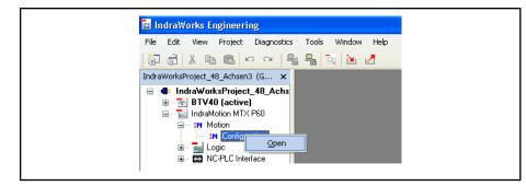
Fig.5-20: Opening the configurator
