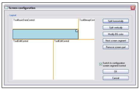
Fig. 16-147: Dialog: Screen configuration (division of the new tool editor after dividing)
