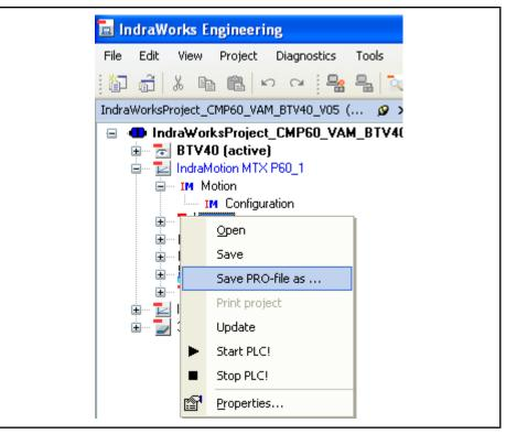
*Fig.12-11:* Context menu: Logic (backing up PLC project)
