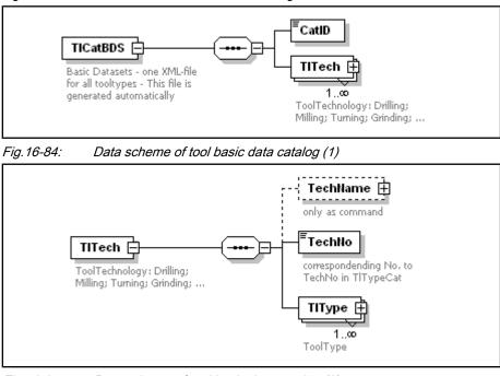
Fig. 16-85: Data scheme of tool basic data catalog (2)
