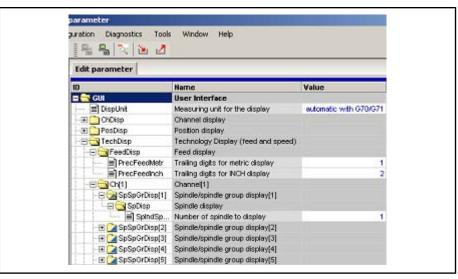
*Fig.7-51:* Settings options for the technology display in the configurator
