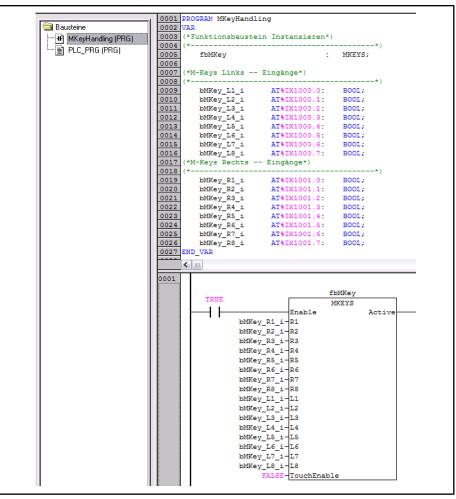
Fig.6-14: Creating a function block for M-keys
