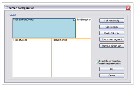
*Fig.16-123:* Dialog: "Screen configuration" (with controls without process connection inserted into screen segments)
