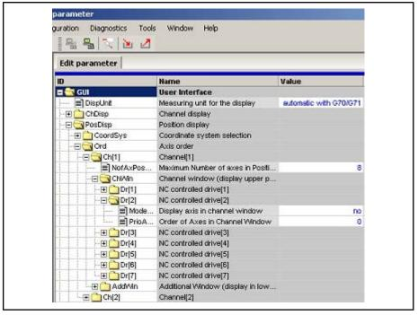
*Fig.7-44:* Specifying the channel axes to be displayed in the upper portion of the position display
