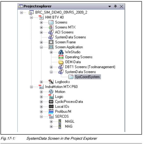
Only one SD variable can be visualized in one system data screen.
