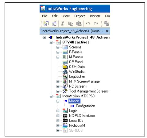
*Fig.4-12:* IndraWorks Engineering (Project Explorer of an IndraWorks project) Before working with the IndraWorks project, it must first be created or an existing saved project must be imported (restored).
