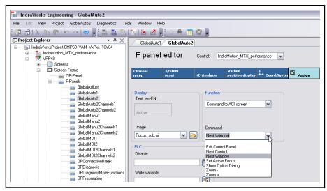
Fig.7-34: F-panel editor: Assign ACI functions to F-keys
