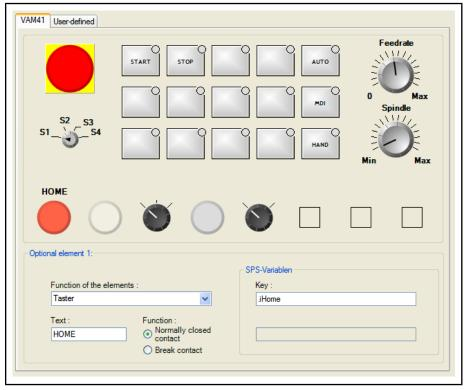
Fig.21-21: Freely configurable elements: VAM 41
