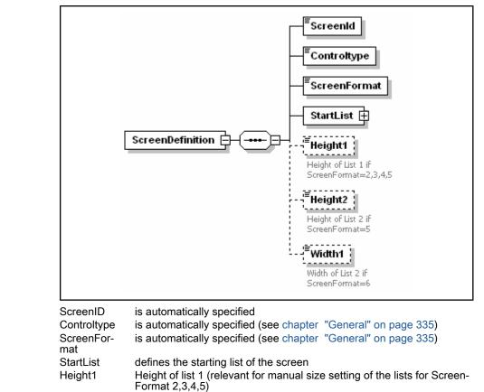
Height 2Height of list 2 (relevant for manual size setting of the lists for Screen-<br/>Format 5)Width 1Width of list 1 (relevant for manual size setting of the lists for Screen-
