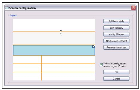
Fig.7-29: Dialog: "Screen configuration" (cursor symbol indicates the possibility for moving the screen segment divider)
