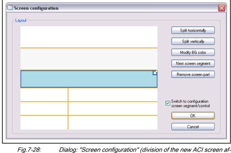
Dialog: "Screen configuration" (division of the new ACI screen after deleting and filling the screen segment)
