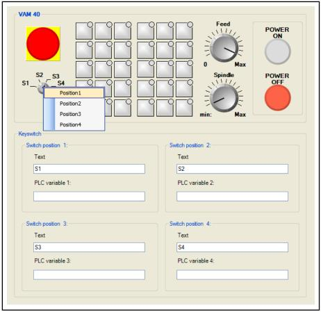
*Fig.21-17: Configuration page of the key-operated switch*
