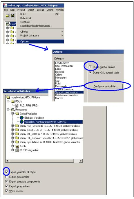
Fig.6-13: Procedure for configuring the symbol file
