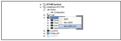
Fig.9-5: Inserting the MSD interface
