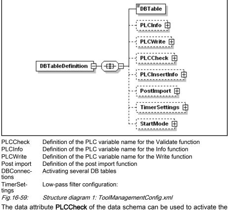
Ine data attribute **PLCCheck** of the data schema can be used to activate the input value check in terms of tool-specific limit value exceedance in the PLC for every data element via the entry"**Lim**".
