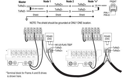
Only pins 4 and 5 on the RJ45 plug should be wired. The other pins on the PowerFlex 4M RJ45 socket contain power, etc. for other Rockwell Automation peripheral devices and must not be connected.
