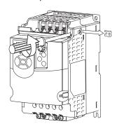
Figure 1.2 Phase to Ground MOV Removal
