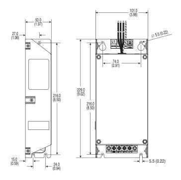
Figure B.7 Frame C EMC Line Filters – Dimensions are in millimeters and (inches) Catalog Number: 22F-RF039-CS, 22F-RF039-CL; 22F-RF026-CS, 22F-RF026-CL
