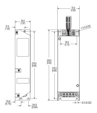
Figure B.6 Frame B EMC Line Filters – Dimensions are in millimeters and (inches) Catalog Numbers: 22F-RF025-BL; 22F-RF021-BS, 22F-RF021-BL; 22F-RF012-BS, 22F-RF012-BL
