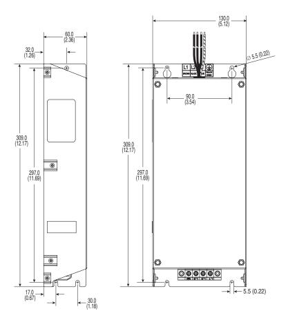
Figure B.8 Remote (Panel Mount) HIM – Dimensions are in millimeters and (inches) Catalog Number: 22-HIM-C2
