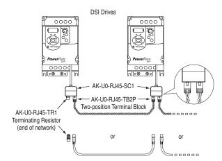
Customer supplied RJ45 male-to-RJ45 male cables with wires connected at pins 4 and 5 only.
