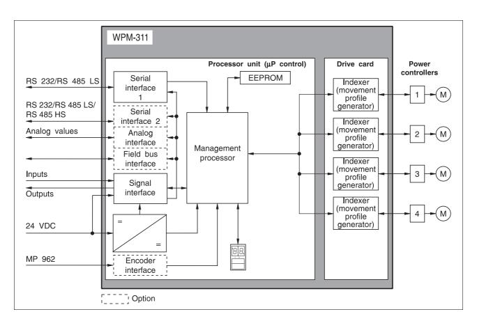
Fig. 1-6 Block diagram
