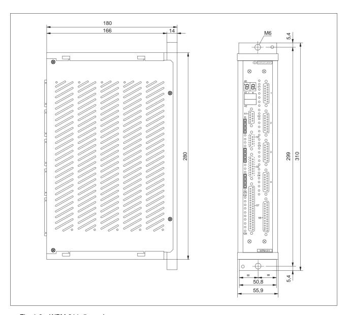
Fig. 1-9 WPM-311 dimensions with 5-phase housing
