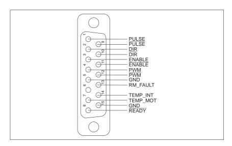
Fig. 2-2 Power controller connection - device end
