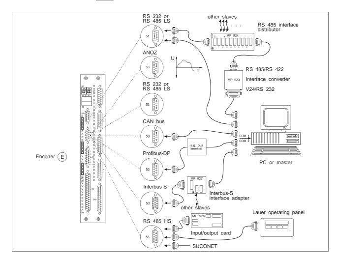
Fig. 1-5 Connection diagram
