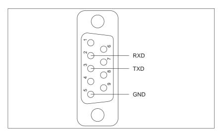
Fig. 2-12 Interface connection - device end
