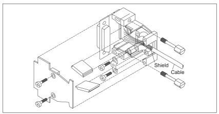
Fig. 2-9 Limit switch connector assembly - device end
