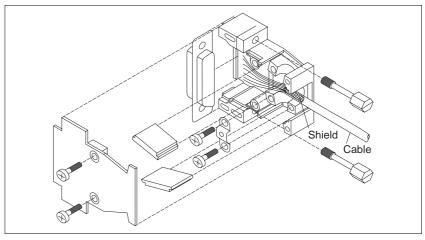
Fig. 2-3 Power controller connector assembly
