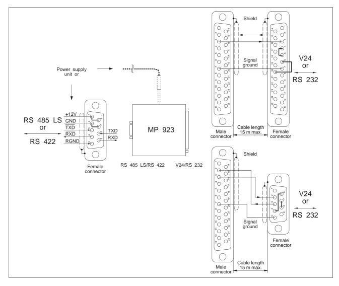
Fig. 6-4 MP 923 interface converter wiring
