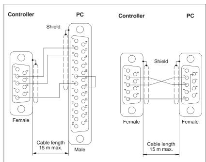
Fig. 2-13 Controller/PC wiring
