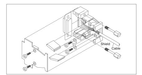
Fig. 2-10 Signal connector assembly - device end
