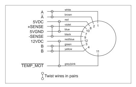
Fig. 2-21 Encoder connector – motor end
