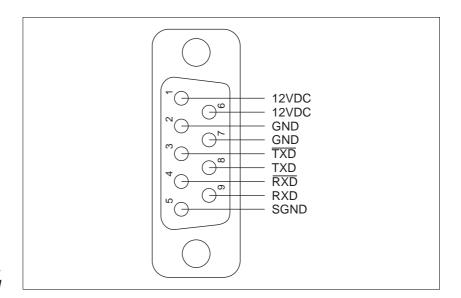
Fig. 2-15 Interface connection - device end
