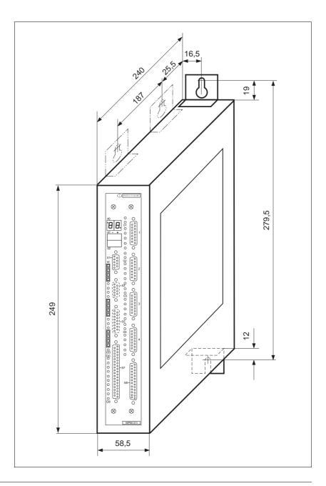
Fig. 1-8 WPM-311 dimensions with 3-phase housing
