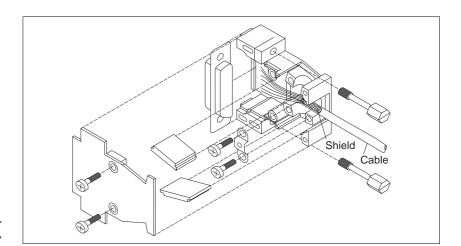
Fig. 2-16 Interface connector assembly
