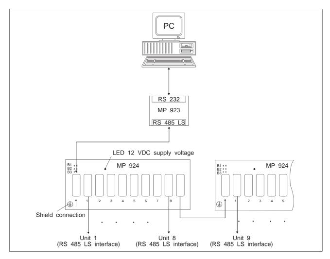
Fig. 6-6 MP 924 interface distributor wiring
