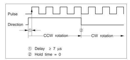
Fig. 2-5 Pulse and direction signals
