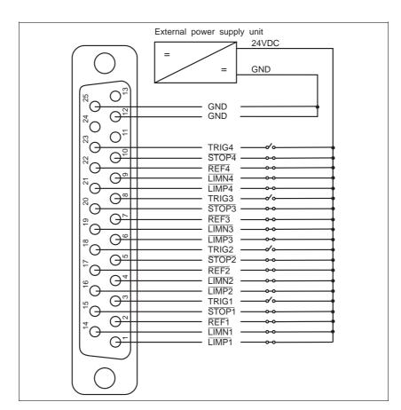
Fig. 2-8 Limit switch connection - device end
