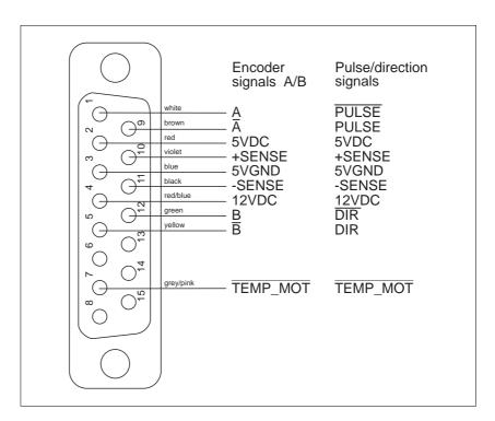
Fig. 2-19 Encoder connector – device end
