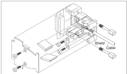
Fig. 2-20 Encoder connector assembly – device end
