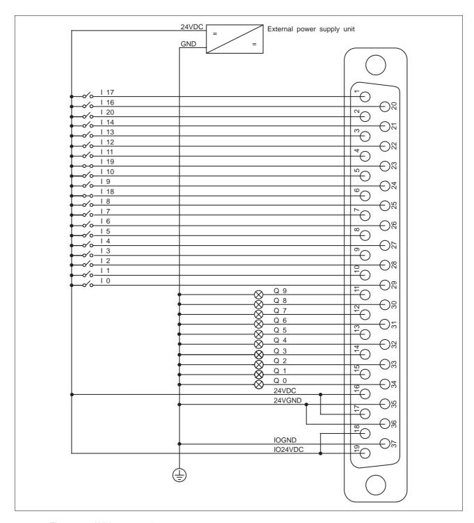
Fig. 2-11 Wiring example
