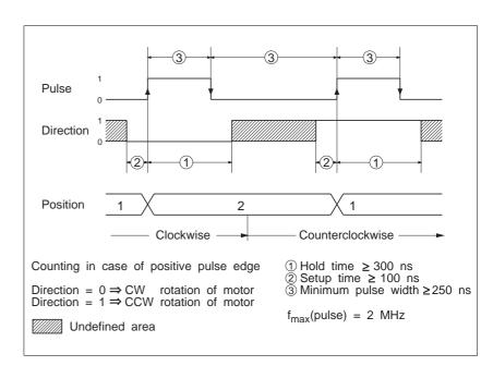
Fig. 2-23 Timing diagram – pulse/direction signals
