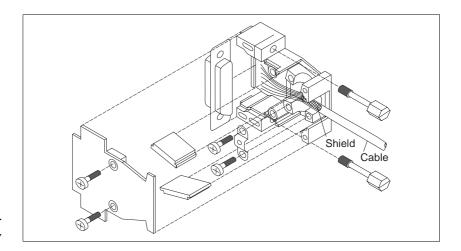
Fig. 2-14 Interface connector assembly
