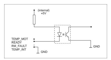
Fig. 2-7 Input circuit principle
