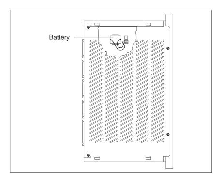
Fig. 5-1 Battery in 5-phase housing of WPM-311
