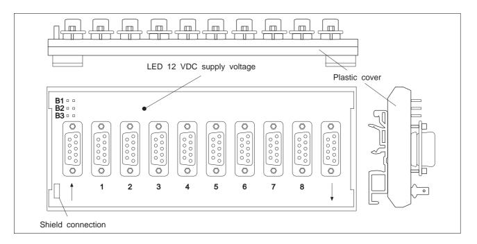
Fig. 6-5 MP 924 interface distributor
