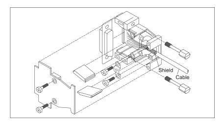
Fig. 2-18 Interface connector assembly
