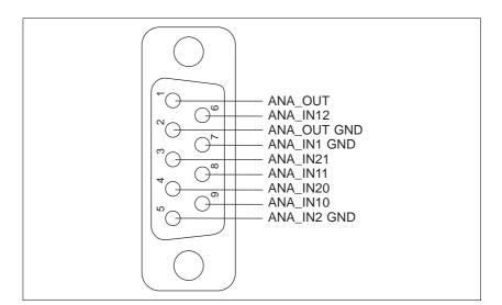
Fig. 2-17 Interface connection - device end
