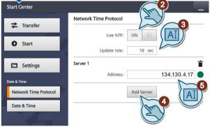
With the **w** button, you remove the corresponding time server from the configuration.
