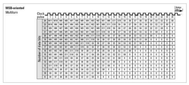
Picture: Arrangement of data bit in the Standard-P-format
