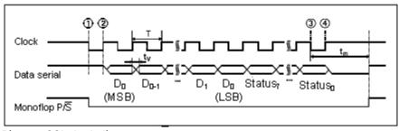
Picture: SSI clock diagram
