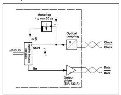
Picture: Block diagram of SSI interface
