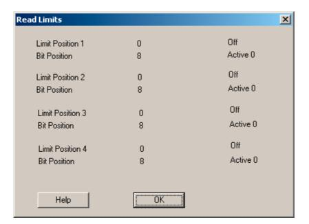
All limit positions (soft limits) are set as 3-byte values. They can be freely adjusted within the value range of the encoder. A status bit is set when the corresponding limit position has been reached. This bit can be output as a status bit at the SSI interface.
