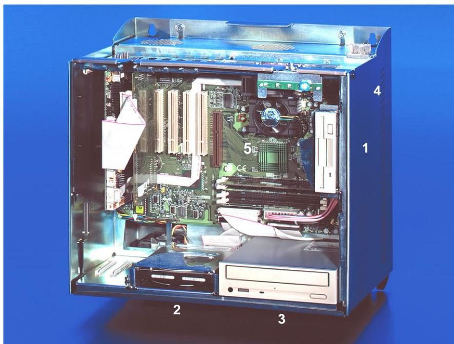
Removing the cover provides access to the floppy drive (1), the 3½ inch hard disk (2), the CD-ROM drive (3), the power supply (4) and the motherboard (5) with processor, memory and plug-in cards. A standard ATX motherboard is used.
