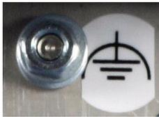
Establish a low-impedance connection from the earthing point on the PC housing to the central earthing point on the control cabinet wall, in which the computer is being installed. The earthing connection is located at the top of the housing (see photograph on the left).
