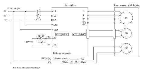
1\*, 2\*: The output terminals allocated with Pn511
