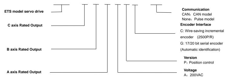
Notes: Each axis of ETS servo drive equips 50W、100W、200W、400W、750W、1.0kW servo motor, and assures three times overload capacity.
