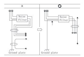
Connect the noise filter ground wire directly to the ground plate. Do not connect the noise filter ground wire to other ground wires.
