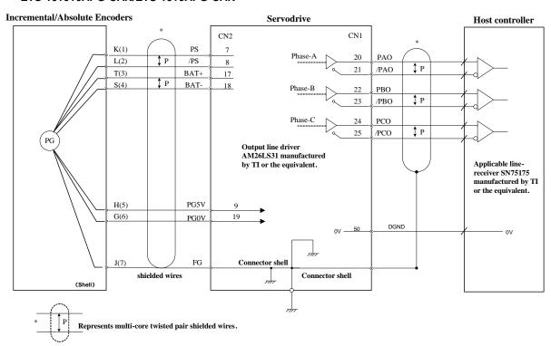
Note: (1)BAT+ and BAT- signals are not used when using an incremental encoder. (2)The pin numbers for the connector wiring differ depending on the servomotors.
