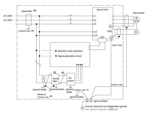
•For ground wires connected to the ground plate, use a thick wire with a thickness of at least 3.5 mm² (preferably, plain stitch cooper wire)
