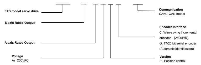
Notes: Each axis of ETS servo drive equips 50W、100W、200W、400W、750W、1.0kW servo motor, and assures three times overload capacity.
