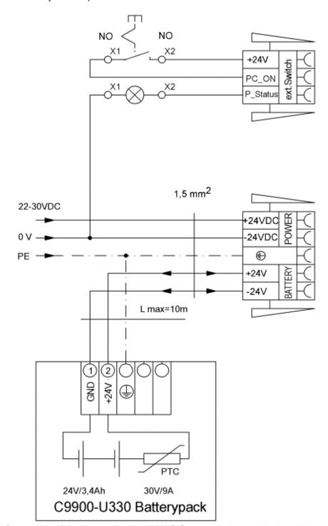
Connection of the Battery Pack and UPS Output only in combination with integrated UPS (order option).
