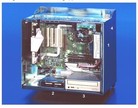
Removing the cover provides access to the floppy drive (1), the 3½ inch hard disk (2), the CD-ROM drive (3), the power supply (4) and the motherboard (5) with processor, memory and plug-in cards. A standard ATX motherboard is used.
