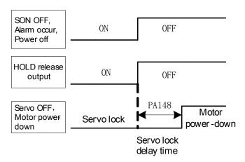
Generally, if HOLD is cut off, simultaneously, the servo drive unit is turned off. When the machinery or worktable slightly moves under the gravity; adjust the PA148 to delay the servo drive unit OFF and then avoid the slight movement.
