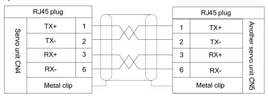
The GSKLink interface of the CNC system is connected by the CN4 or CN5 interface, which carries out the real-time communication with the CNC system. The GR-L series servo unit can be performed by the control, monitoring, administration, debugging and tuning. (Refer to the Section 5.4 for details)
