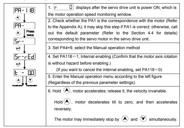
During Manual operation, Sr - r E d displays on the monitoring window, then  $rac{r}{r} - r E d$  shows by OK button, which means the servo drive unit is without enabling signal, set the PA118 as 1; if the  $rac{r}{r} - r E d$  appears on the monitoring window, then displays  $rac{r}{r} - r E d$  by OK button, which means the working method setting of the servo drive unit is incorrect, then set the PA4 as 9.
