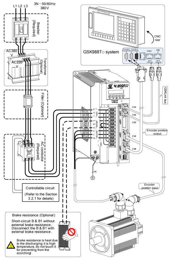
Fig. 3-1 (b) Single peripheral equipment connection of GR2000T-L
