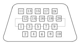
Fig. 3-17 CN3 wiring plug pin figure (Welding cable side)
