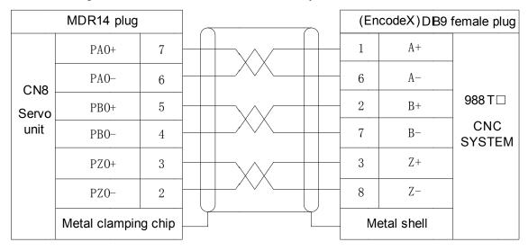
Fig. 3-22 CN8 wiring plug pin (Welding cable side)
