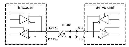
1. The standard wiring of CN2 matches with SJT series permanent synchronous motor absolute encoder.
