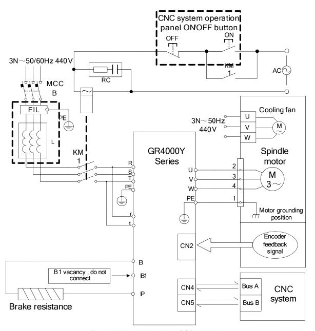
Fig. 3-9 Main circuit wiring of GR4000Y-L
