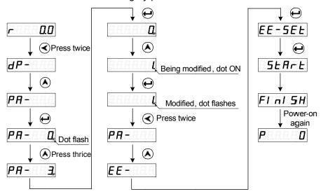
Fig. 4-2 The monitoring operation of the parameter selection state
