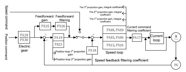
Fig. 6-1 Basis performance parameter debugging
