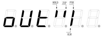
**Explanation:**  $dP - \alpha UE$  monitors the brake releasing signal state via CN7.
