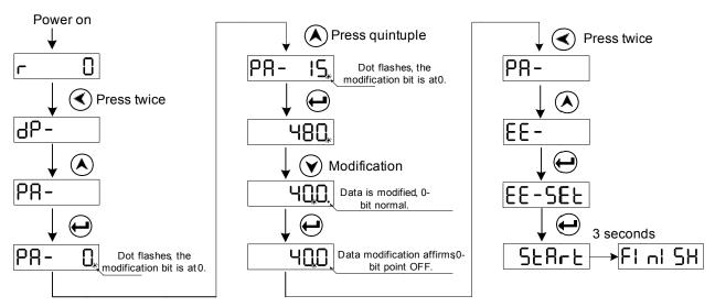
Fig. 4-4 The operation steps for saving the parameter
