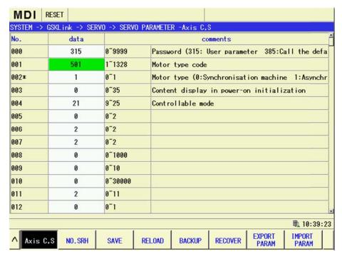
In the above-mentioned interface, enter the "System>GSKLink>Servo>Servo configuration - some one axis" to recover the motor's default parameter operation after the value of the PA1 is
