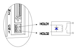
**Notice:** CN1 peripheral loading selection should be less than or equal to the 1.0A/30VDC, 0.3A/60VDC and 0.5A/125VAC!
