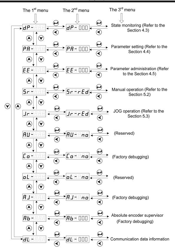
Fig. 4.1 The operation of the display menu
