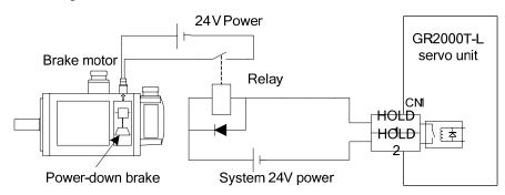
Fig. 6-2 The typical example of the HOLD± brake releasing signal
