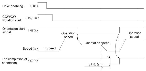
Spindle orientation time-sequence B (The motor is on the free or null velocity state.)
