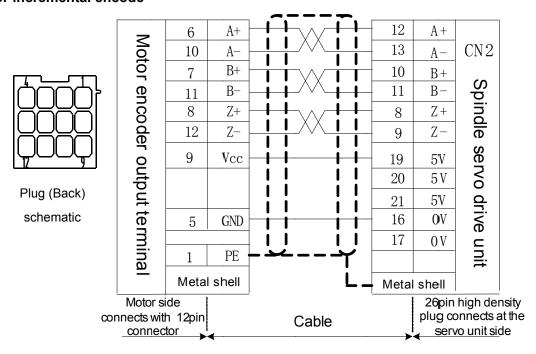
Fig. 3-14 CN2 matching with ZJY182 series spindle motor encoder/12PIN plug wiring
