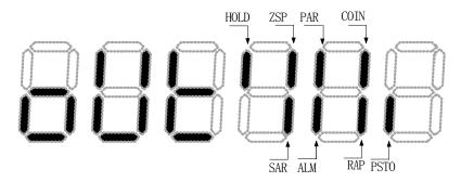
**Explanation:** If the nixie light of the abovementioned figure is ON, the command signal input is enabled; whereas, OFF is disabled.
