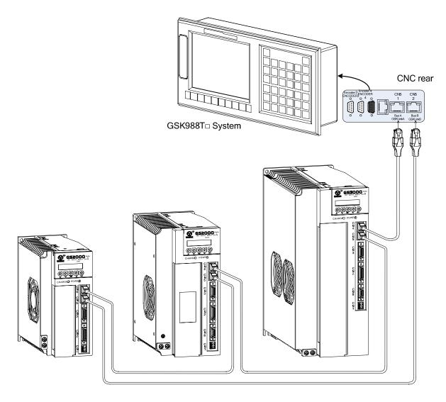
Fig. 3-4 GSKLink bus connection figure for multi servo drive units
