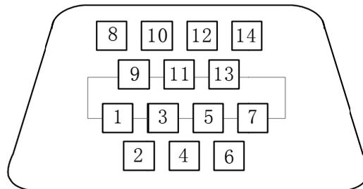
Fig. 3-21 CN8 wiring plug pin (Welding cable side)
