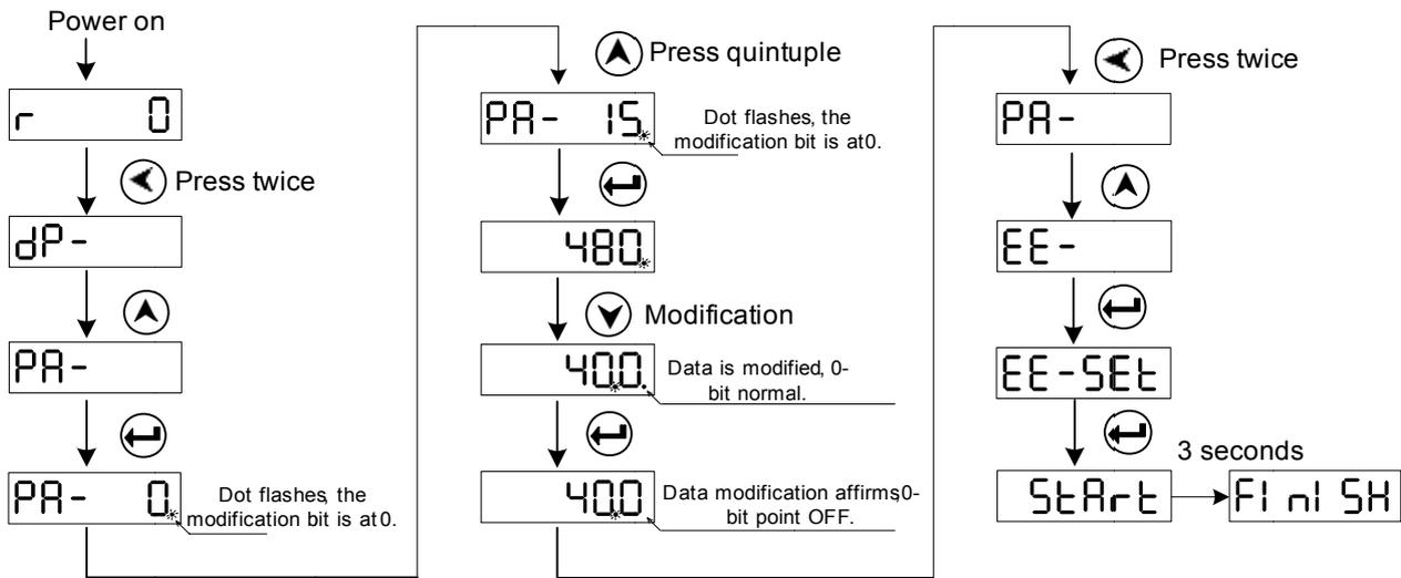
Fig. 4-4 The operation steps for saving the parameter
