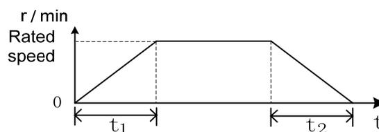
The actual acceleration time of the motor = Command velocity/Rated speed×PA57;
