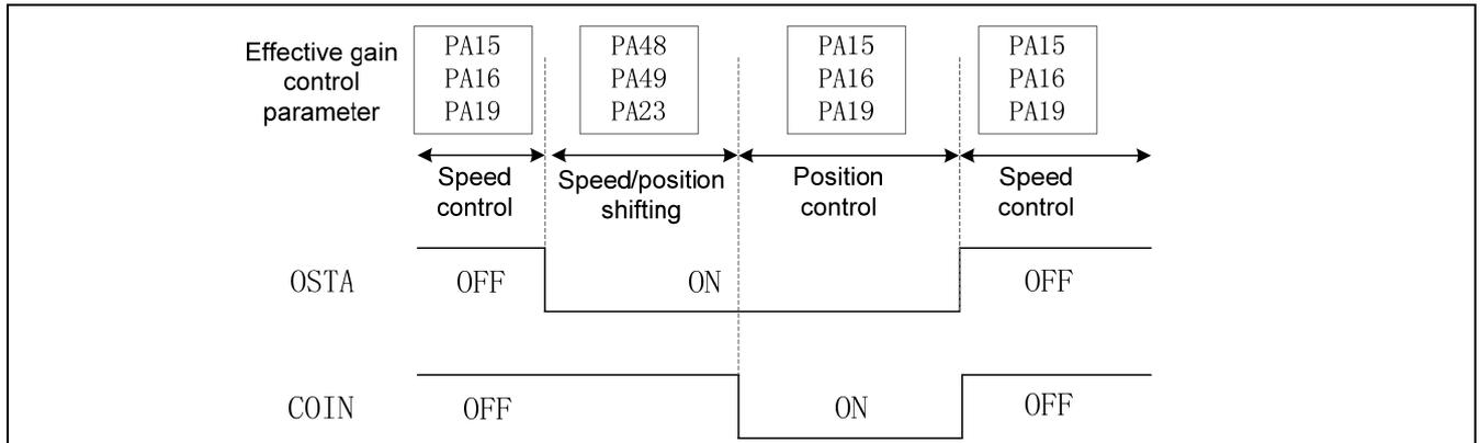
Hence, the spindle swings during orientation, decrease the values of the PA48, PA49 PA23 according to the proportion to remove the swing.
