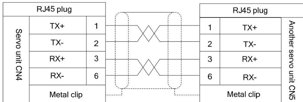
The GSKLink interface of the CNC system is connected by the CN4 or CN5 interface, which carries out the real-time communication with the CNC system. The GR-L series servo unit can be performed by the control, monitoring, administration, debugging and tuning. (Refer to the Section 5.4 for details)
