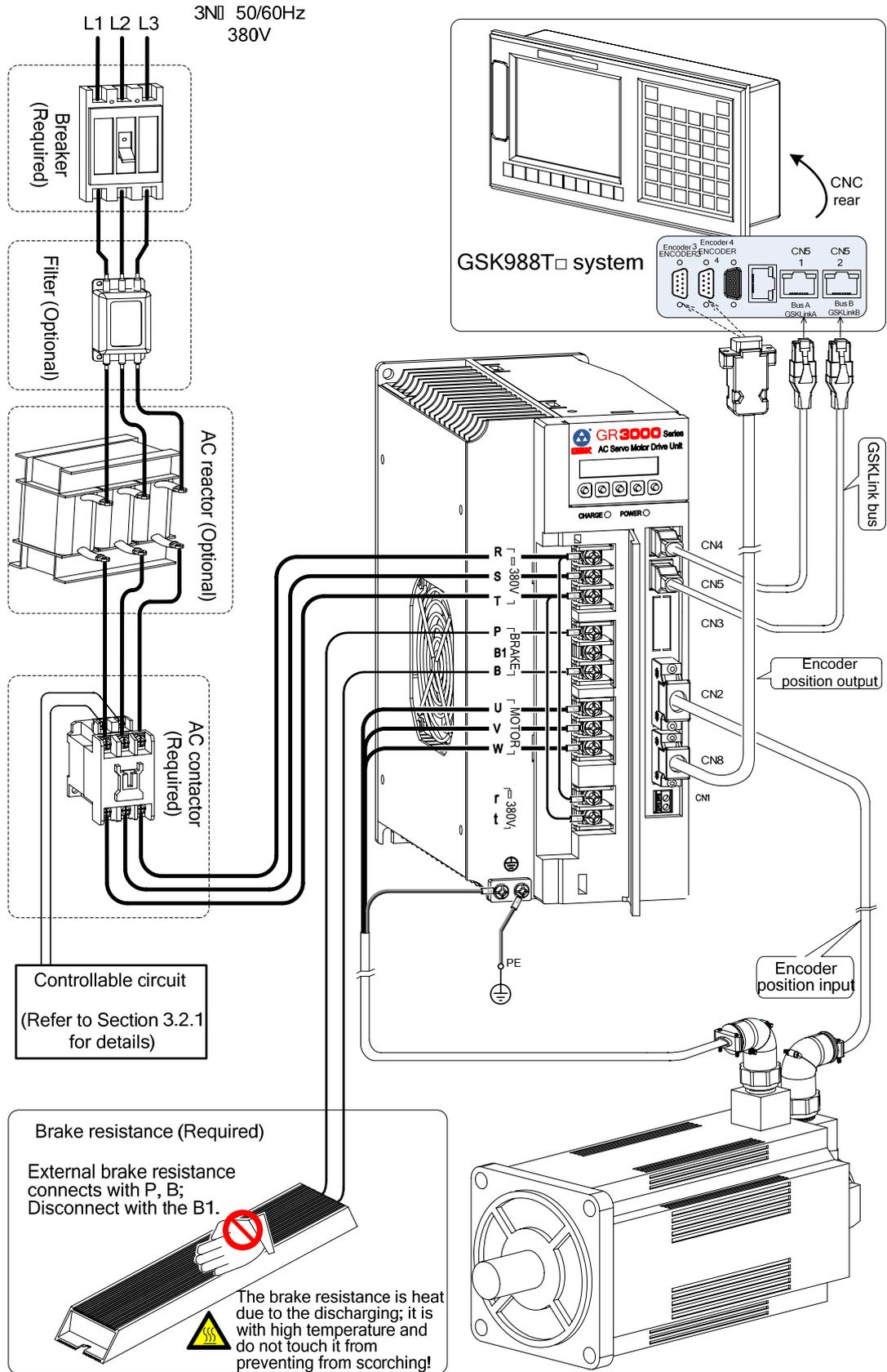
Fig. 3-2 Single peripheral equipment connection of GR3000T-L
