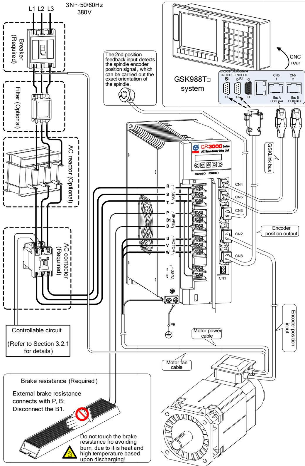
Fig. 3-3 Single spindle servo drive unit peripheral equipment connection of GR3000Y-L
