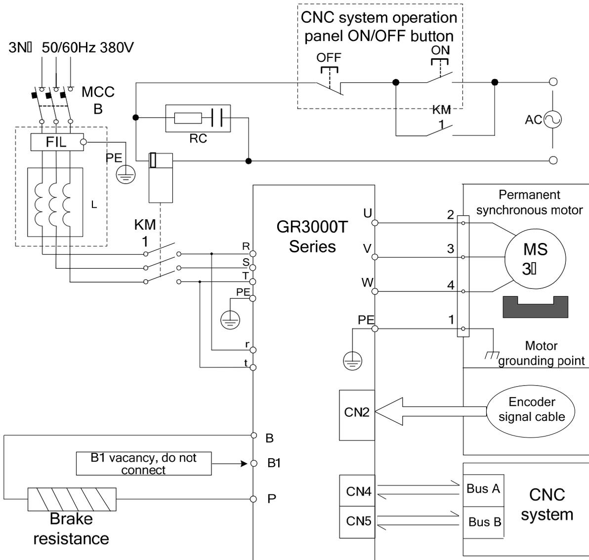
Fig. 3-6 Main circuit wiring of GR3000T-L series
