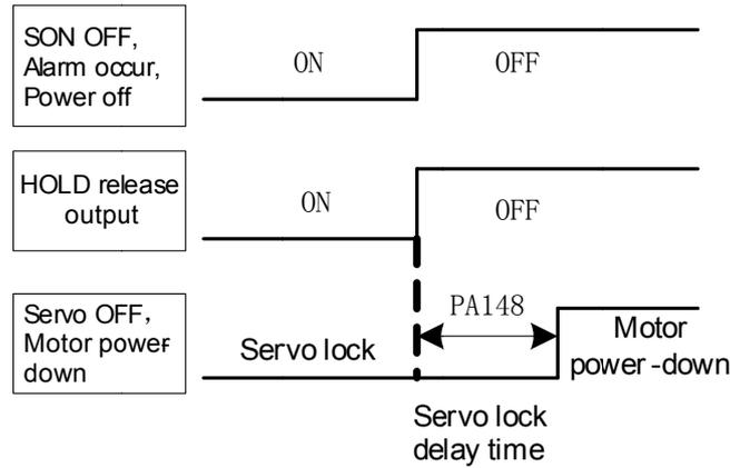
Generally, if HOLD is cut off, simultaneously, the servo drive unit is turned off. When the machinery or worktable slightly moves under the gravity; adjust the PA148 to delay the servo drive unit OFF and then avoid the slight movement.
