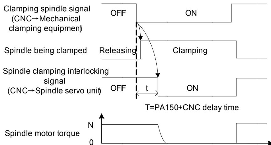
When the workpiece is already machined and spindle clamping equipment releases, the BREF signal is set to OFF. The spindle enters to the position method again and the spindle position is still at the clamping position. The spindle position will slightly offset if the clamping equipment is released; and the spindle position is then drawn back to its clamping position after the BREF turns into OFF.
