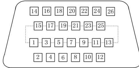
Fig. 3-10 CN2 wiring plug pin (Welding cable side)
