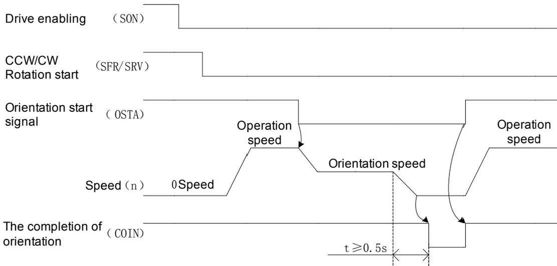
■ Spindle orientation time-sequence B (The motor is on the free or null velocity state.)
