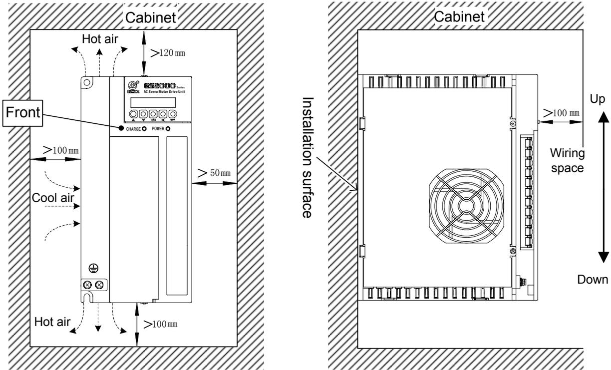
Fig. 2-1 The installation interval for 1 servo drive unit
