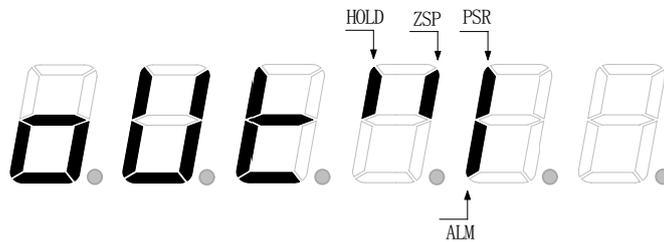
**Explanation:** `dp-out` monitors the brake releasing signal state via CN7.
