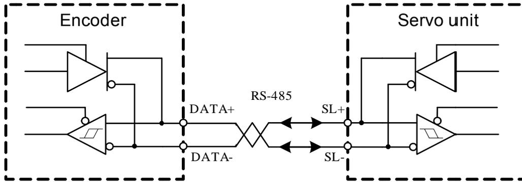
1. The standard wiring of CN2 matches with SJT series permanent synchronous motor absolute encoder.
