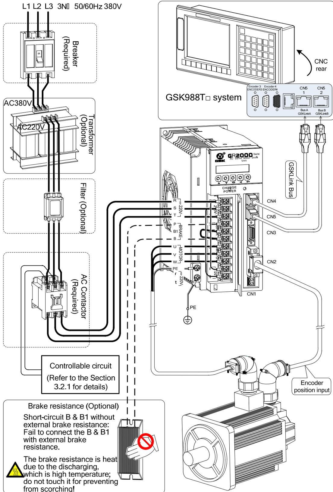
Fig. 3-1 (a) Single peripheral equipment connection of GR2000T-L
