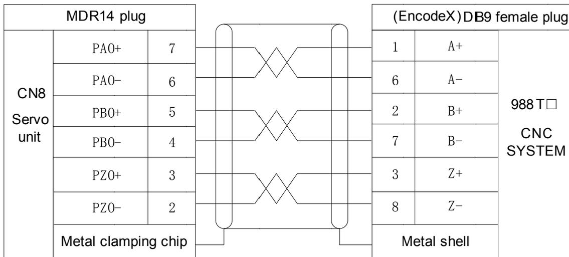
Fig. 3-22 CN8 wiring plug pin (Welding cable side)
