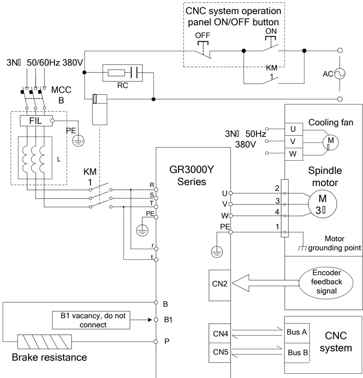
Fig. 3-8 main circuit wiring of GR3000Y-L series
