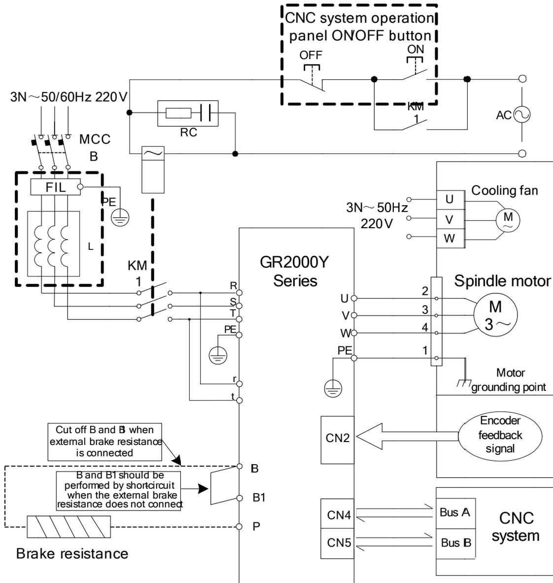
Fig. 3-7 Main circuit wiring of GR2000Y-L series
