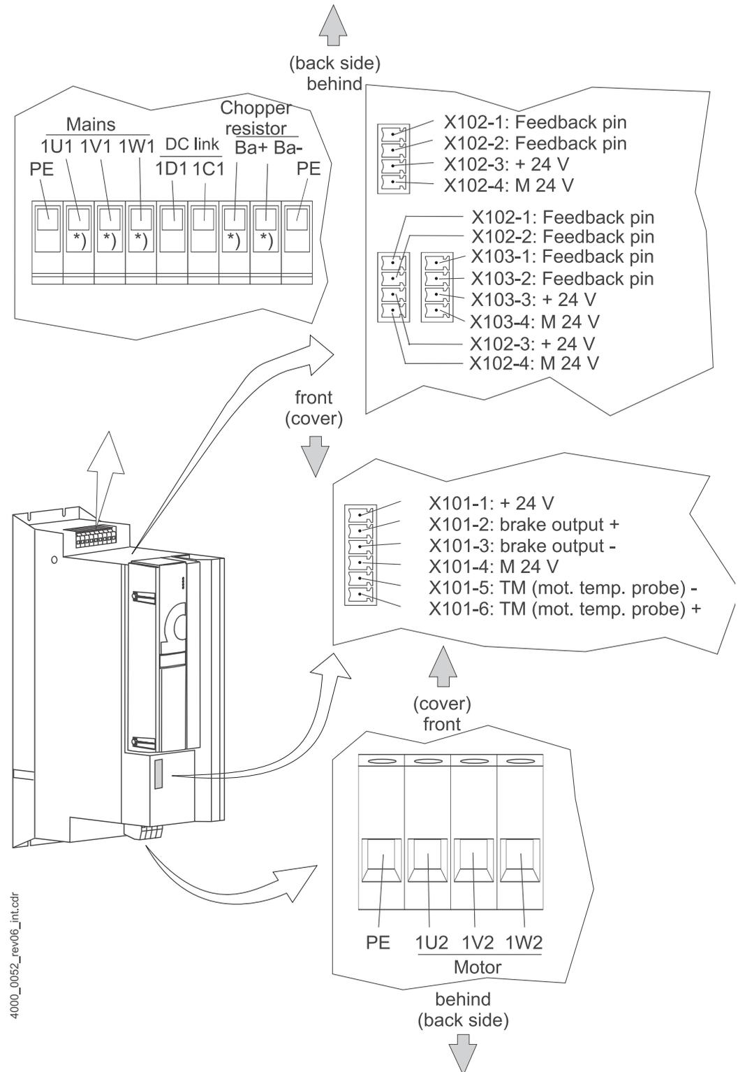
Figure 12: Electrical connections for mains, motor, upon others for BM443X and BM463X
