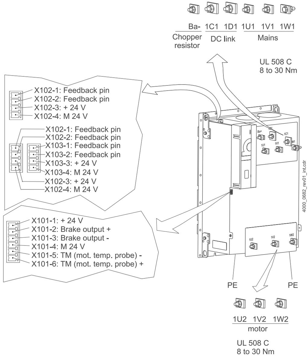
Figure 15: Electrical connections for mains, motor, upon others for BM466X and BM476X
