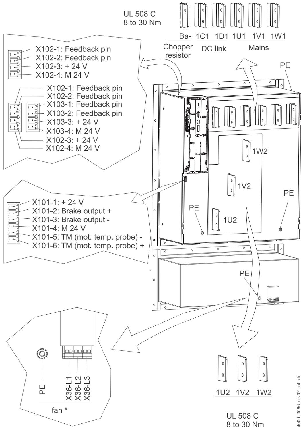
Figure 17: Electrical connections for mains, motor, upon others for BM447X and BM4773
