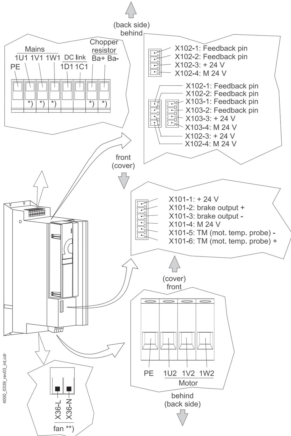
Figure 13: Electrical connections for mains, motor, upon others for BM444X and BM464X
