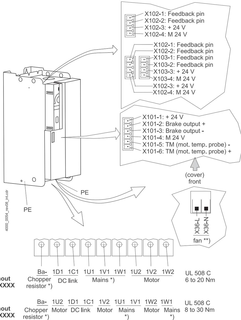
Figure 14: Electrical connections for mains, motor, upon others for BM445X, BM465X, BM446X and BM466X
