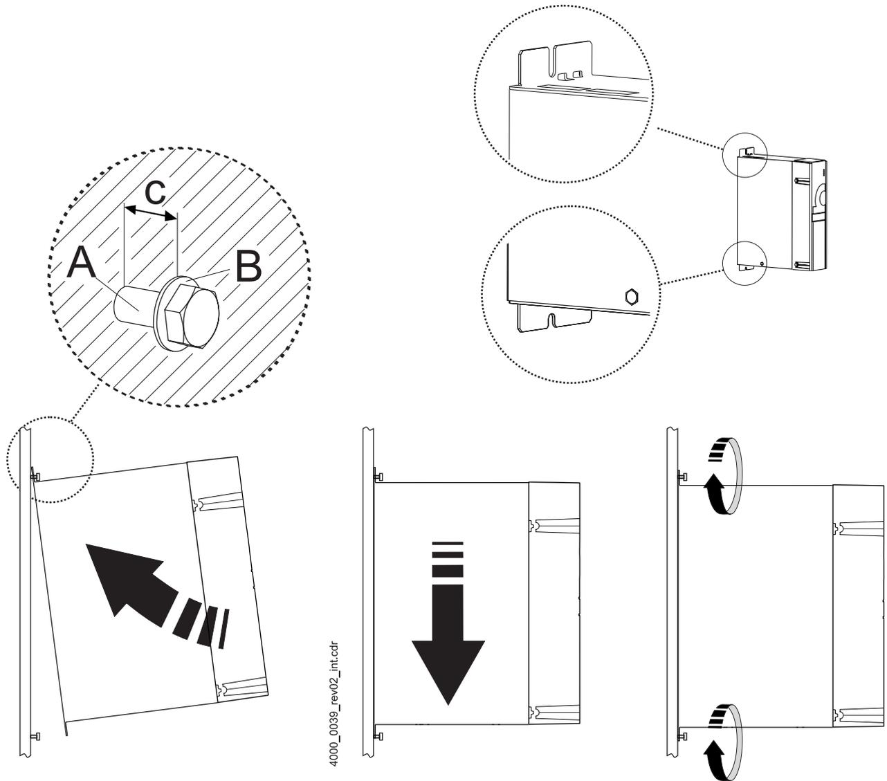
Figure 2: Mounting instruction BM441X, BM442X-S, BM443X-S/Z, BM463X-S/Z, BM444X-S/Z, BM464X-S/Z
