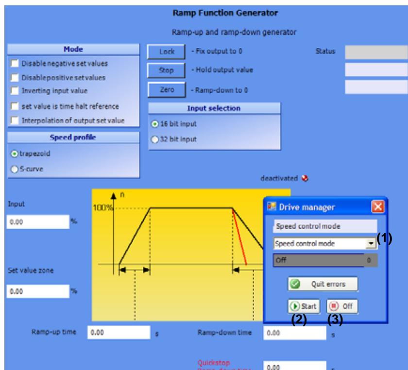
Figure 42: ProDrive: Ramp function generator - Drive manager
