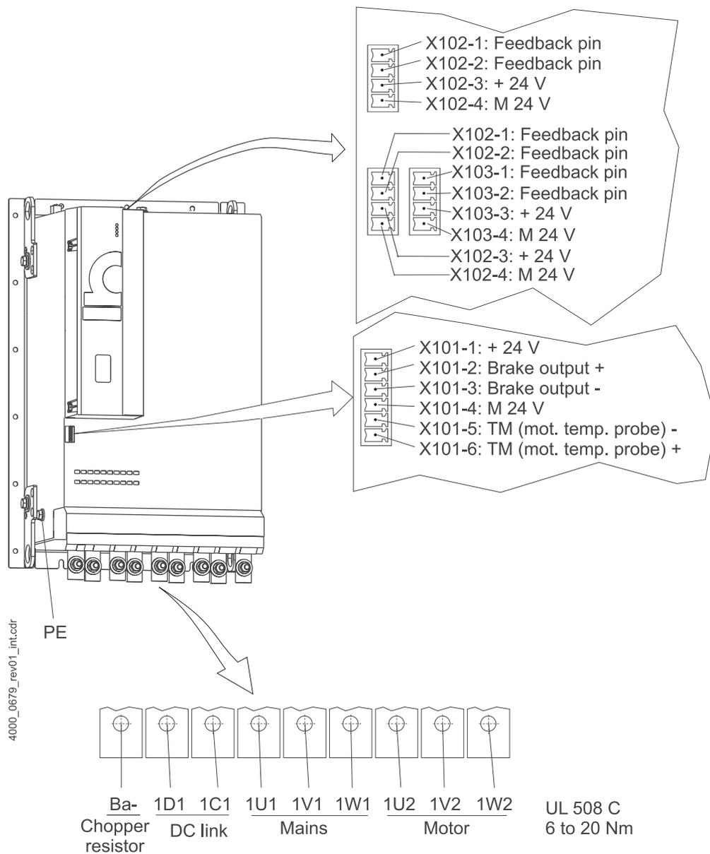
Figure 16: Electrical connections for mains, motor, upon others for BM4755
