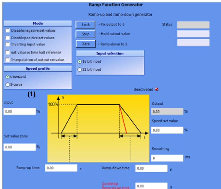
Figure 40: ProDrive: Ramp function generator
