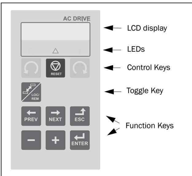
Fig. 42 Control panel display, LEDs and Keys.
