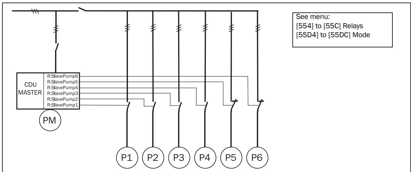
Fig. 35 Example of "Fail safe" operation
