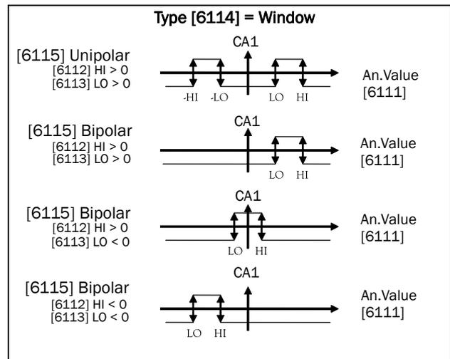
Fig. 98 Principle functionality of comparator features for "Type [6114] = Window" and "Polar [6115]".
