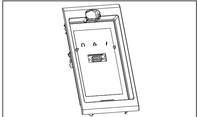
Fig. 52 RS232 connector behind the HCP control panel (Optional)
