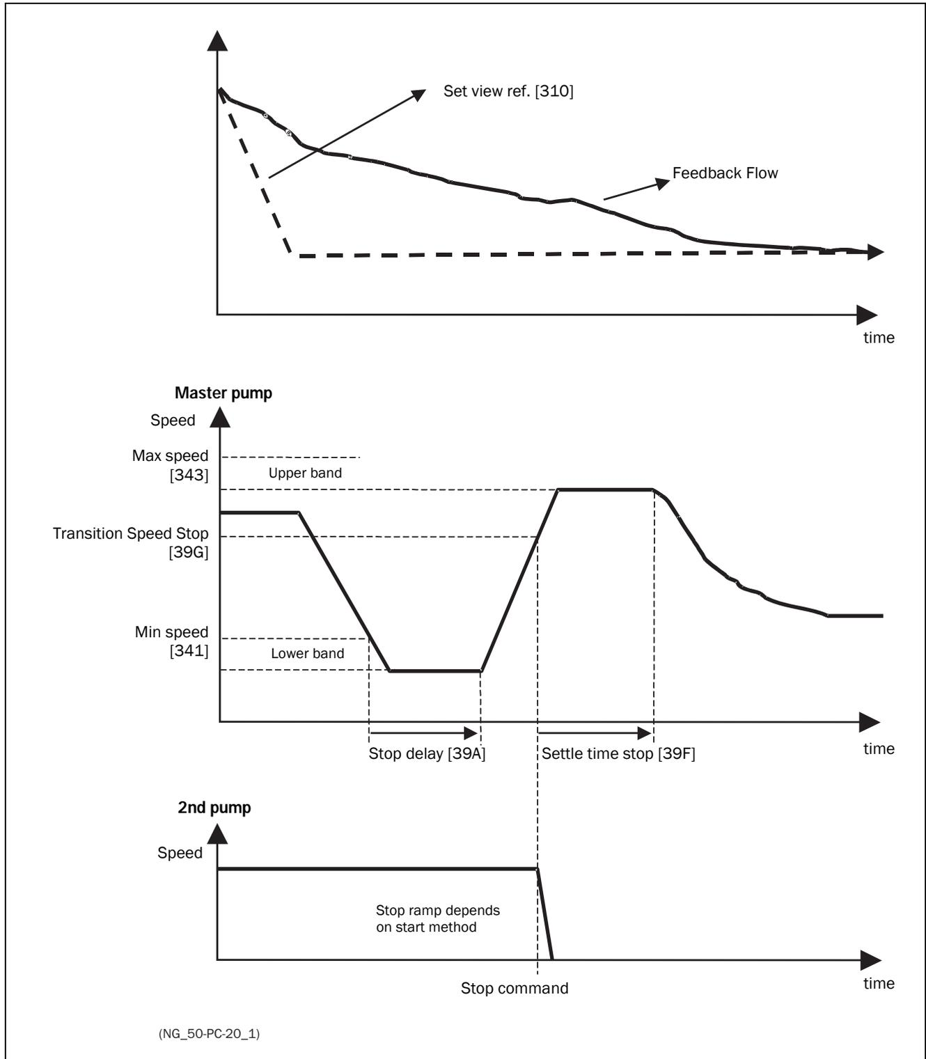
Fig. 38 Time sequence stopping an additional pump
