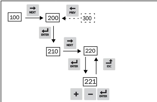
Fig. 22 Example of menu navigation when entering motor voltage
