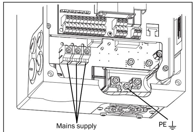
Fig. 10 Mains connections, CDU 008-018 with side cable entry/outlet.
