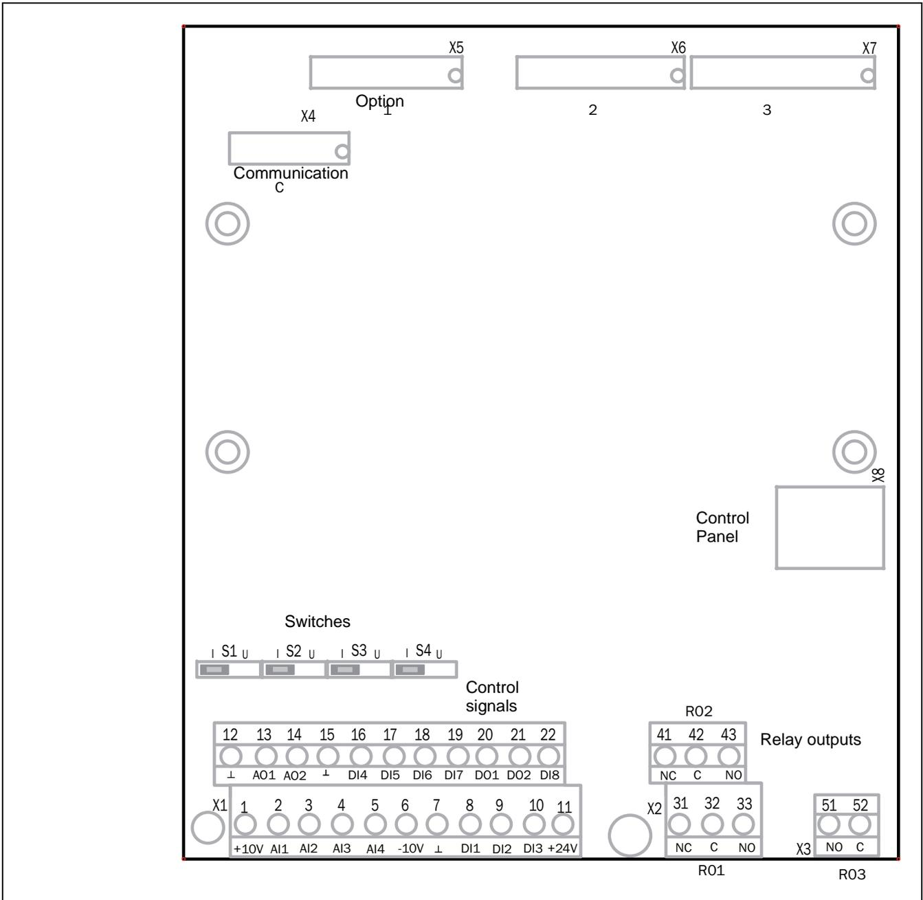
Fig. 16 Control board layout
