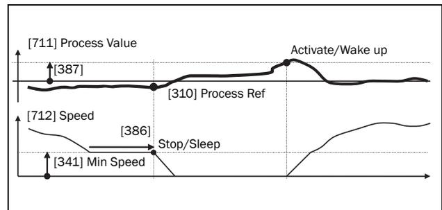
Fig. 75 PID Stop/sleep with inverted PID
