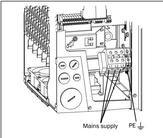
Fig. 12 Mains connections, CDU 026-046 with side cable entry/outlet.
