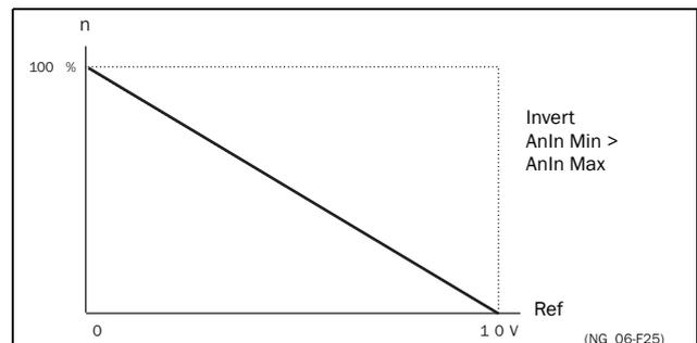
Fig. 90 Inverted reference
