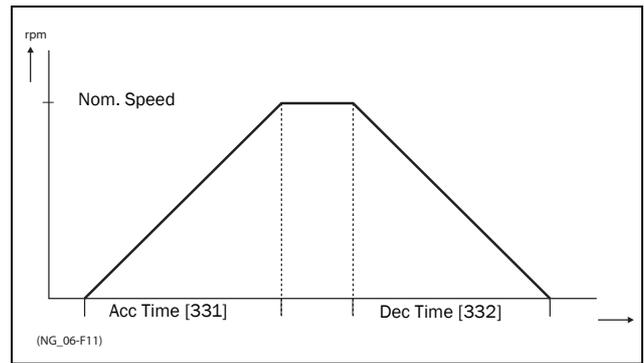
Fig. 61 Acceleration and deceleration times
