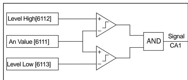
Fig. 94 Analogue comparator type "Window"
