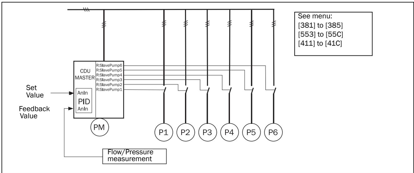
Fig. 36 PID control
