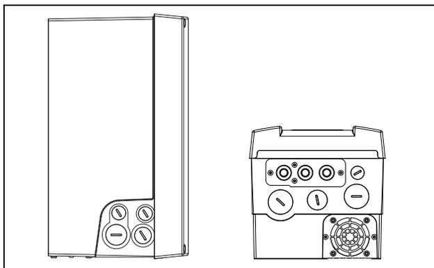
Fig. 3 CDU 48/52 Model 008 to 018, frame size B with cable inlet from long side (standard) or short side.
