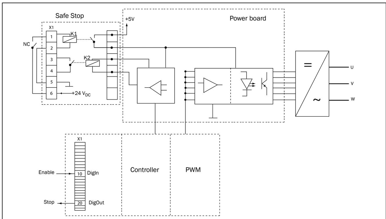
Fig. 115 Safe Stop connection
