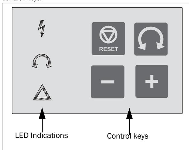
Fig. 40 LED indication and control keys.
