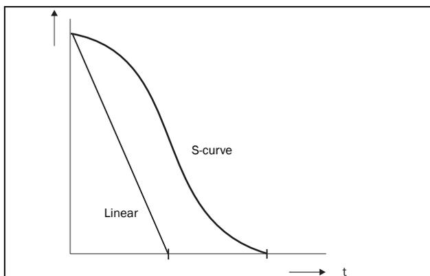
Fig. 64 Shape of deceleration ramp
