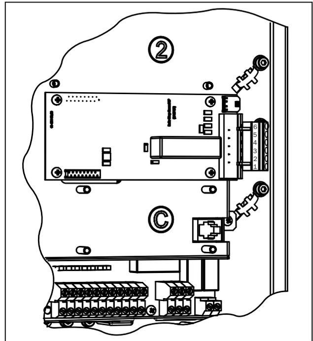
Fig. 113 Connection of safe stop option in size B.
