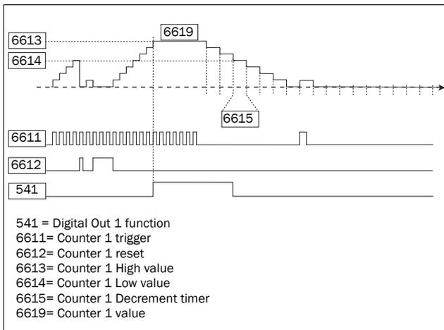
Fig. 102 Counters, operating principle.
