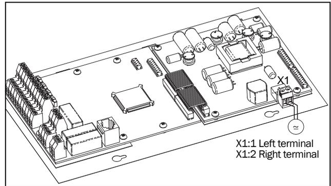
Fig. 112 Connection of standby supply option .
