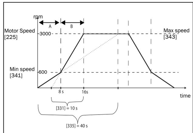
Fig. 62 Calculation example of accelerating times (graphics not proportional).
