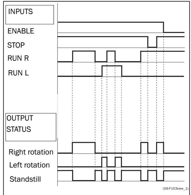
Fig. 26 Input and output status for level-control
