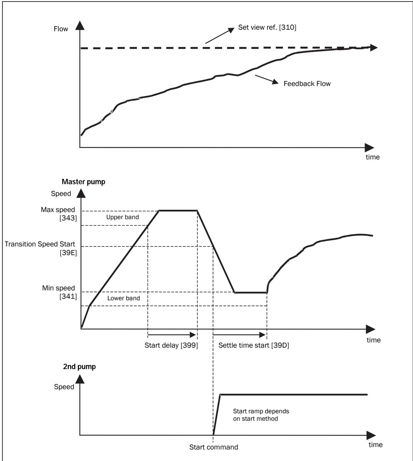
Fig. 37 Time sequence starting an additional pump
