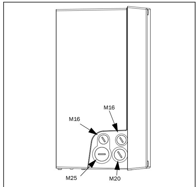
Fig. 6 CDU 48/52: Model 008 to 018 (B) with side cable entry/outlets.
