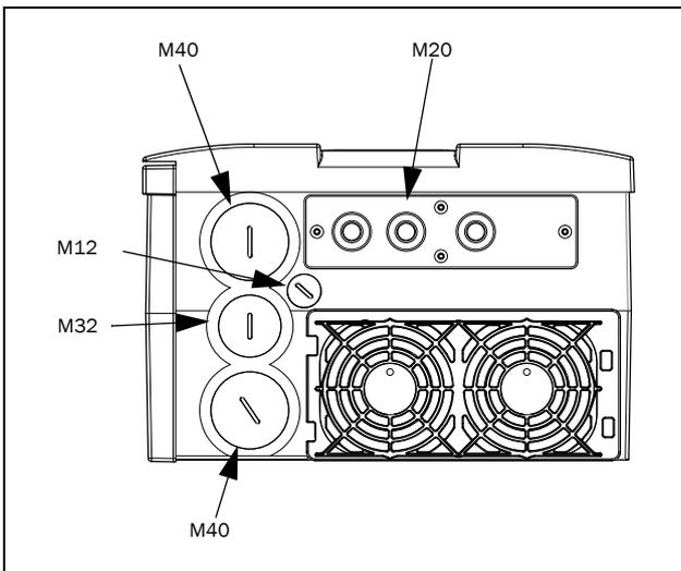
Fig. 9 CDU 48/52: Model 026 to 046 (C), with cable entry/outlets on short side
