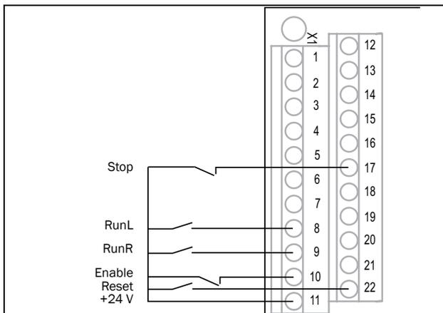
Fig. 25 Example of wiring for Run/Stop/Enable/Reset inputs
