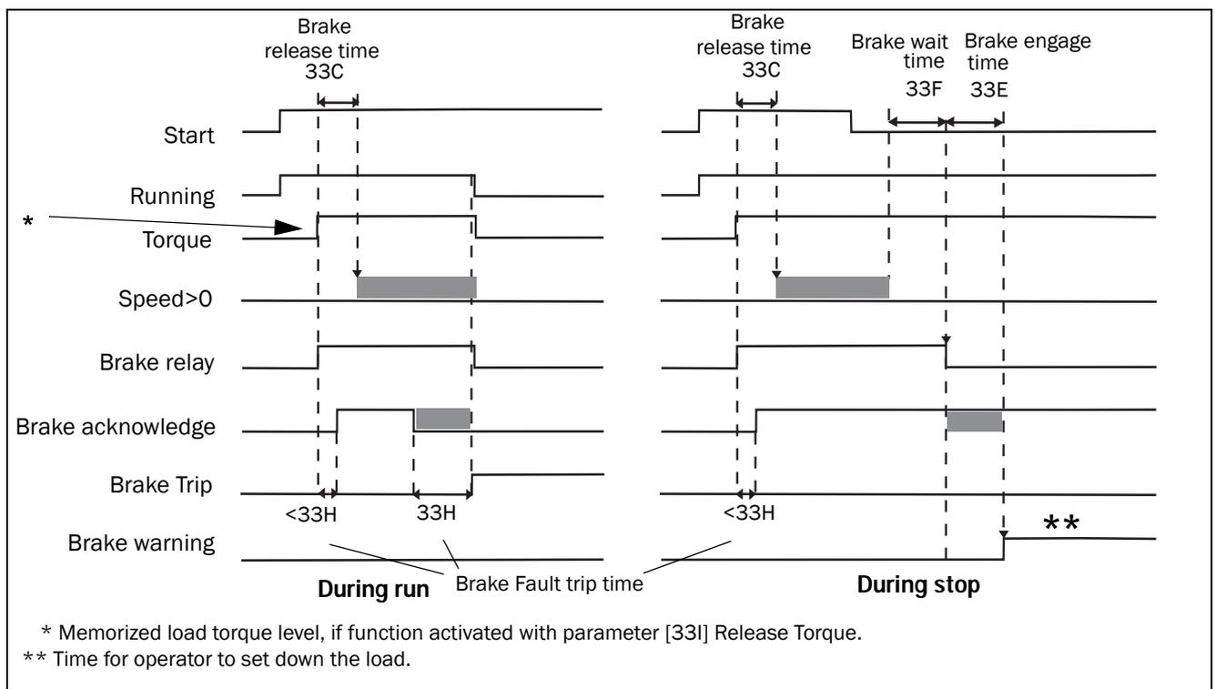
Fig. 66 Principle of Brake operation for fault during run and during stop
