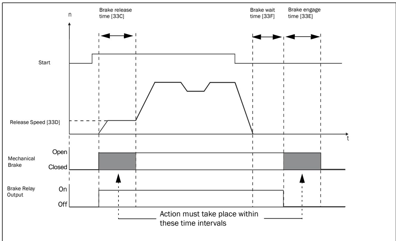
Fig. 65 Brake Output functions
