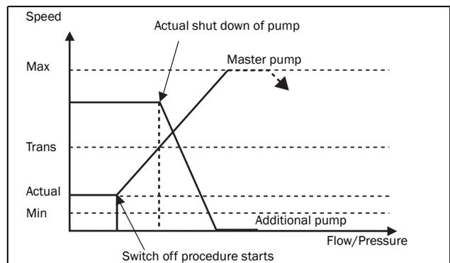
Fig. 83 Transition speed stop
