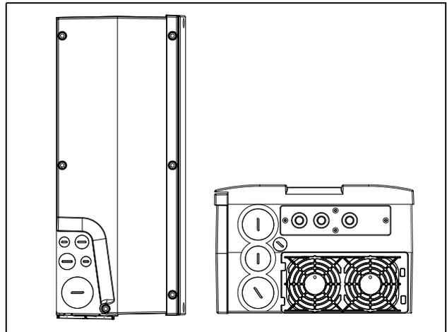
Fig. 4 CDU 48/52 Model 026 to 046, frame size C with cable inlet from long side (standard) or short side
