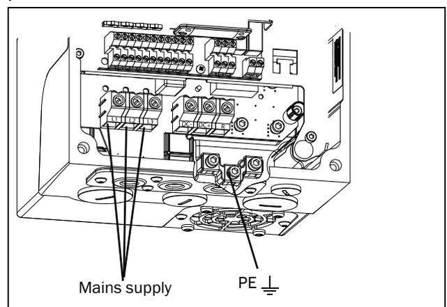
Fig. 11 Mains connections, CDU 008-018 with cable entry/outlet on short side.
