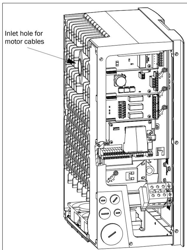
Fig. 15 Inlet for motor cables
