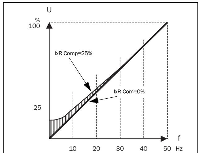
Fig. 70 IxR Comp at Linear V/Hz curve
