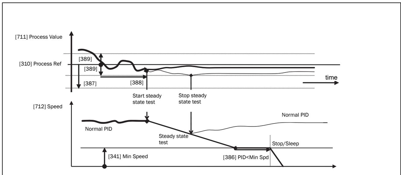
Fig. 76 Steady state test
