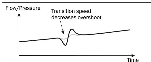
Fig. 82 Effect of transition speed
