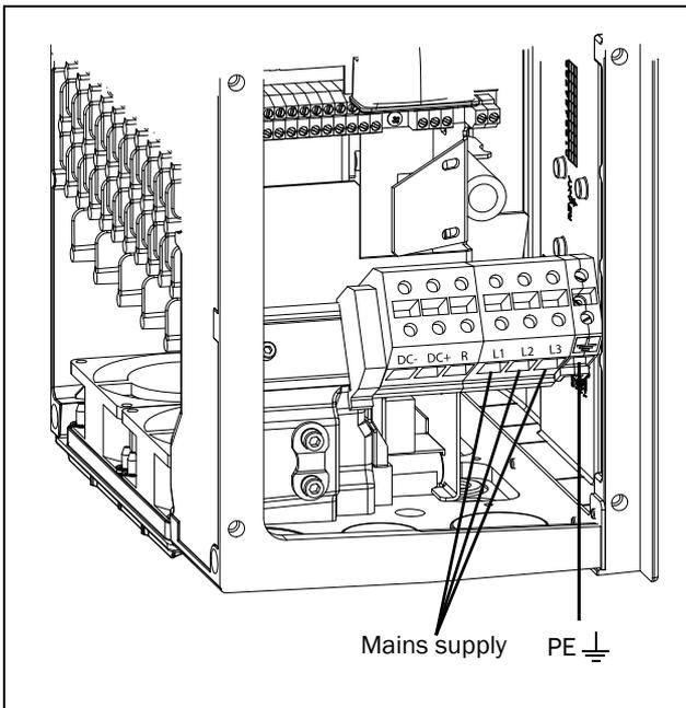
Fig. 13 Mains connections, CDU 026-046, with cable entry/outlet on short side.
