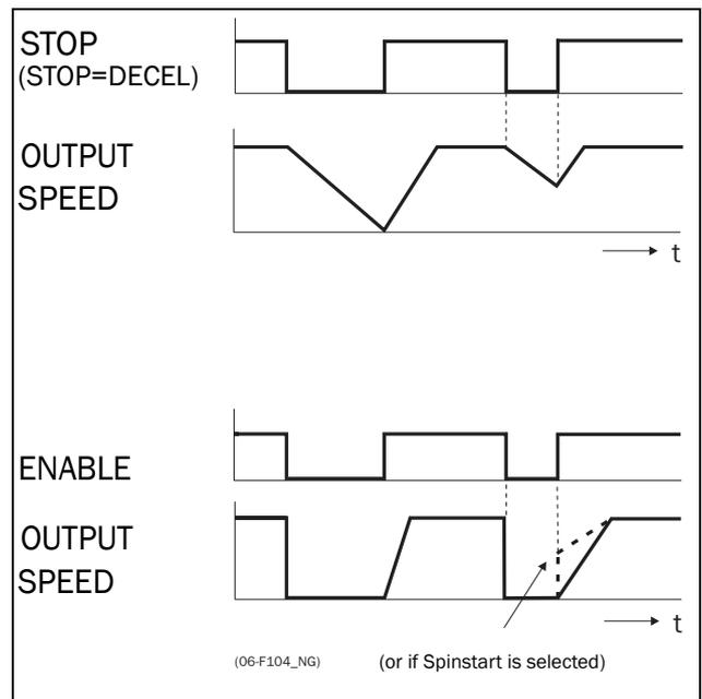
Fig. 24 Functionality of the Stop and Enable input
