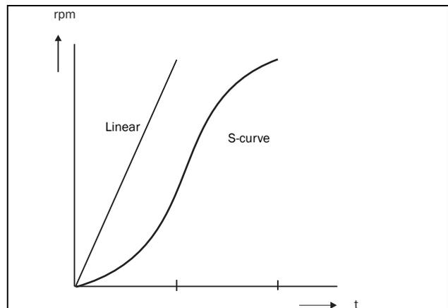
Fig. 63 Shape of acceleration ramp
