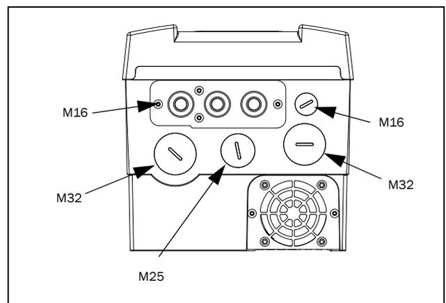
Fig. 7 CDU 48/52: Model 008 to 018 (B) with cable entry/outlets on short side.
