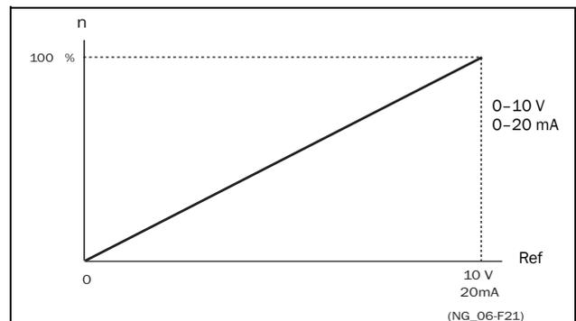
Fig. 88 Normal full-scale configuration
