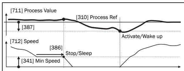
Fig. 74 PID Stop/sleep with normal PID
