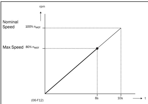
Fig. 60 Acceleration time and maximum speed
