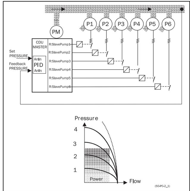
Fig. 31 Pressure control with pump control option
