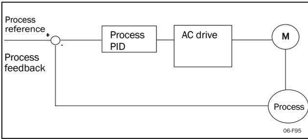
Fig. 73 Closed loop PID control
