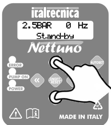
To access these pages switch the device to Stand-by and keep the "+" and "-" keys pressed together for 5 seconds. On entry to the hidden menu, use the "<<<" and ">>>" keys to scroll the pages and the "+" and "-" keys to change the parameters. To return to the main page press the central key.
