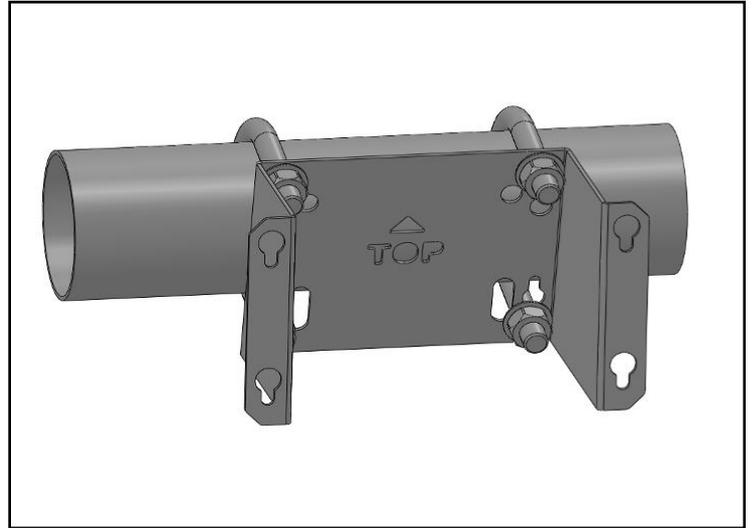
1) Fix the bracket to the pipe by means of the “U-shaped” hooks and 4 bolts supplied. See fig. 6 for selection of the holes.
