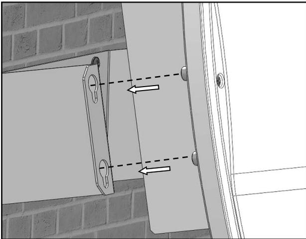
3) Fit *Nettuno* onto the bracket, passing the screw heads on the larger holes and then slide downwards.
