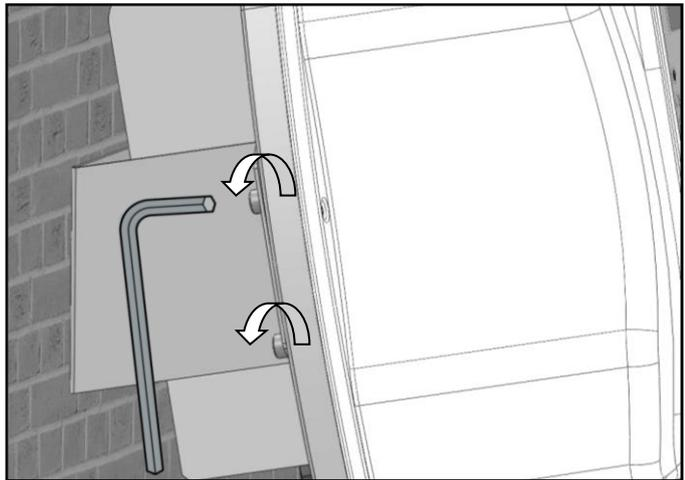
4) Tighten the rear screws fully down on *Nettuno*.
