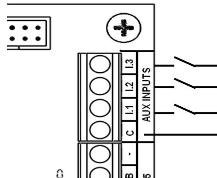
The three digital inputs can all be configured via the software as NO or NC; if the input is set to OFF their functioning is completely ignored.
