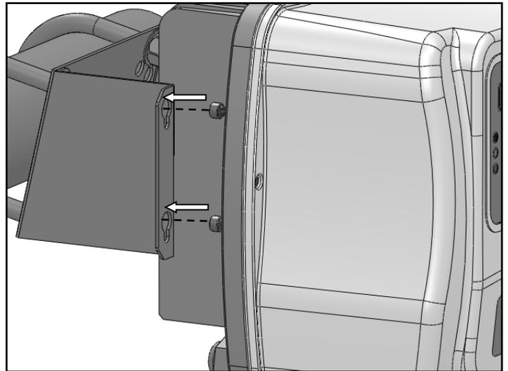
4) Insert Nettuno onto the bracket, passing the screw heads on the larger holes and then slide downwards.
