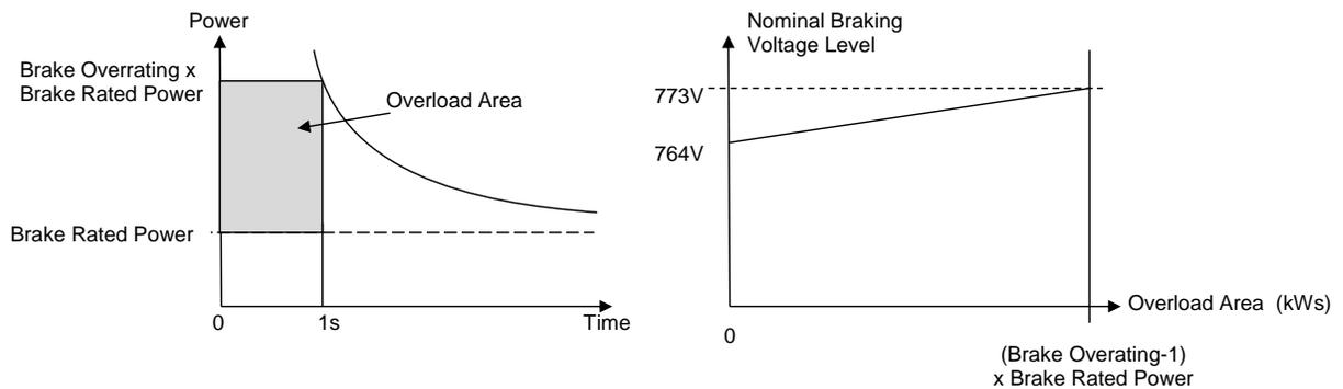
The **Braking** feature also provides a control signal that is used by the **Slew Rate** limit feature. This causes the setpoint to be temporarily frozen whenever the brake is operating because the dc link voltage exceeds the internal comparison level. This allows the stop rate to be automatically tuned to the characteristics of the load, motor, Drive and brake resistor.
