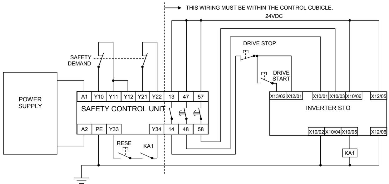
**Note:** On power-up, the Safety Control Unit outputs are OPEN; thus STO is requested of the inverter. This responds by energising KA1 if both channels are active and healthy. KA1 is used as a self-check for the reset cycle of the Safety Control Unit. If a reset cannot be achieved due to KA1 being de-energised, a fault may be present and must be resolved by the user before relying on the STO function. See Fault Operation on page 6-14.
