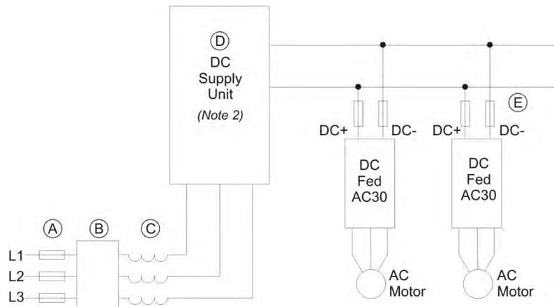
A – Semiconductor fuses, rated to protect the dc supply unit and dc bus installation at maximum power.
