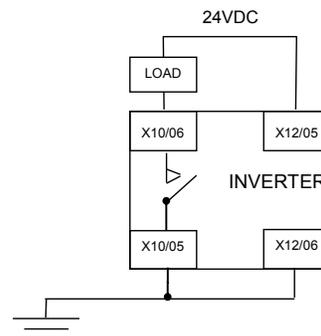
The load is energised and X10/06 is low when STO is in the intended safe STO state.
