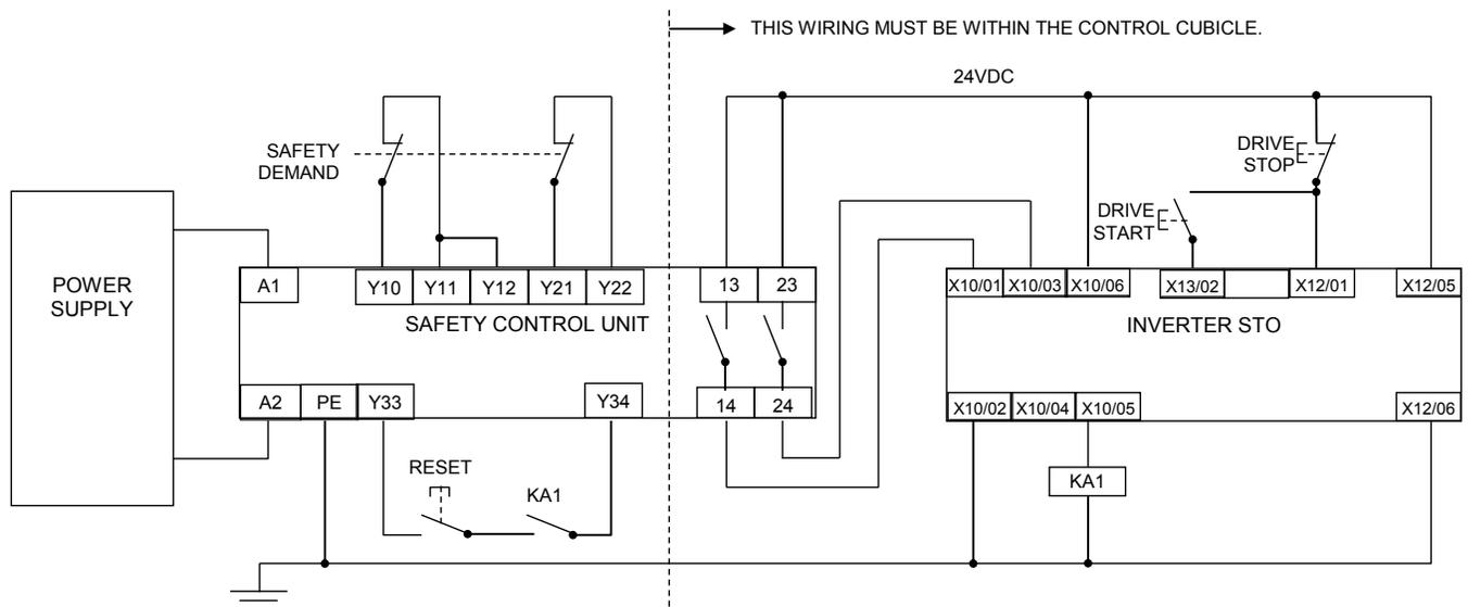
**Note:** On power-up, the safety control unit outputs are OPEN; thus the STO state is requested of the inverter. The latter responds by energising KA1 if both channels are active and healthy. KA1 is used as a self-check for the reset cycle of the safety control unit. If a reset cannot be achieved due to KA1 being de-energised, a fault may be present and must be resolved by the user before relying on the STO function. See Fault Operation on page 6-14.
