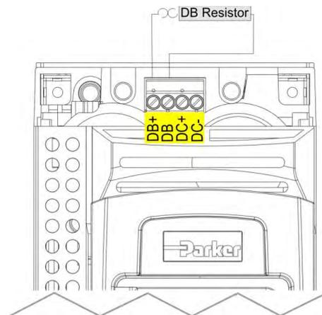
Figure 5.1 External Braking Resistor
