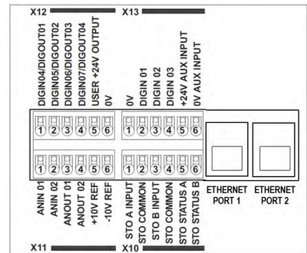
The default macro requires the following electrical wiring diagram for AC30P/AC30D control board. Use of different inputs will need to be accompanied by the appropriate change in the application.
