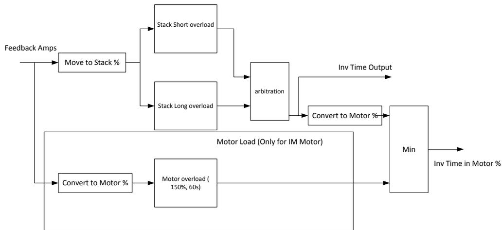
Short Overload : is using 180% of the Heavy Duty rating, for 3s.
