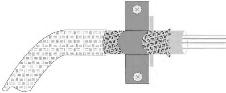
*Figure C-1 360 Degree Screened Connection (Motor)*
