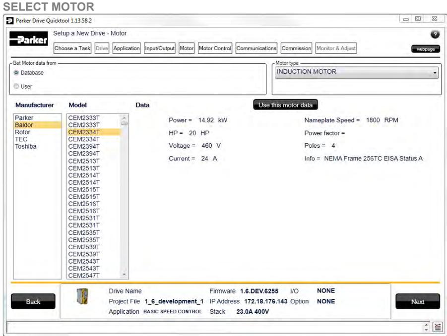
Figure 9-8 Motor selection from database
