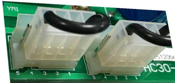
Note: When links are fitted they should be across pins 1 and 4 on the connectors, as shown above.
