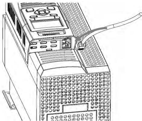
To remove the cable first remove the GKP and then insert a screwdriver to release the catch on the Ethernet clip.
