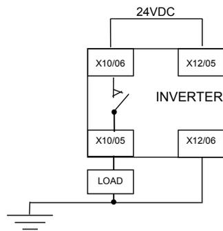
The load is energised and X10/05 is high when STO is in the intended safe STO state.
