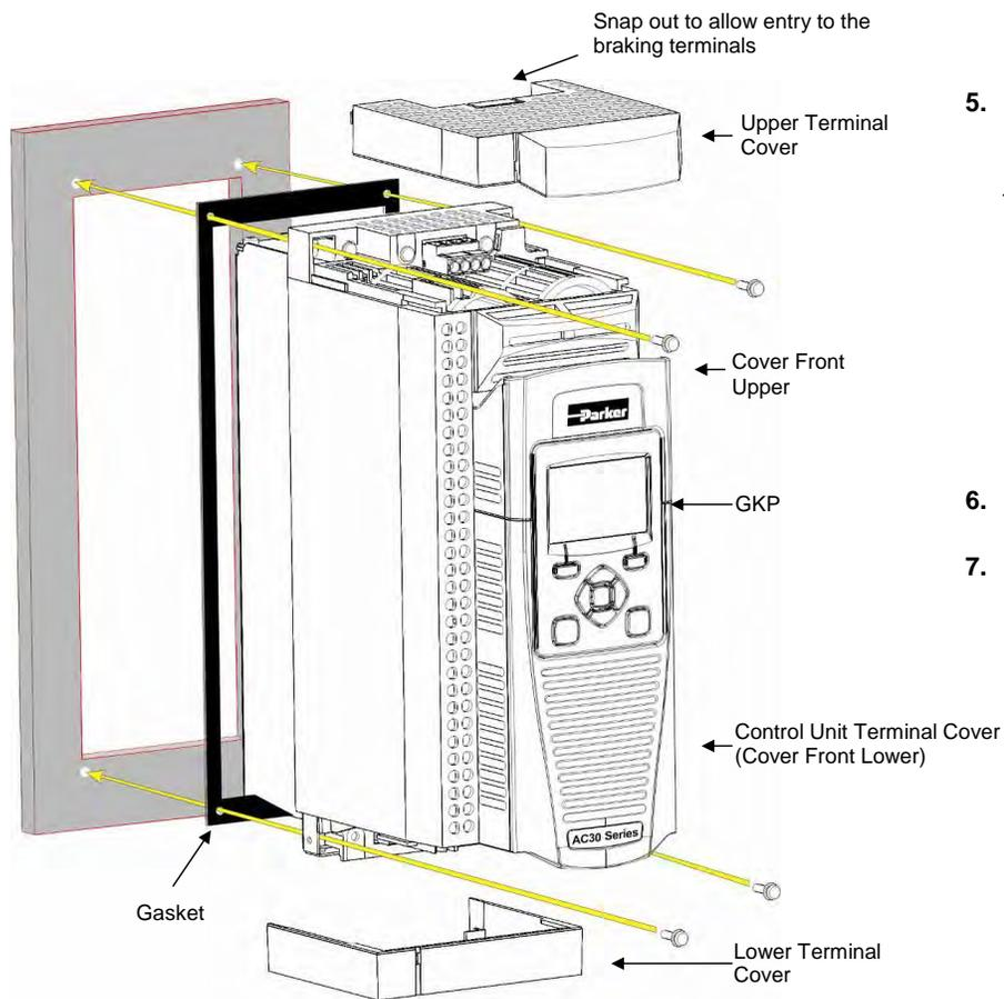
5. Fit gasket to the inverter so that an air-tight seal will be made between the inverter and the panel.
