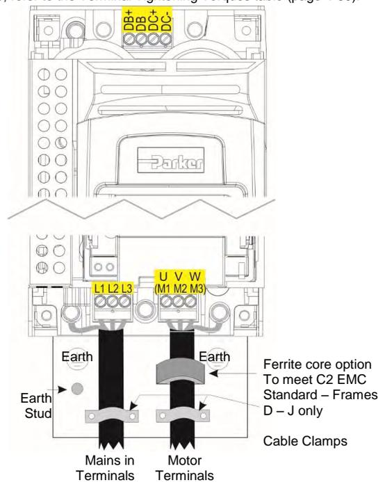
Frame K - no DB+ connect resistor between DC+ & DB)
