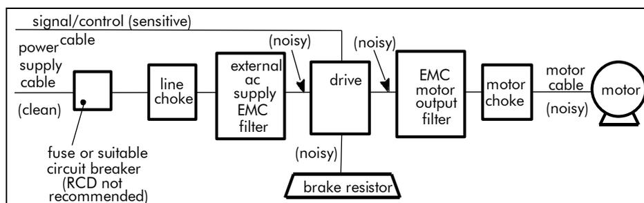
Figure C-2 Cabling Requirements
