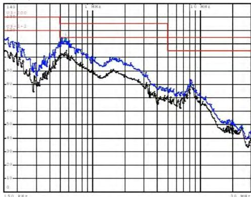
Typical common d.c bus system emissions, for reference (800uH a.c. choke + 890CS supplying 740-4D0012 + 740-4E0023) (Actual system emissions will depend on the details of the specific application.)
