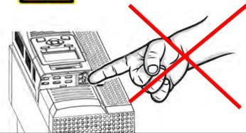
**DO NOT touch the board surface via the aperture shown**
