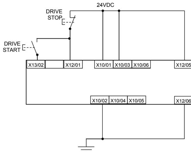
STO inputs X10/01 and X10/03 must be connected to 24VDC with respect to terminals X10/02 or X10/04.
