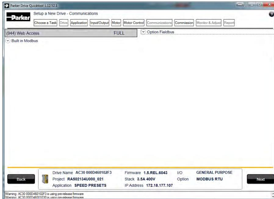
Figure 9-13 Drive Communications setup
