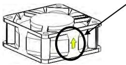
3. Replace the fan guard and tighten the screws to 1.3Nm.
