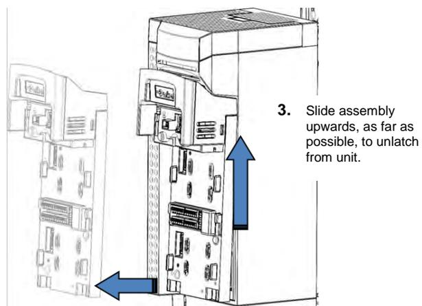
4. Lift assembly away from Power Stack
