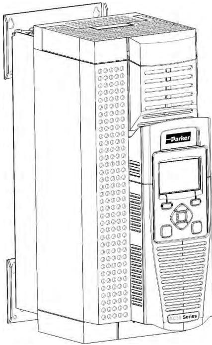
Rear view showing fixing holes for cubicle mount
