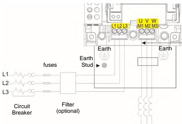
AC Motor Chokes. Only on long cable runs >50m
