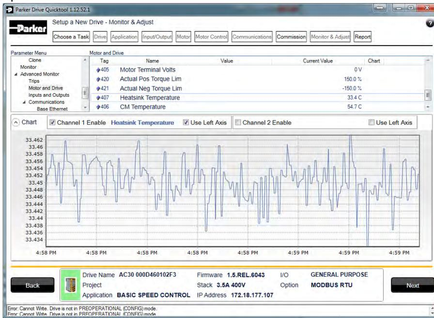
Figure 9-16 Charting Drive Parameters
