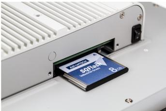
2. ➤ With the label facing up, insert the CFast card until it is completely seated in the slot and reinstall the cover plate.
