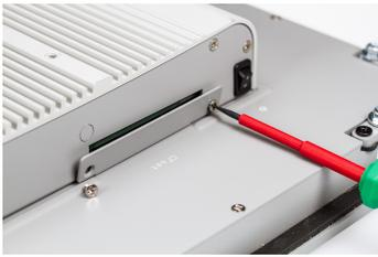
1. Remove the cover plate of the slot by removing the screws and pulling the plate.
