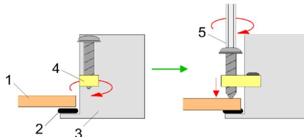
1. ➤ Push the Panel PC [3] from the front side into the front panel cutting [1] until it touches the panel with the seal [2].
