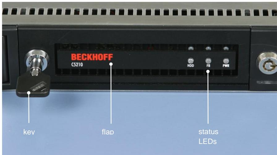
The control elements are located behind a flap at the front side of the Industrial PC. After unlocking the flap with the key it can be folded down. You now have access to the control elements:
