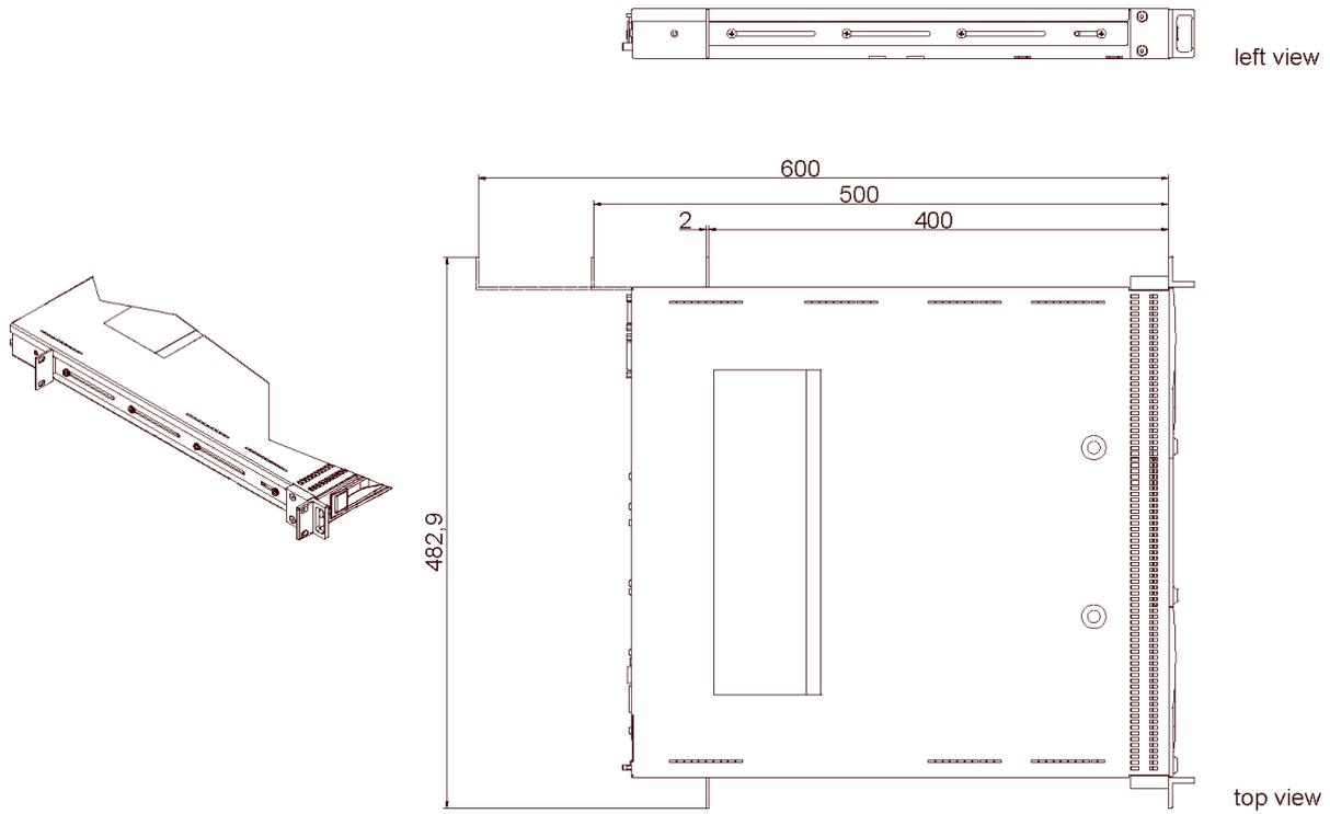
**C5210 with telescope rail Maedler-Accuride 2907**
