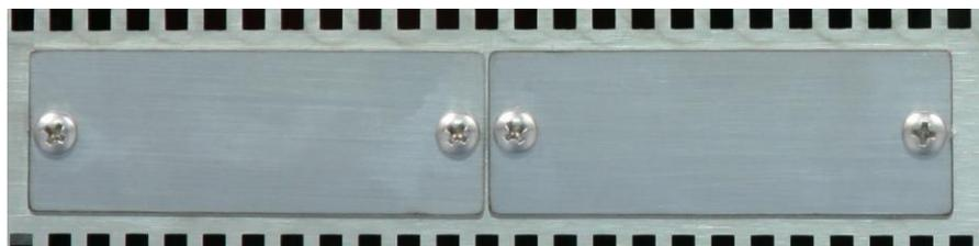
For the installation of the plug in cards first remove the cross-head screws. The cover caps can now be removed and allow plugging in the plug in cards.
