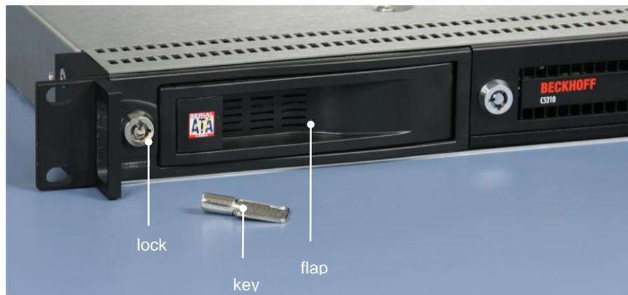
The hard disks are located into two removable hard drive racks at the front of the Industrial PC. After unlocking the flaps of the removable racks you can swivel out the hard disks. Now the disks can be removed.
