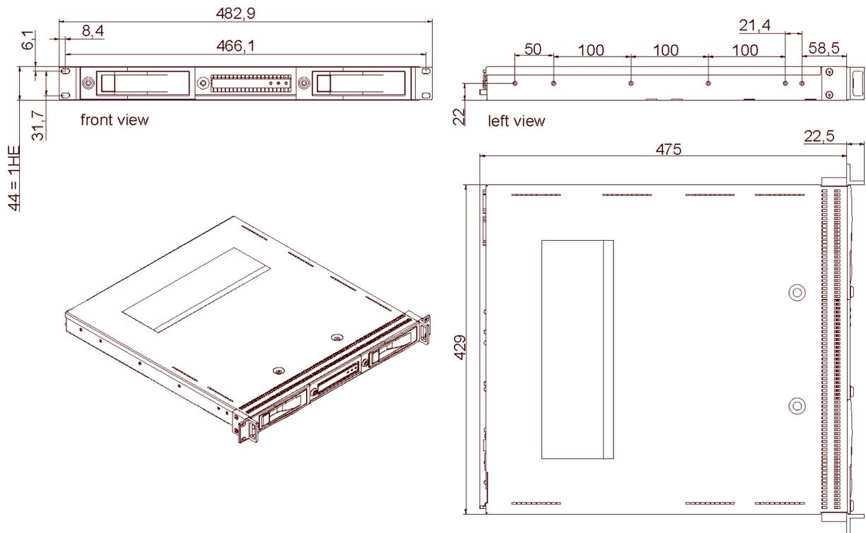
**C5210, view with mounted assembly brackets**
