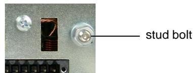
The Industrial PC is grounded via the stud bolt.
