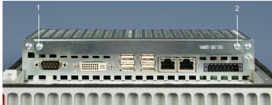
After loosening the two screws (1) and (2) the cover plate can be removed.
