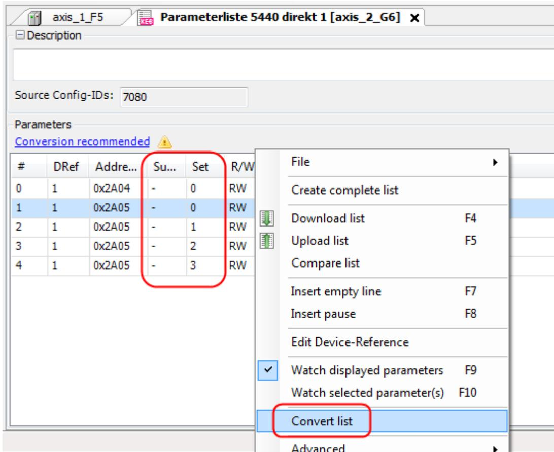
The screenshot shows the 'Parameterliste 5440 direkt 1 [axis\_2\_G6]' window. It features a table of parameters with columns for index, DRef, Address, Sub-index, Set, and R/W. A red circle highlights the 'Su...' and 'Set' columns for rows 1 through 4. A context menu is open over the table, with 'Convert list' highlighted by another red circle.
