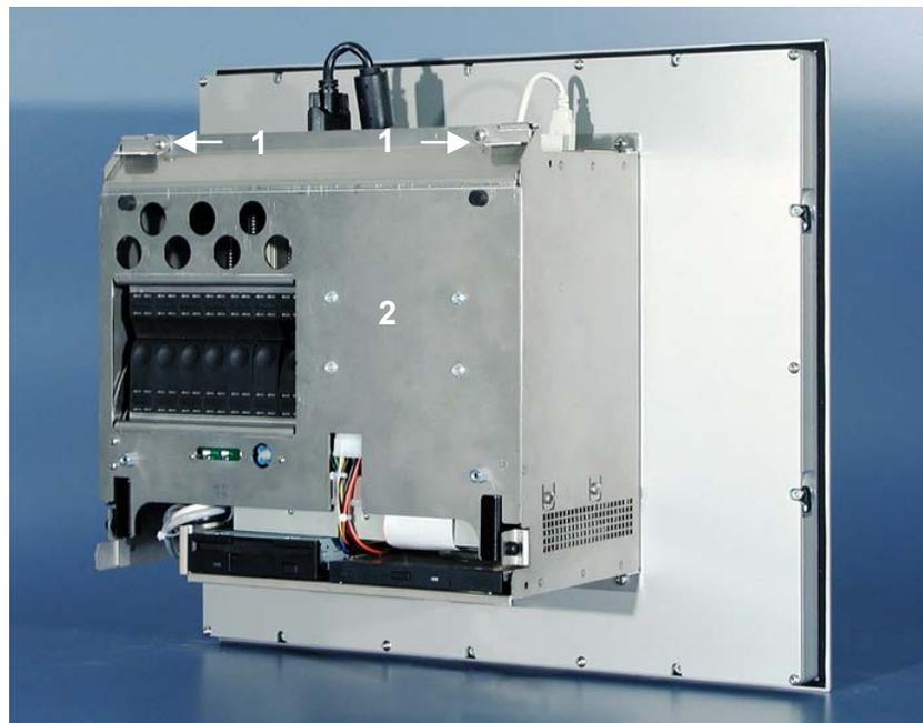
Unfasten the two securing levers (1) that hold the fold-out inner chassis (2).
