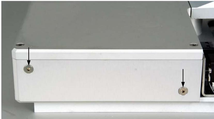
After unscrewing the two Allen screws (see arrows) the drive cover can be taken off.
