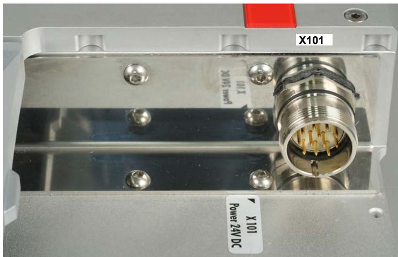
The power supply connection of the Industrial PC and the connection with the UPS (optional) is established via the power supply socket (**X101**).
