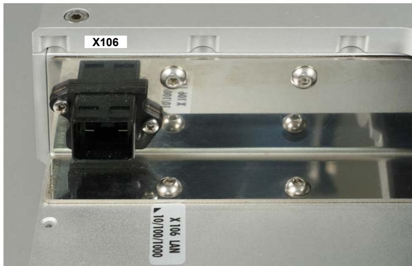
The Ethernet-interface with RJ-45-connector (**X106**) allows the PC to be connected to a network (LAN). In the basic configuration a Gigabit-port is available.
