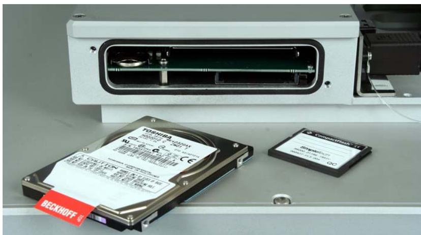
The hard-disk drive and the memory card can now be pulled out. Here, changing the lithium battery is also possible.
