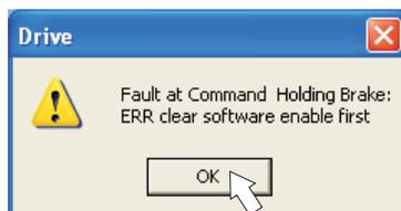
If Software Enable is active, a warning appears. You can proceed, but after the amplifier is restarted, you must check whether the holding brake configuration is correct. Click OK.
