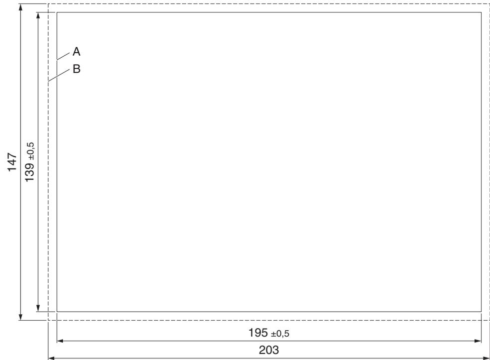
Figure 2-8 Mounting cutout (dimensions in mm)
