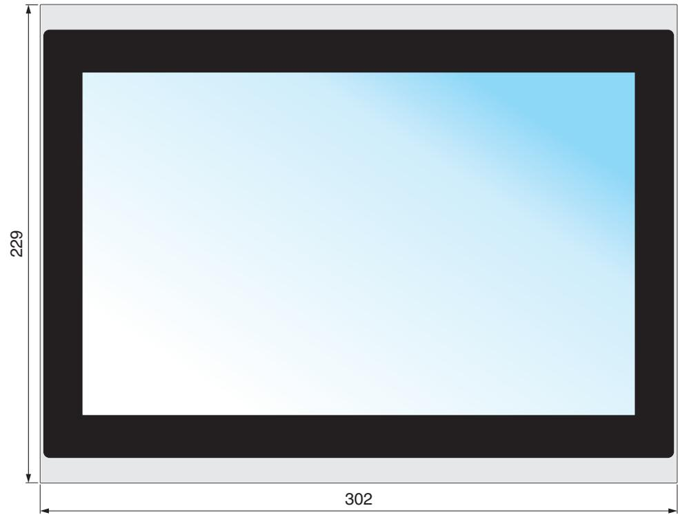
Figure 2-5 Front panel (dimensions in mm)
