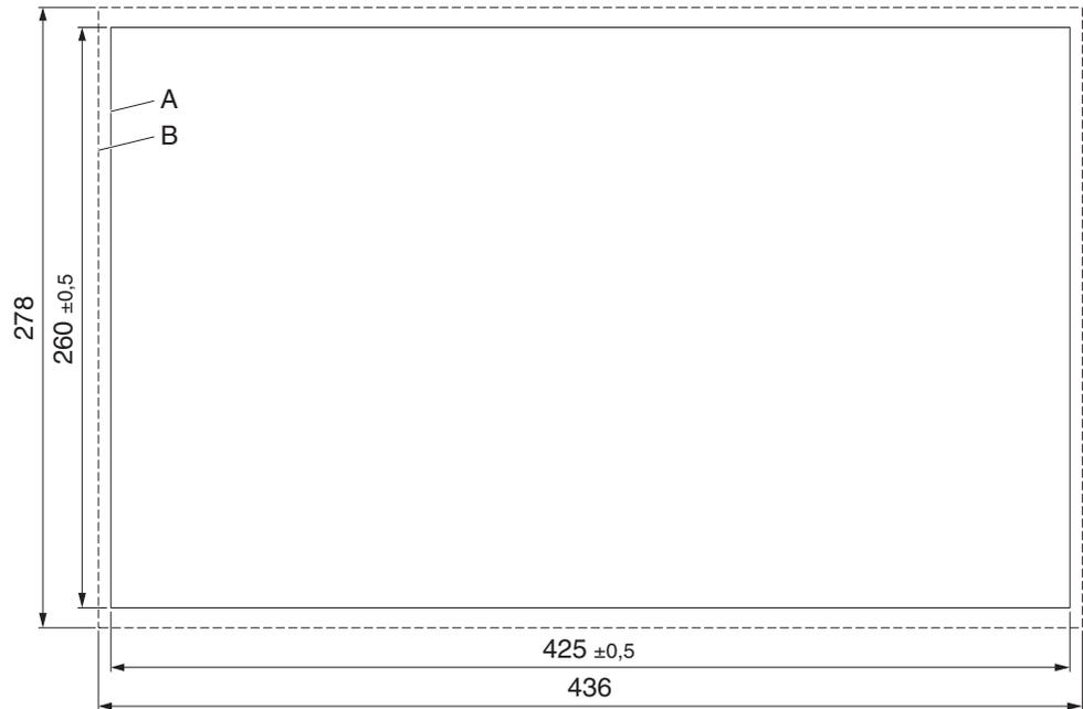
Figure 2-12 Mounting cutout (dimensions in mm)
