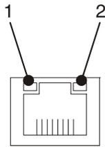
Figure 4-2 Position of the ethernet diagnostics LEDs
