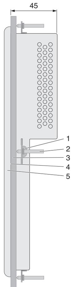
Figure 2-17 Side view, mounting depth (dimensions in mm)
