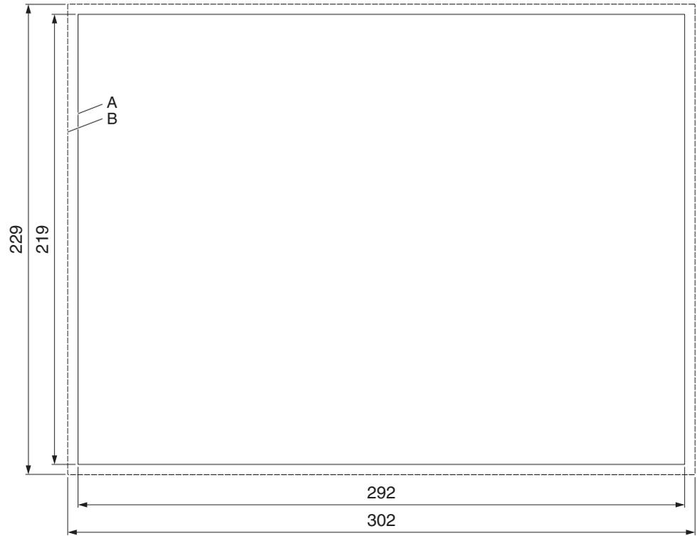
Figure 2-11 Mounting cutout (dimensions in mm)
