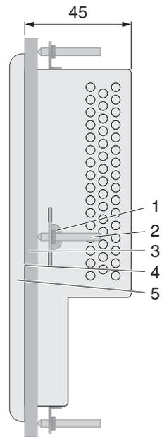
Figure 2-15 Side view, mounting depth (dimensions in mm)
