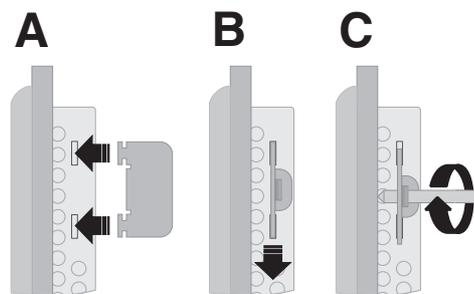
Figure 2-1 Mounting the device using a mounting bracket
