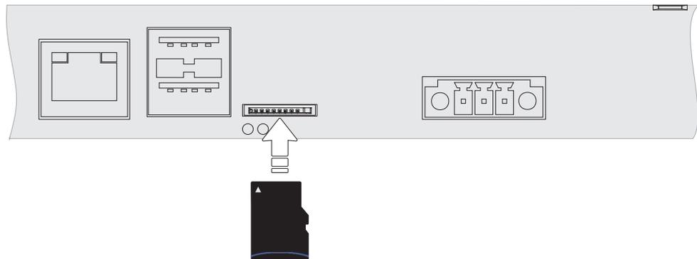
Figure 4-3 Inserting the memory card
