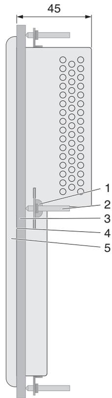
Figure 2-16 Side view, mounting depth (dimensions in mm)
