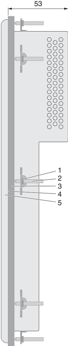
Figure 2-18 Side view, mounting depth (dimensions in mm)
