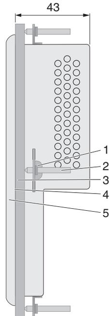
Figure 2-14 Side view, mounting depth (dimensions in mm)
