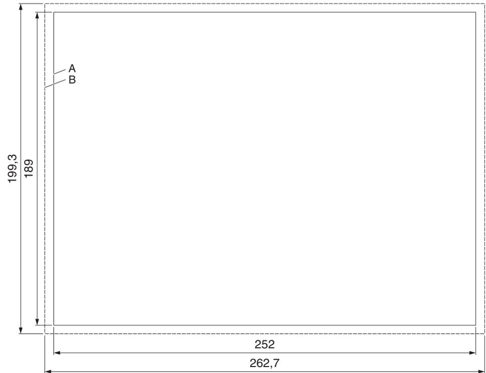
Figure 2-10 Mounting cutout (dimensions in mm)
