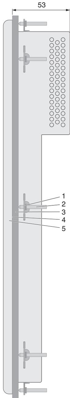
Figure 2-19 Side view, mounting depth (dimensions in mm)
