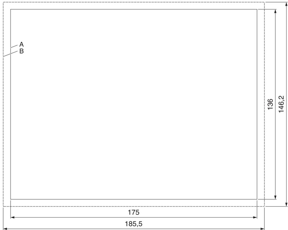
Figure 2-9 Mounting cutout (dimensions in mm)
