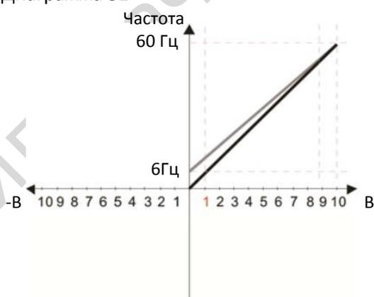
$$\text{Сдвиг } 03-03: = \frac{60-6\text{Гц}}{10\text{В}} = \frac{6-0\text{Гц}}{(0-x\text{В})}; x\text{В} = \frac{10}{-9} = -1.11\text{В}$$
